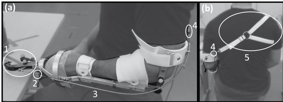
Figure 3–1. Side-view (a) and back-view (b) of one subject wearing the custom-made bypass-prosthesis. The prehensor (1) is connected to the fitting. The prehensor (1) was connected via a Bowden cable (3) to the “figure-of-nine” harness (5). The Bowden cable forces were measured before and after the outer cable housing with force sensor 1 (2) and force sensor 2 (4).
