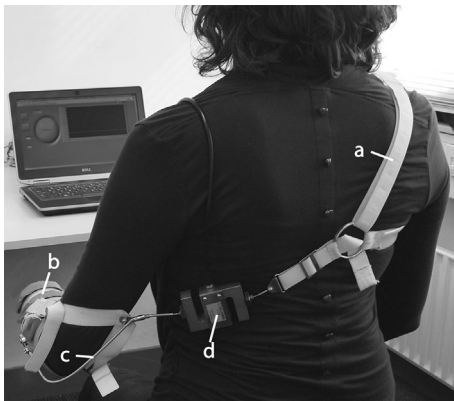
Figure 4–2. Measurement set-up for maximum force measurements: the “figure-of-nine” harness (a) and thermoplastic shell (b) are connected through a Bowden cable (c), which is interrupted by a force sensor (d). In this set-up cable excursions are disabled.
