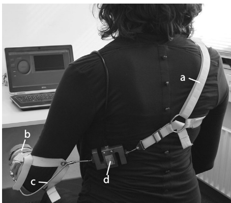
Figure 2–1. Measurement set-up for maximum force measurements: the “figure-of-nine” harness (a) and thermoplastic shell (b) are connected through a Bowden cable (c), which is interrupted by a force sensor (d). In this set-up cable excursions are disabled.
