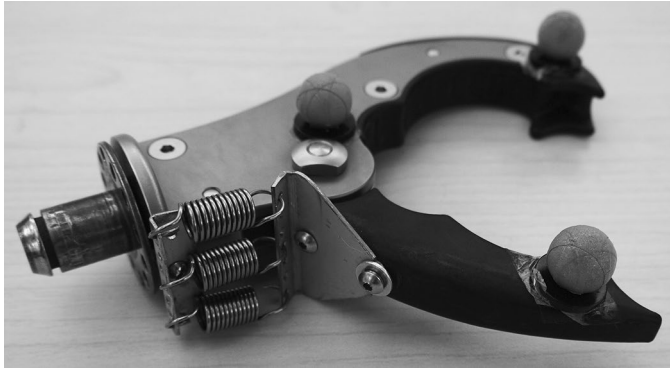
Figure 3–2. TRS hook with the internal torsion spring replaced by external linear springs in the high force setting (3 x 1.7 N/mm springs); 2 x 0.11 N/mm springs were used for the low force setting.
