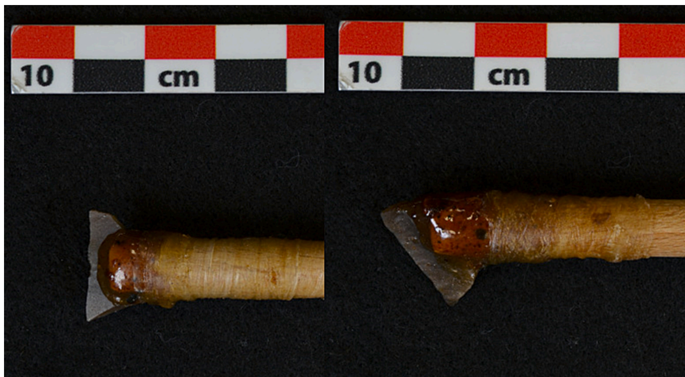
Fig. 1. Photos of experimental arrows A and C used in the experiments showing the transversal and diagonal hafting configurations.
