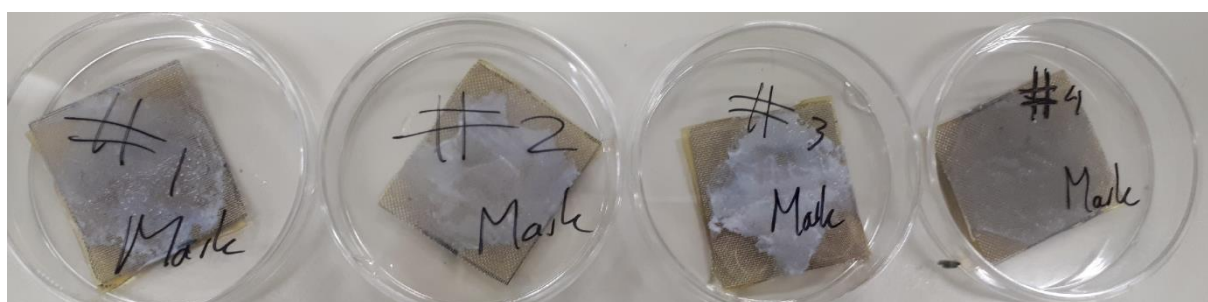
Figure 40. Visual whitening of the ionomer solution after immersion in water. Sample #4, which has the lowest ionomer loading, shows the smallest visual alteration.
