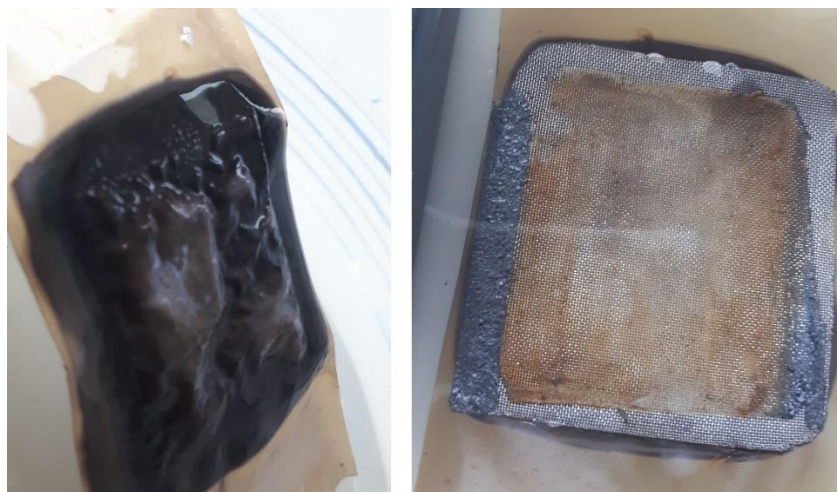
Figure 46 The ionomer BPMEA configuration after 1 day in water. On the left the partially delaminated bipolar membrane turned black at the interface region. On the right a brownish colour appeared where the ionomer was applied, the taped off edges do not show this colour change.
