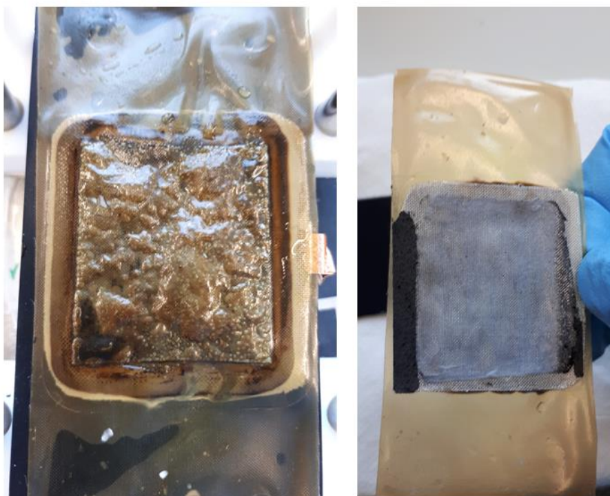
Figure 45 The ionomer BPMEA configuration after 1 h chronoamperometry. Extreme bubble formation on the anode side of the membrane is found, while the cathode side only shows no irregularities, aside of some carbon paper stuck to the Ag-mesh.
