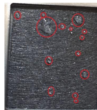
Figure 24 Electrolyte seeping through the GDL towards the gas phase. Red circles indicate visible droplets.
