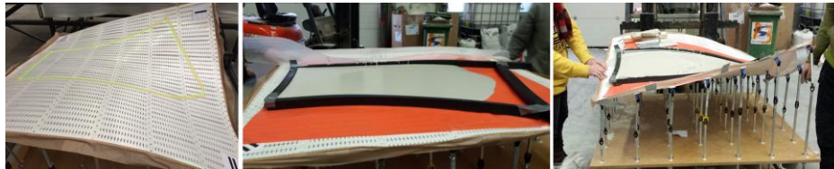
Fig. 1. Flexible mould system before and after deformation [1].
