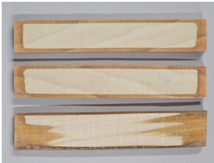
Figure A.14 Cross-sections of the three yellow poplar blanks after processing. The dark peripheral border surrounding the lighter core was confirmed to be a surface colouration effect rather than a density gradient. Densification is uniform.
