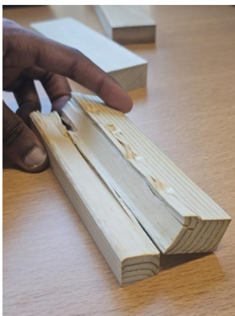
Figure C.5. A Norway spruce specimen at 50% compression after indentation, showing catastrophic brittle fracture in which the coupon split along its full length into separate halves.
