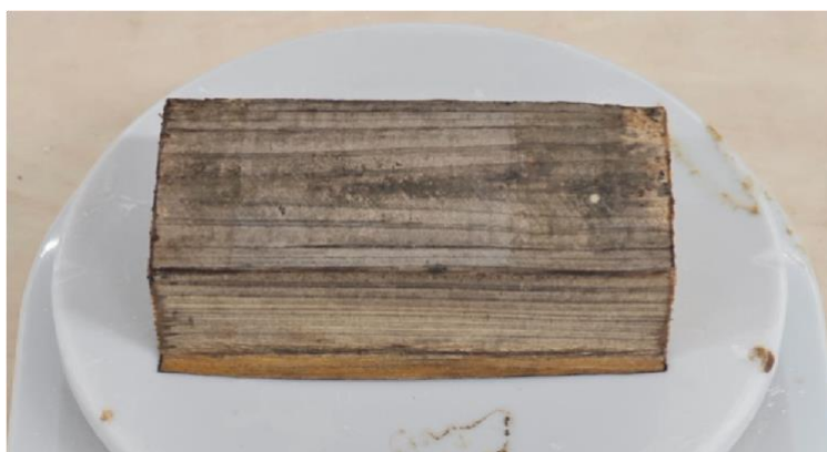
Figure A.12 Sample 3 After Pressing - Clean Surface, No Cracking, No Springback
