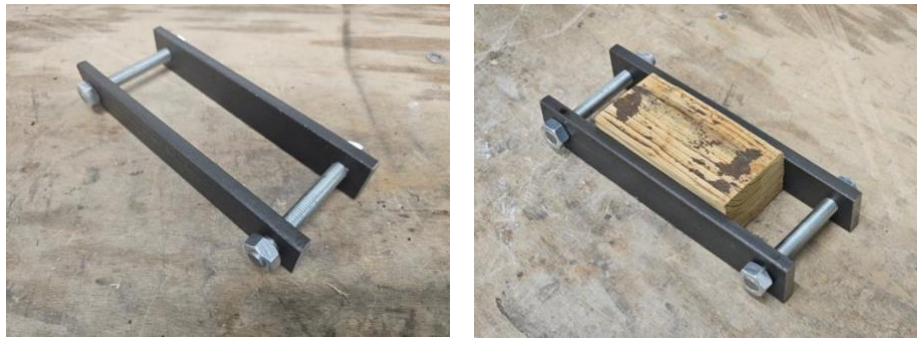
Figure A.10 Steel Jig to Constrain the Sample During Pressing
