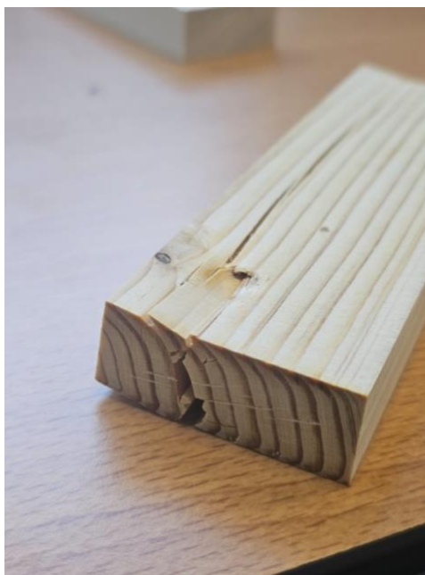
Figure C.4. A Norway spruce specimen at 25% compression after indentation, showing a longitudinal split propagating from the indented surface along the grain instead of a plastic indentation.
