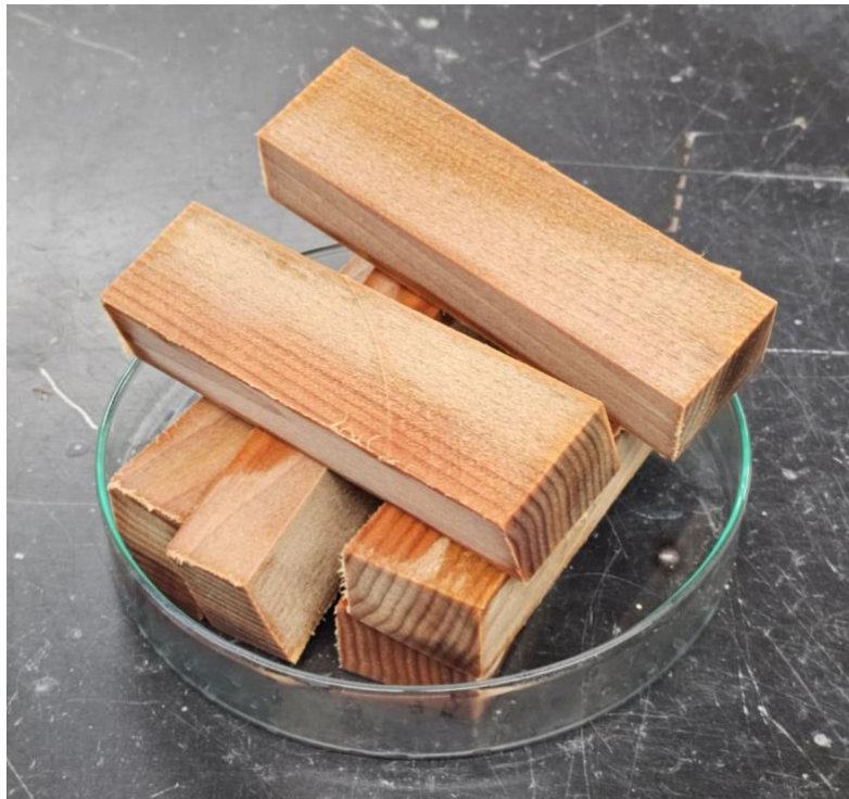
Figure A.13 Yellow poplar blanks after boiling, showing the characteristic dark amber colouration of the solution and the darkened sample surfaces.
