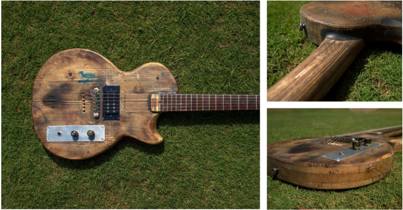
Scratch Paul, the author's reclaimed-wood electric: a body laminated from pine drawing-board offcuts and a laterally laminated marine plywood neck.[1]
