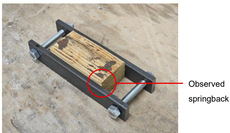
Figure A.11 Sample 2 After Cold Pressing, Showing Springback Upon Release from Jig
