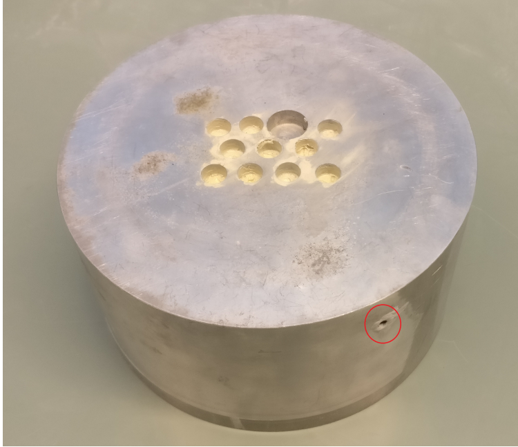
Figure 29: Aluminum block as thermal low pass filter
