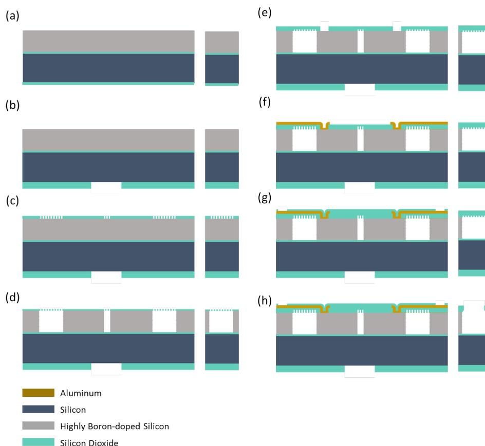
Figure 4.7: Process flow of the Electrode Integrated Embedded Microchannel (EIEMC)
