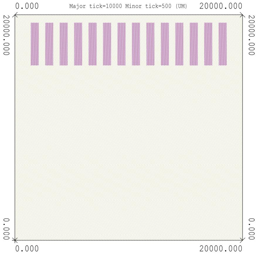
Figure A.3: Mask design of the bondpad
