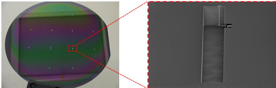
Figure 4.6: Backside window after DRIE. (a) Wafer level view (b) Zoomed view of the area shown in the box. The inner area of the rectangle was discolored and transparent.
