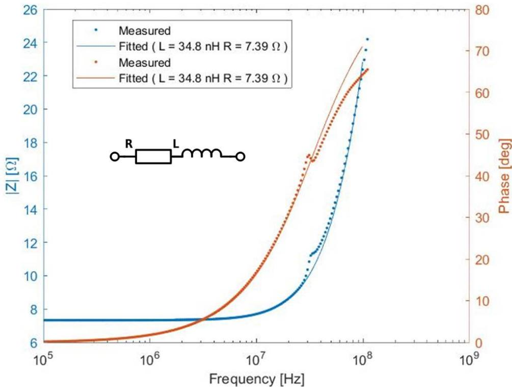
Figure 5.3: Impedance spectroscopy result of the ground connection.
