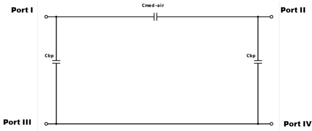
Figure 5.5: Equivalent circuit model with only air inside the channel
