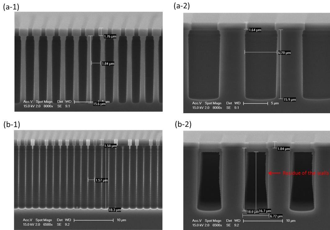
Figure 3.5: 4.5 min of etching with single step DRIE with the spacing between etch hole as (a) 1.8 μm and (b) 0.8 μm.
