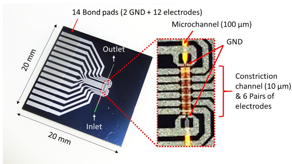
Figure 4.8: Fabricated device (Left). Close up image of the device (Right)
