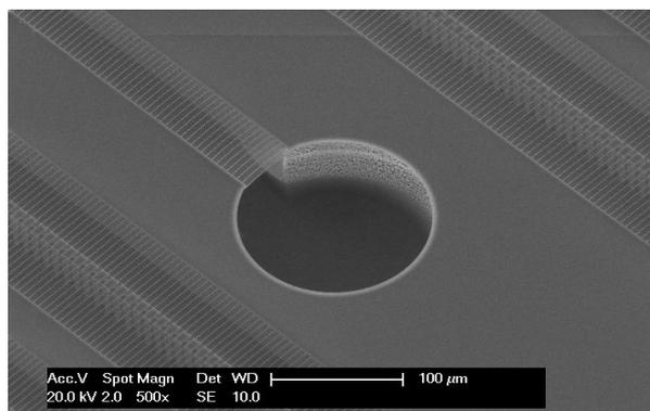
Figure 4.2: Inlet/Outlet opened with method 1; simultaneously etching the inlet/outlet along with the EMC.
