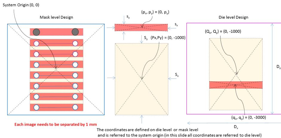
Figure B.2: Design guide for multi-level exposure
