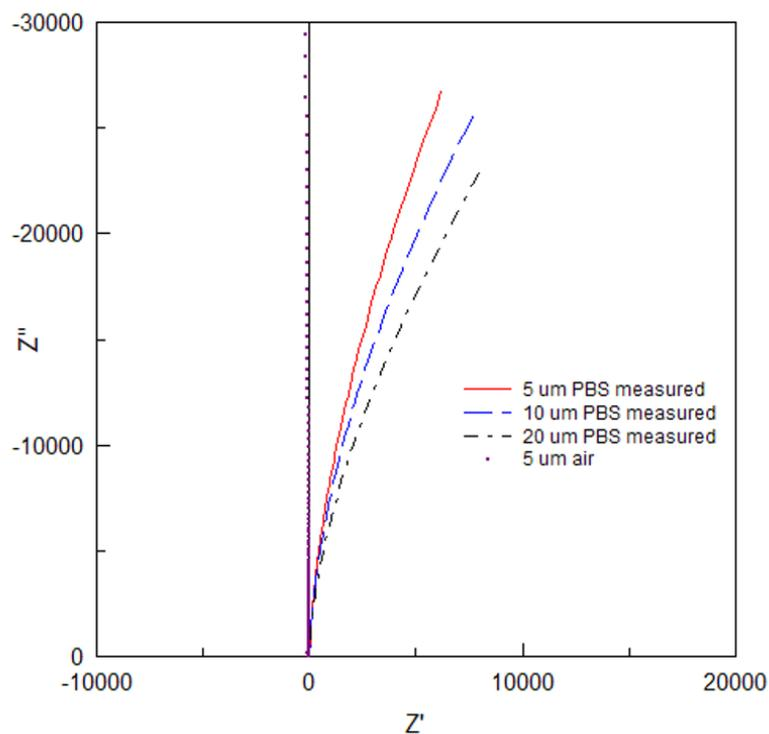
Figure 5.7: Measured real and imaginary impedance when PBS is inside the channel. For comparison, the impedance when air was inside the channel is also shown in the figure. The figure shows the measured result for 5  $\mu\text{m}$ (10 and 12), 10  $\mu\text{m}$ (9 and 13) and 20  $\mu\text{m}$ (8 and 14). The numbers in parenthesis are the electrodes used for the measurement.
