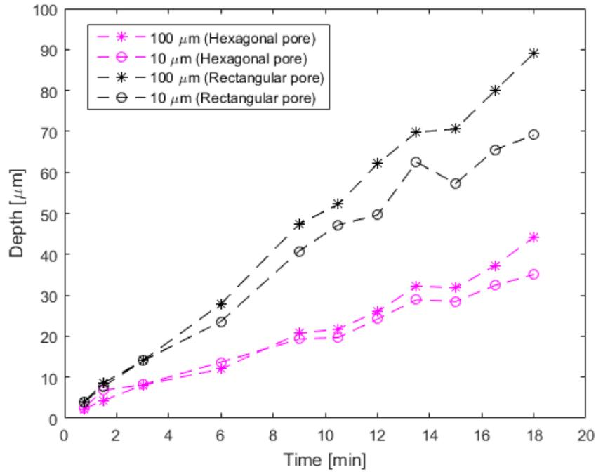
Figure 3.9: The EMC depth against total etch time for different width and design of the mesh hard mask
