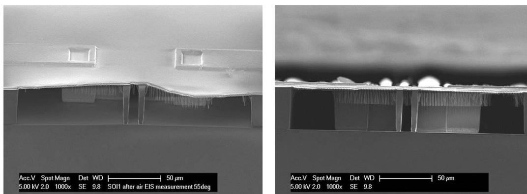
Figure 4.11: A SEM image of the cross section of the channel seen from an 55degree angle (Left) and the cross section seen from a 90 degree angle (Right). The icicle length was 14  $\mu\text{m}$ .
