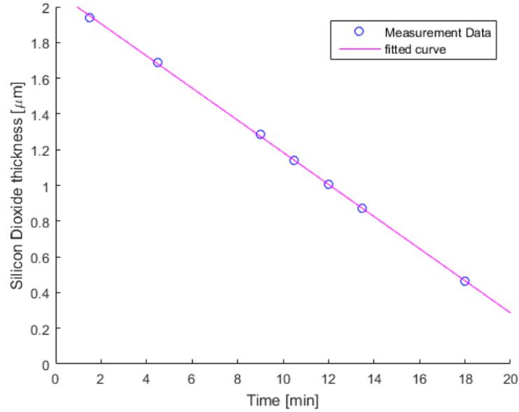
Figure 3.7: The decrease in the thickness of SiO<sub>2</sub> hard mask during the single step DRIE
