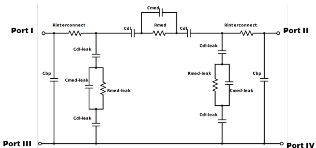
Figure 5.2: Equivalent circuit model with PBS inside the channel equivalent to the model that was presented in 2. For the values of the component refer to 2.
