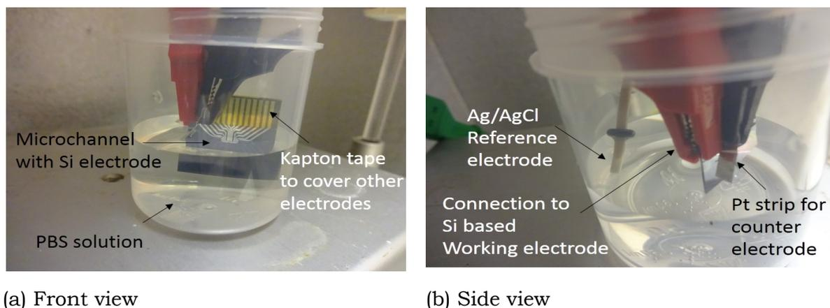
Figure 5.14: Cyclic voltammetry experiment setup.
