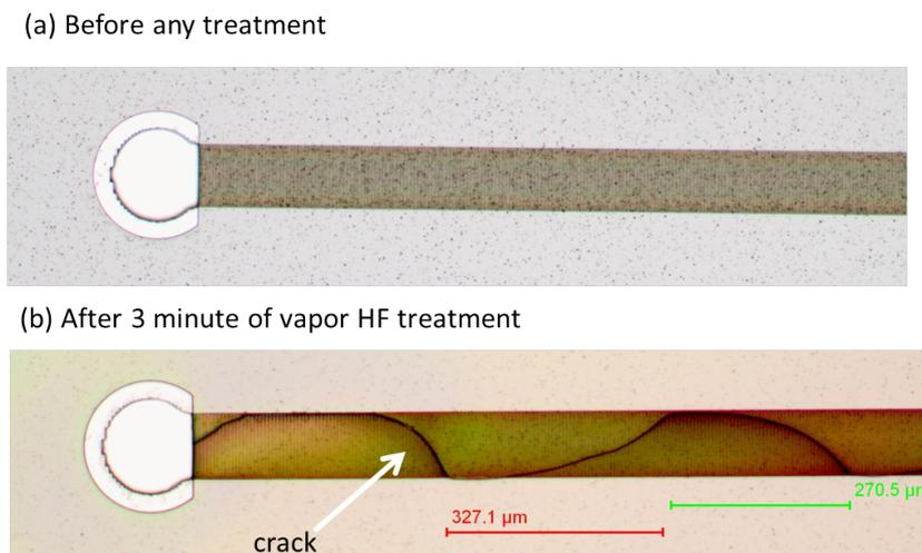
Figure 4.15: An image of the channel from above using a optical microscope before and after 3 min of vapor HF treatment.
