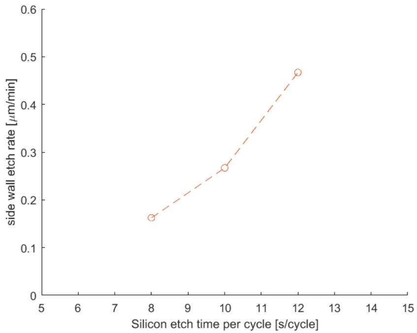
Figure 3.12: The side wall etch rate against the silicon etch rate per cycle
