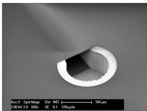
Figure 4.12: SEM image of the inlet/outlet after it was opened with dry etch. More stress is induced because there are many corners.
