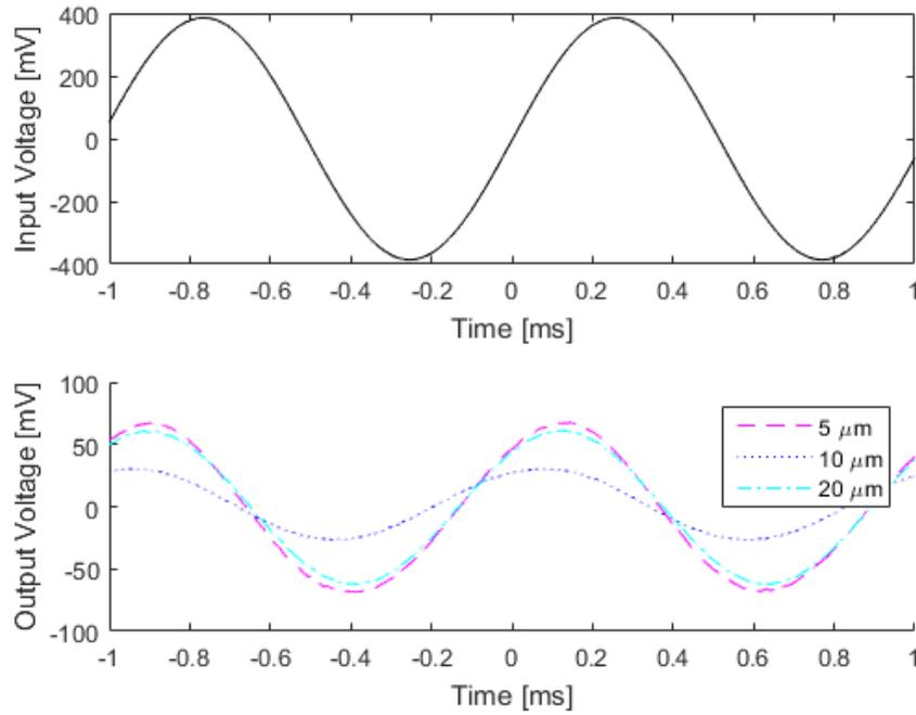
Figure 5.10: Input voltage (above) and the output voltage for different electrode width (bottom) when PBS solution was continuously injected through the channel.
