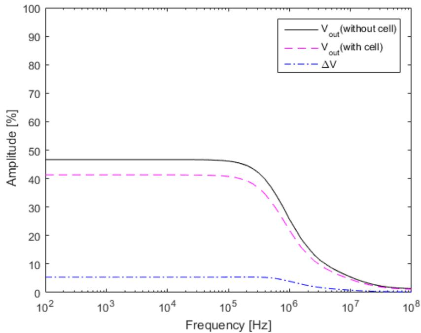
Figure 2.11: AC simulation result from 100 Hz to 100 MHz. The output voltage is plotted for two situation with and without the cell.  $\Delta V = V_{out}(\text{without cell}) - V_{out}(\text{with cell})$  is the difference between the amplitude.
