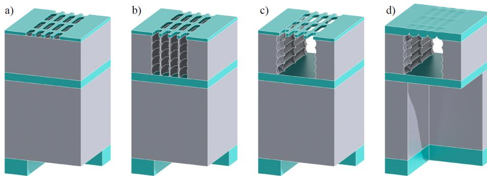
Figure 3.1: Process steps for the fabrication of embedded microchannels. a) Small holes are etched into a 500 nm  $\text{SiO}_2$  layer. b) The silicon is deep reactive ion etched anisotropically until the BOX layer. c) The remaining silicon is removed from the channels with a  $\text{CF}_4$  etch isotropically. d) The holes are closed with a 2.0  $\mu\text{m}$  TEOS and the observation port is deep reactive ion etched from the back. *Source: reprinted from R.Stoute et al. [12].*
