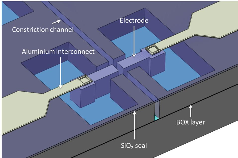
Figure 2.3: 3D model of the Electrode Intergrated Embedded Microchannel.
