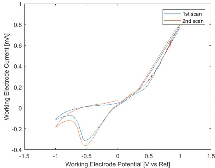
Figure 5.15: Cyclic voltammetry result for silicon electrode using a Ag/AgCl reference electrode and Pt counter electrode.
