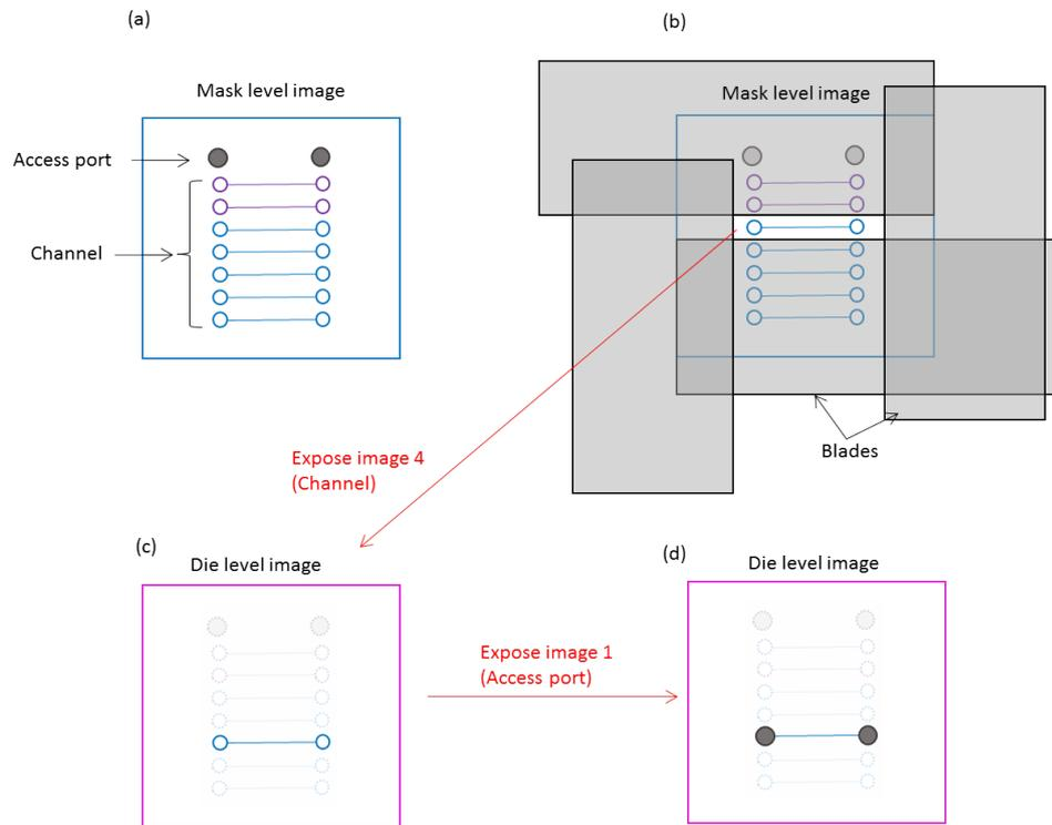
Figure B.1: Multilevel exposure method 1
