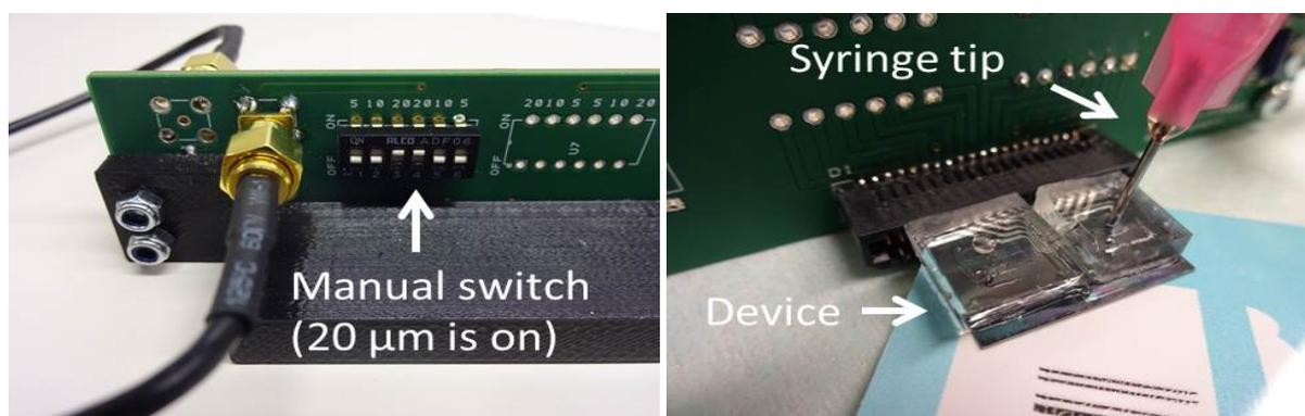
(a) Manual switch on the backside of the (b) Device inside the edge card slot with the PCB. Electrodes  $20\ \mu\text{m}$  wide are on in this microfluidic pump connected to the device via the syringe tip and the PDMS seal.
