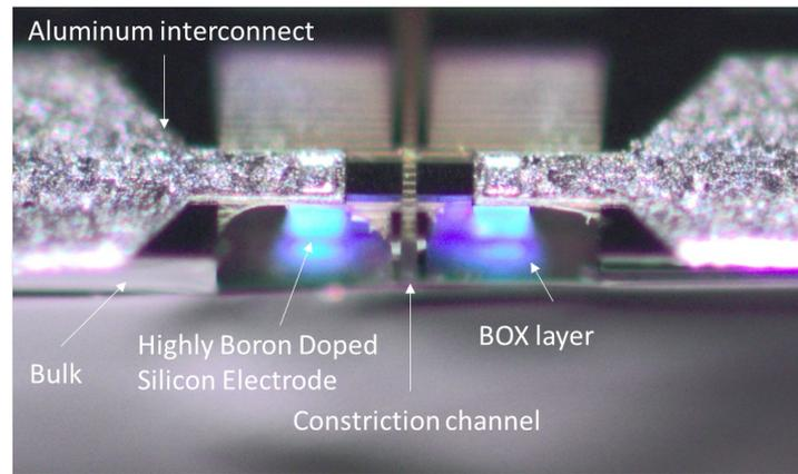
Figure 4.9: An optical microcope image of the cross section of the electrode and the constriction channel.
