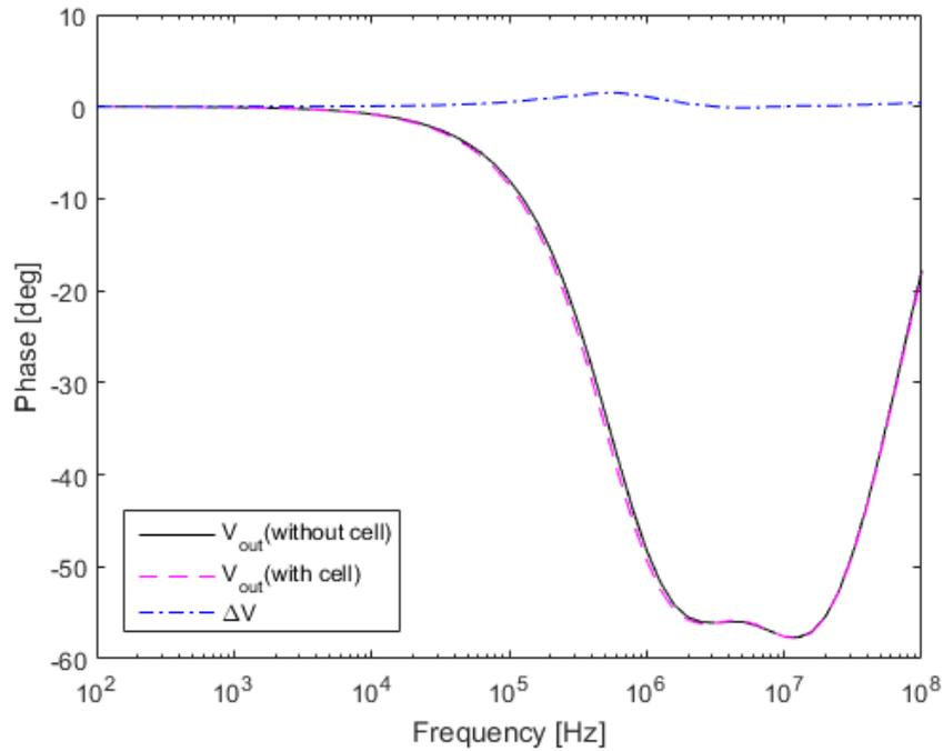
Figure 2.10: AC simulation result from 100 Hz to 100 MHz. The phase of the output voltage is plotted for two situation with and without the cell.  $\Delta V = V_{out}(\text{without cell}) - V_{out}(\text{with cell})$  is the difference between the phase.
