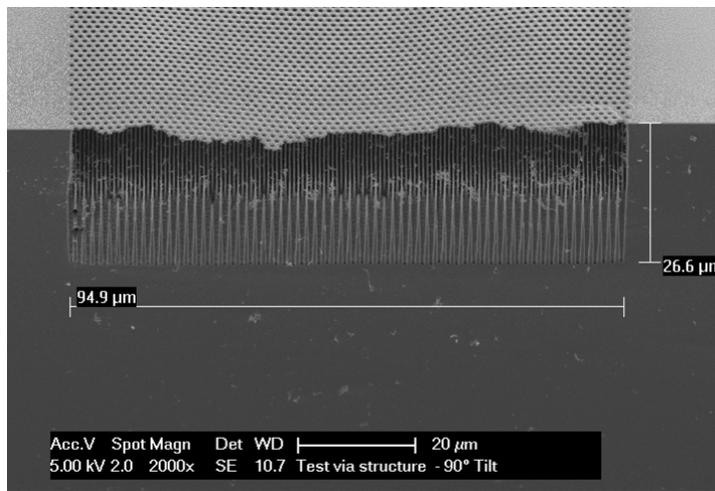
Figure 3.14: 2 min of isotropic etch followed by a DRIE with a lower substrate bias.
