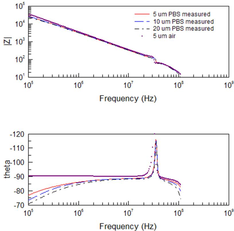
Figure 5.6: Measured modulus and phase of the impedance when PBS is inside the channel. For comparison, the impedance when air was inside the channel is also shown in the figure. The figure shows the measured result for 5  $\mu\text{m}$ (10 and 12), 10  $\mu\text{m}$ (9 and 13) and 20  $\mu\text{m}$ (8 and 14). The numbers in parenthesis are the electrodes used for the measurement.
