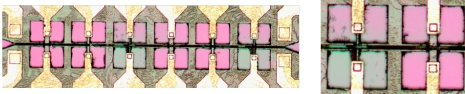
Figure 5.13: 3 min of vapor HF treatment followed by a kapton tape attached to the mesh and removed along with the  $\text{SiO}_2$  membrane. (There is also a 3 min vapor HF performed beforehand so in total it will be 6 min of vapor HF)
