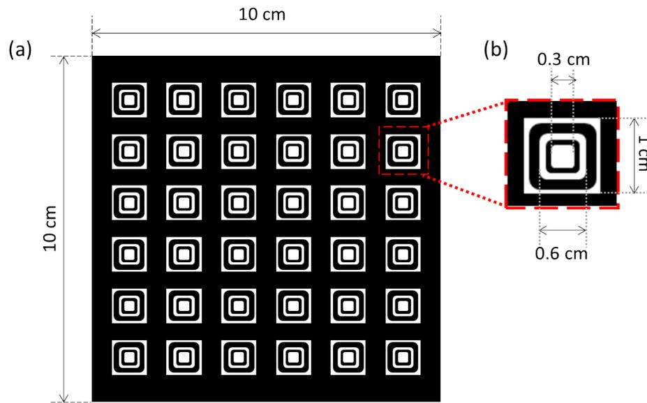
Figure C.1: the printable mask design used for the PDMS seal
