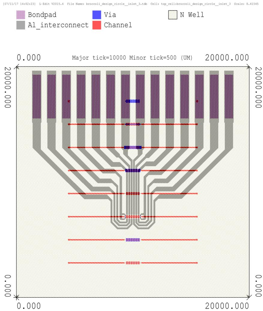
Figure A.1: Mask design with all layers
