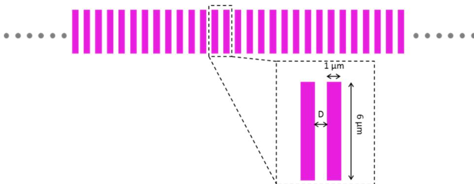
Figure 3.3: The mask design used for evaluating the influence of the distance between neighboring holes to the etch rate. The exposed region is the colored rectangular area. On the same mask spacing between the holes (D) was varied from 0.6 μm to 2.0 μm with a step of 0.2 μm.
