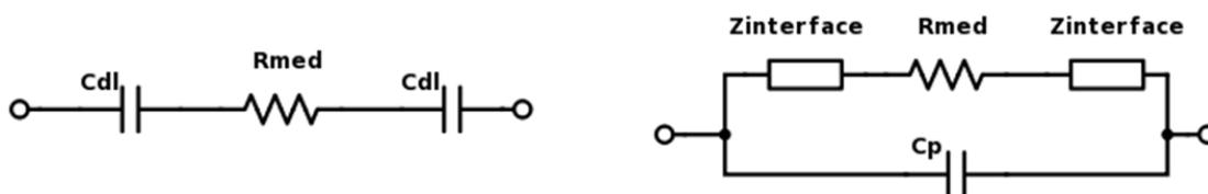
(a) Equivalent circuit model of the channel with the interface impedance modeled as only a double layer capacitance.
