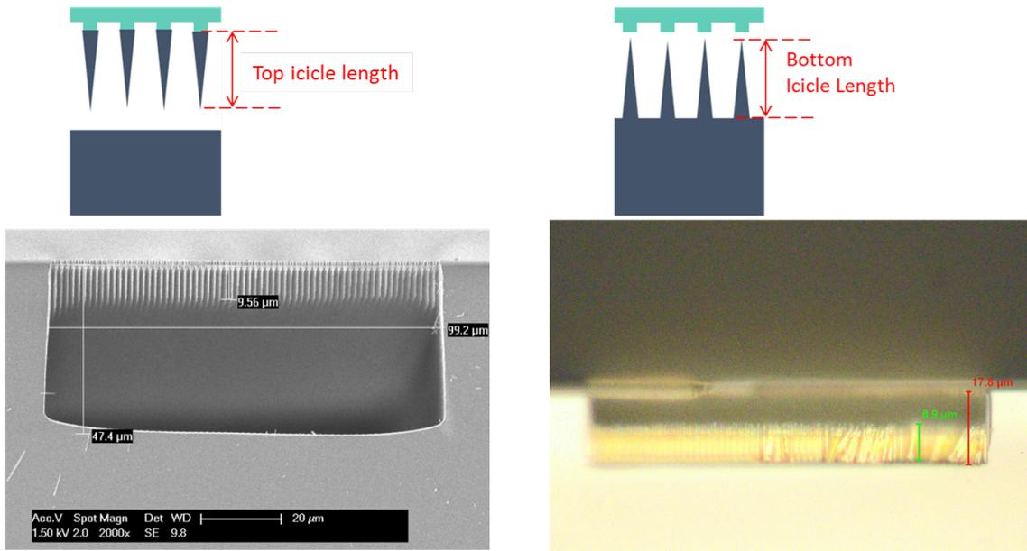
(a) Top icicles that formed when rectangular pores were used for the mesh hard mask. (b) Bottom icicles that formed when hexagonal pores were used for the mesh hard mask.
