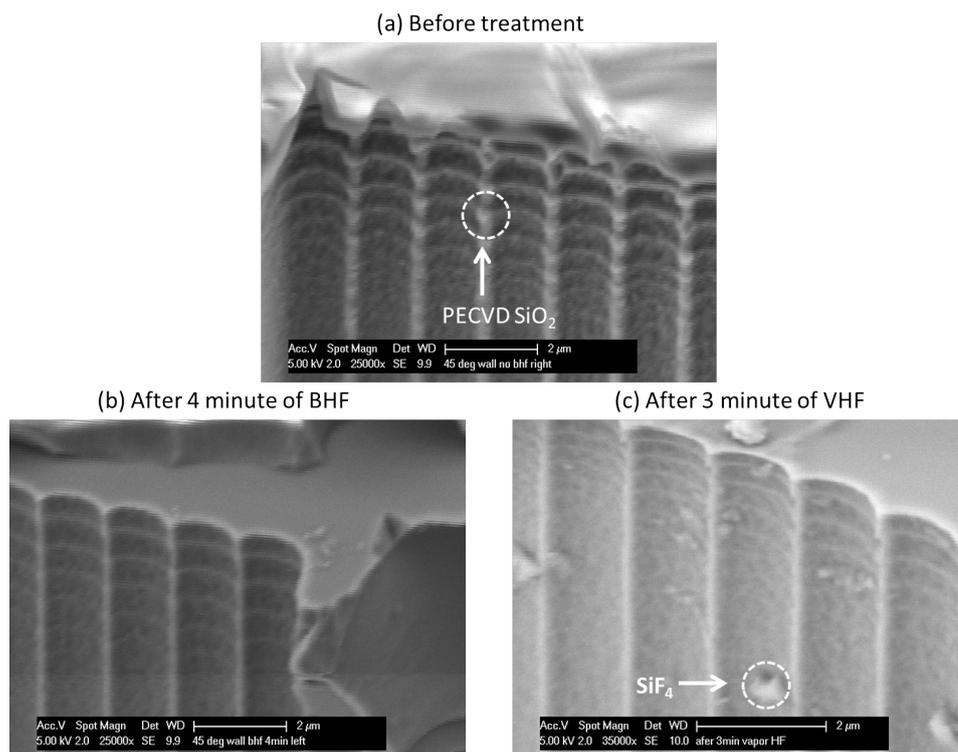
Figure 4.13: (a) Before treatment: PECVD SiO<sub>2</sub> is attached to the inner walls of the channel. (b) After buffered HF treatment for 4 min: PECVD SiO<sub>2</sub> is completely removed. (c) After 3 min vapor HF treatment for 3 min: The PECVD SiO<sub>2</sub> is removed but SiF<sub>4</sub>; the residue of the vapor HF (VHF) treatment is attached to the surface of the channel.
