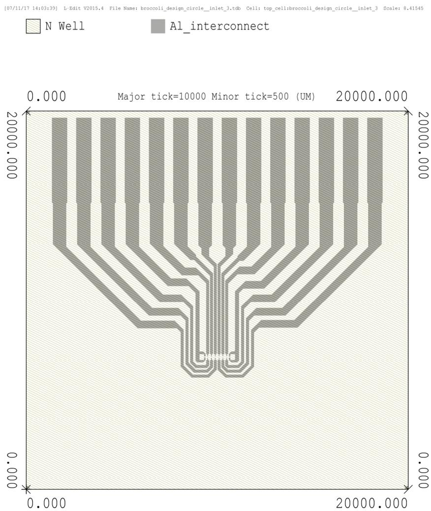
Figure A.2: Mask design of the aluminum interconnect. For this mask we use the inverted version of the mask.
