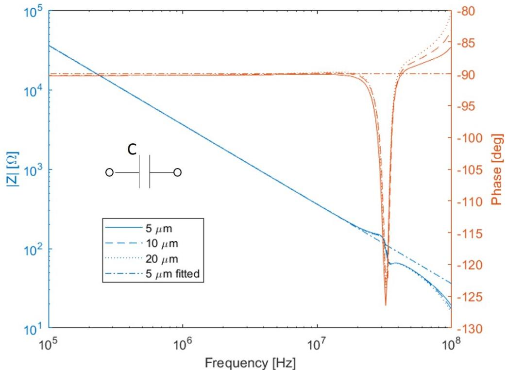
Figure 5.4: The impedance and phase for 5  $\mu\text{m}$ , 10  $\mu\text{m}$  and 20  $\mu\text{m}$  was measured between two ports when the channel was filled with air.
