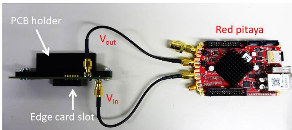
Figure 5.8: Overview of the experimental setup. Using redpitaya a voltage is applied to  $V_{in}$  and the output is monitored at  $V_{out}$ .
