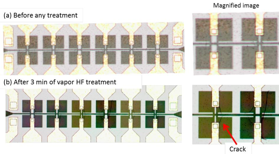
Figure 4.14: An image of the electrodes from above using a optical microscope before and after 3 min of vapor HF treatment. Cracks appear after the treatment as shown in the magnified image on the right with a red arrow.
