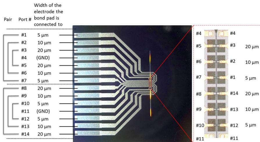
Figure 5.1: Details on the layout of the electrode and the bond pad. For convenience, each bond pad is assigned to a port number from #1 to #14 and the corresponding electrode that it is connected to is shown on the figure to the right.
