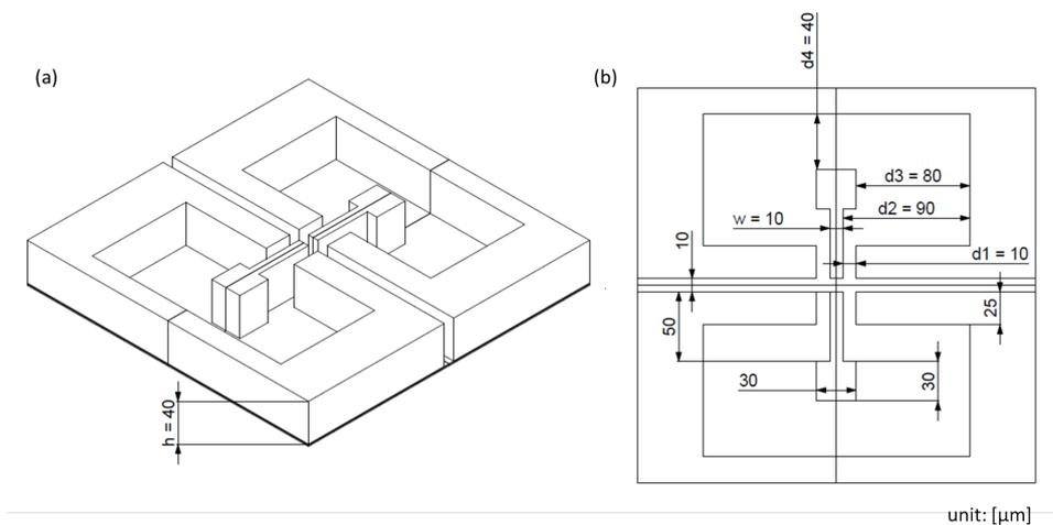
Figure 2.8: Geometry of the channel used in the model
