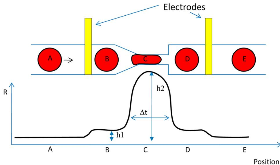
Figure 2.1: The impedance based measurement of cellular stiffness by A. Adamo et al [18].
