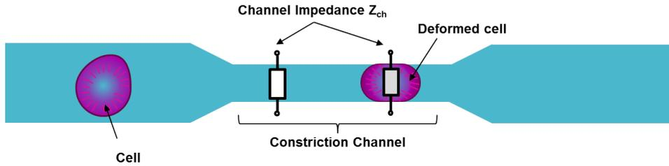
Figure 2.2: Channel impedance  $Z_{ch}$  is the impedance along the channel as shown. The channel impedance changes due to the presence of the cell.
