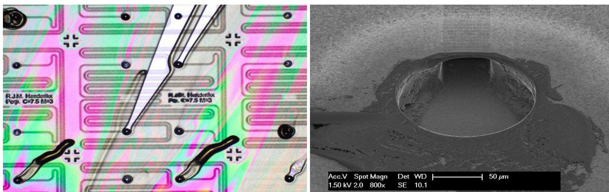
(a) After spin coating  $1.4\ \mu\text{m}$  of SPR3012 (b) After spray coating negative photoresist.
