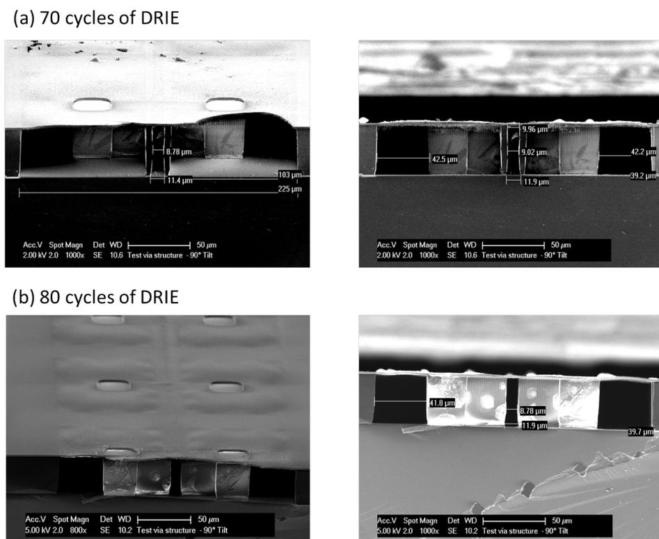
Figure 4.5: (a) After 70 cycle of DRIE seen from an angle -left and cross section - right. (b) After 80 cycle of DRIE seen from an angle - left and cross section - right
