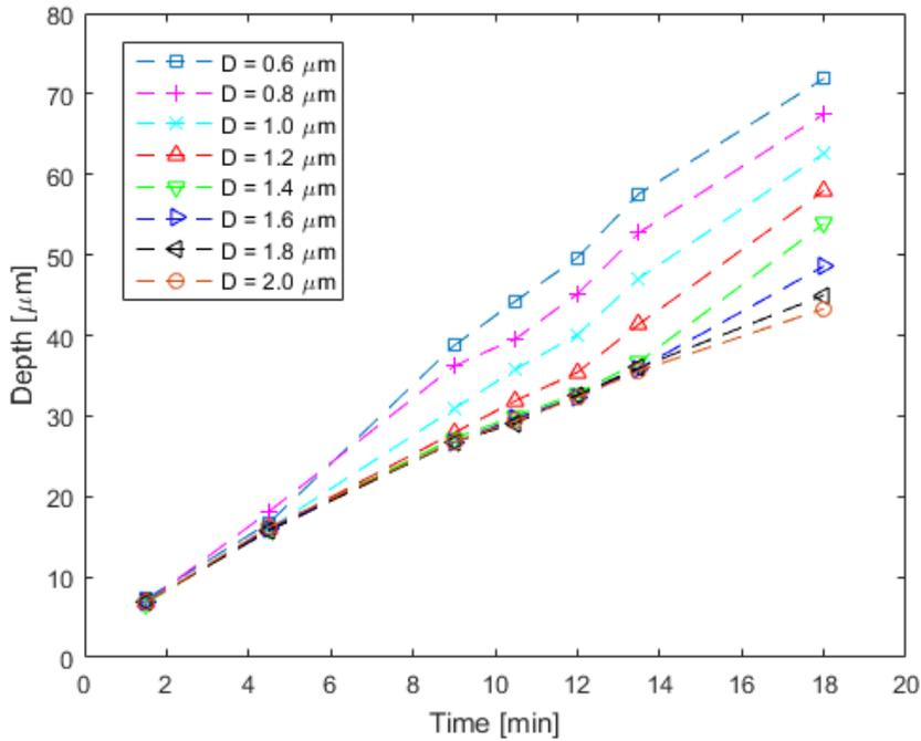
Figure 3.4: Depth of the channel during single step DRIE. The spacing between neighboring holes are varied from  $0.6 \mu\text{m}$  to  $2.0 \mu\text{m}$  in  $0.2 \mu\text{m}$  steps.
