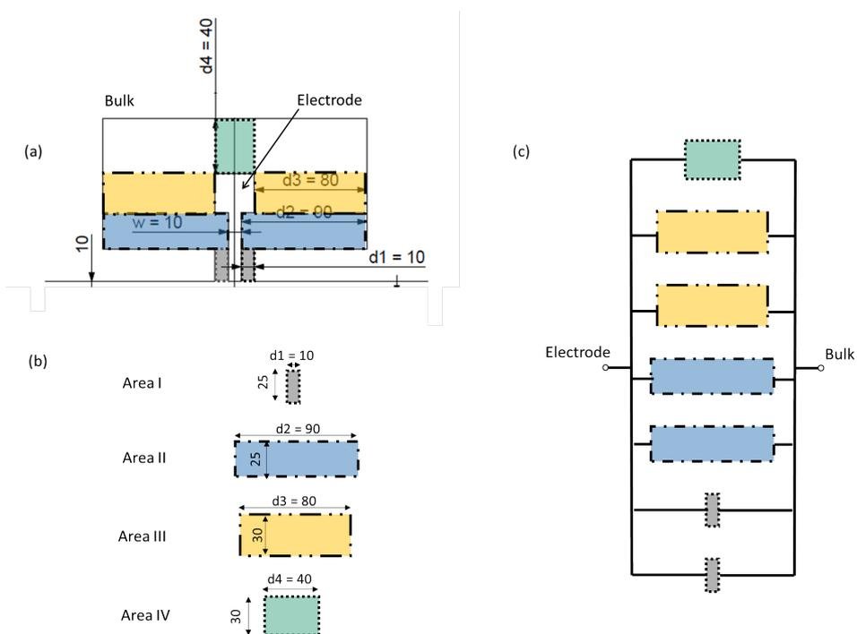
Figure 2.9: Area I to IV where the leakage occurs
