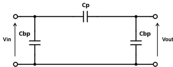
Figure 5.11: Electrical equivalent circuit when DI water is inside the channel.
