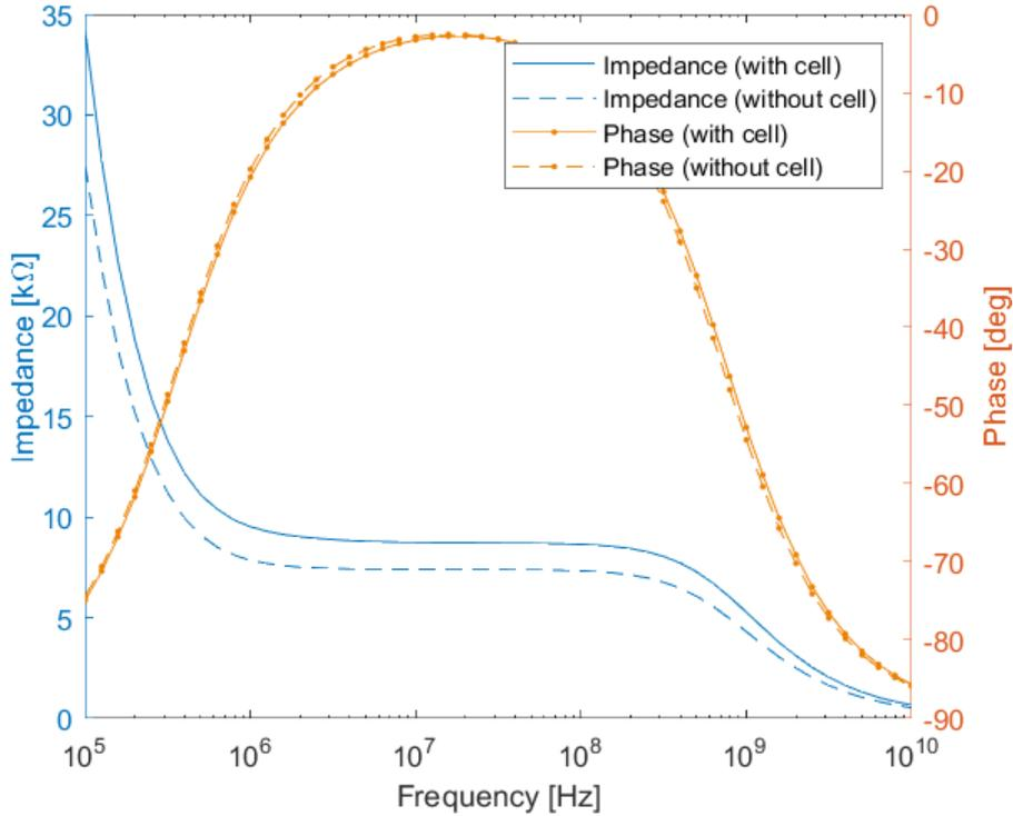
Figure 2.6: AC simulation result of the impedance and phase from 100 kHz to 10 GHz using LT-Spice when the cell is between the electrodes (with cell) and when the cell is not between the electrodes (without cell).
