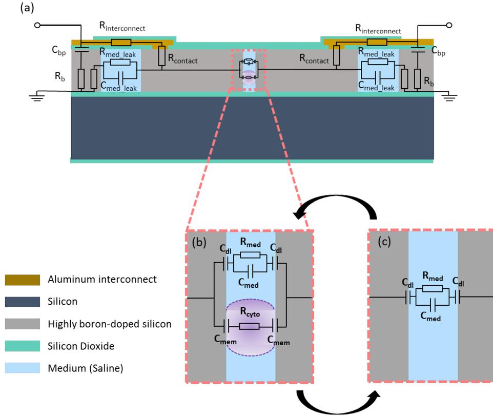
Figure 2.7: (a) Cross section of the channel with the corresponding circuit component. (b) Expanded view of the constriction channel when the cell is present. (c) Expanded view of the constriction channel when the cell is not present. The circuit values for this model are summarized in table 2.1
