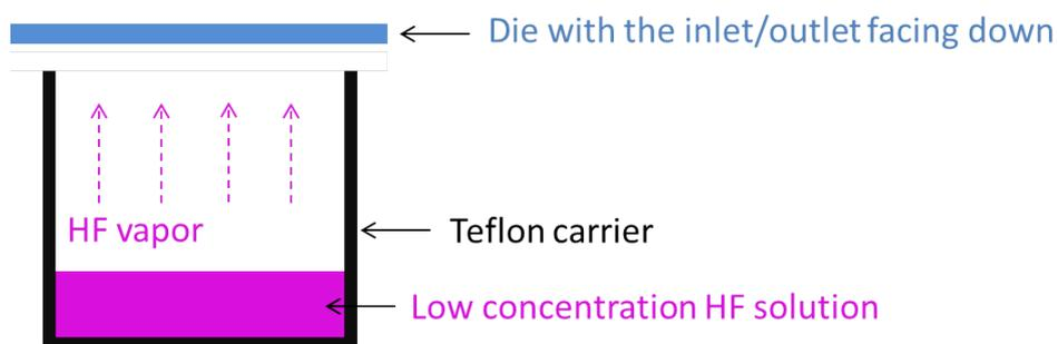
Figure 4.16: Use the evaporating HF from low concentration HF solution to etch the PECVD SiO<sub>2</sub> inside the channel at a mild rate.
