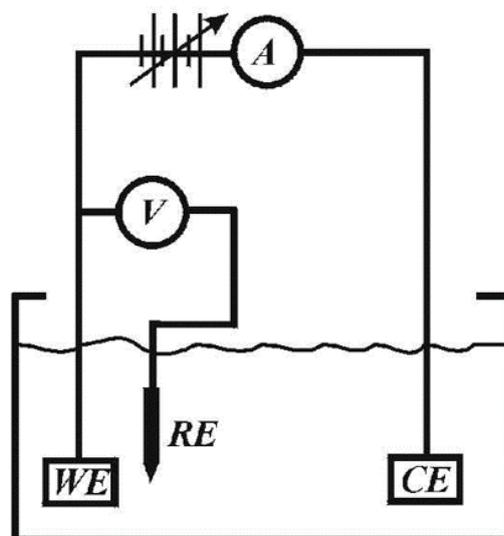
Figure 5.12: Schematic diagram of a 3 electrode schematic. A voltage is applied to the working electrode (Si) against the reference electrode (Ag/AgCl) and the current going through the counter electrode (Pt) is measured.
