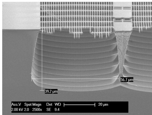
Figure 3.13: The total etch time was 9 min and the silicon etch per cycle was 12 s
