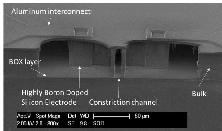
Figure 4.10: A SEM image of the cross section of the electrode and the constriction channel.
