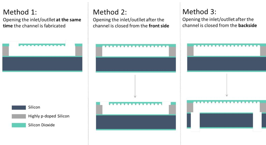
Figure 4.1: Inlet opened simultaneously when the channel was being fabricated.
