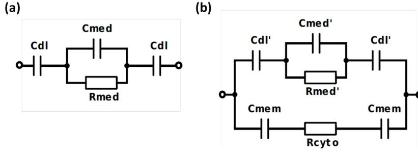
Figure 2.4: Channel impedance model based on Foster and Schwan [21]. The model consists of a double layer capacitance  $C_{dl}$ , medium capacitance  $C_{med}$ , medium resistance  $R_{med}$ , membrane capacitance  $C_{mem}$  and cytoplasm resistance  $R_{cyto}$ .  $R_{med}'$  and  $C_{med}'$  denotes the value when the cell is between the pair of electrodes. (a) Channel impedance without the cell ( $Z_{ch}$ ) (b) Channel impedance with the cell ( $Z_{ch}'$ )
