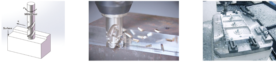
Figure 2.6: Milling is a reductive manufacturing technique based upon the principle of removing material in order to obtain a component such as the one that is illustrated (right) [22].
