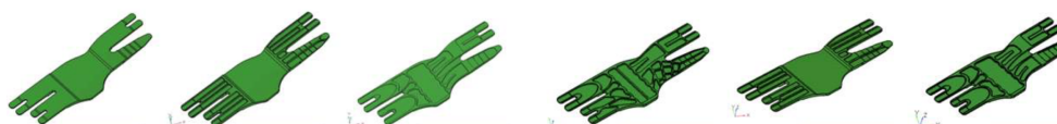
Figure 1.4: The effect of variable design features on distortion is evaluated for a H-plate component. Six different designs were considered which vary in thickness and in the type of stiffeners used [10].
