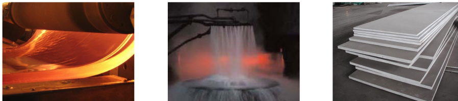
Figure 2.3: The two most dominant stress-inducing processes in the primary production processes, being hot rolling (left) and quenching (middle), where rolled plate stock material (right) is formed from raw material [18].
