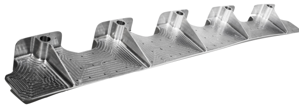
Figure 3.23: A structural bracket belonging to the AIRBUS A350 aircraft [41].
