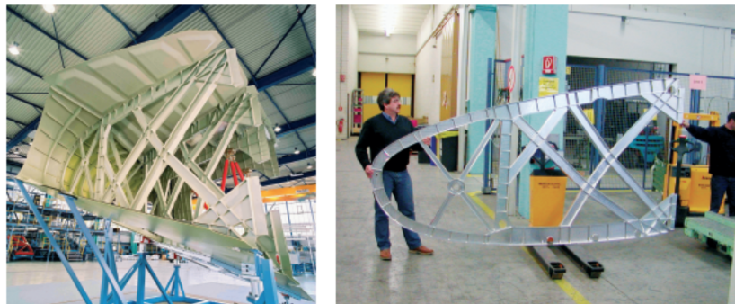
Figure 1.1: An optimized wing rib section (right) using topology optimization that fits into the wing box (left) belonging to the AIRBUS A350 aircraft [1].
