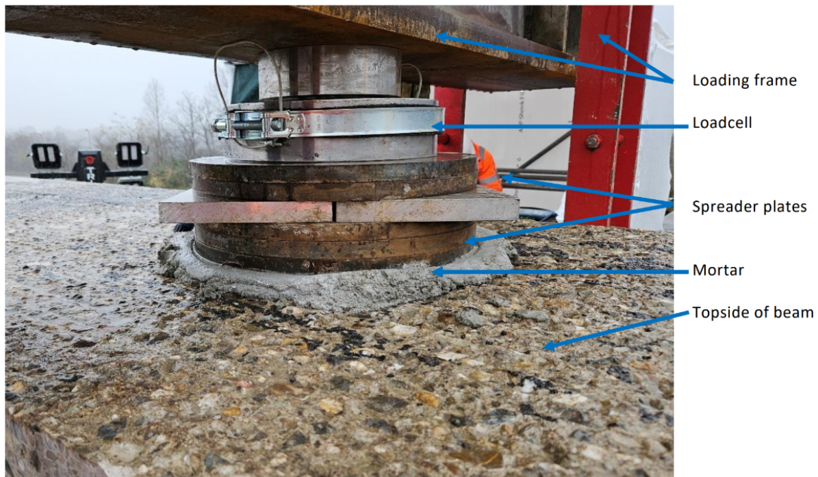
Figure 4.5: Load application joint (Howse et al., 2025)
