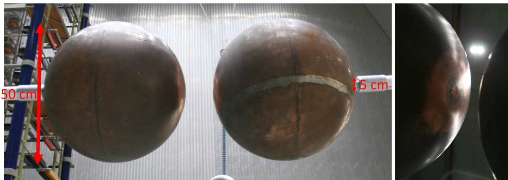
Figure 15.8: Sphere-Sphere gap with a sphere diameter of 50 cm
