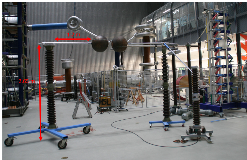
Figure 15.10: High voltage test setup with Sphere-Sphere electrodes
