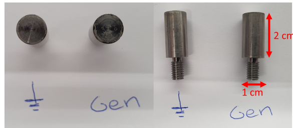
Figure 15.7: Tips that are used for the Rod-Rod setup, with labels for the earthed side and the high voltage side.
