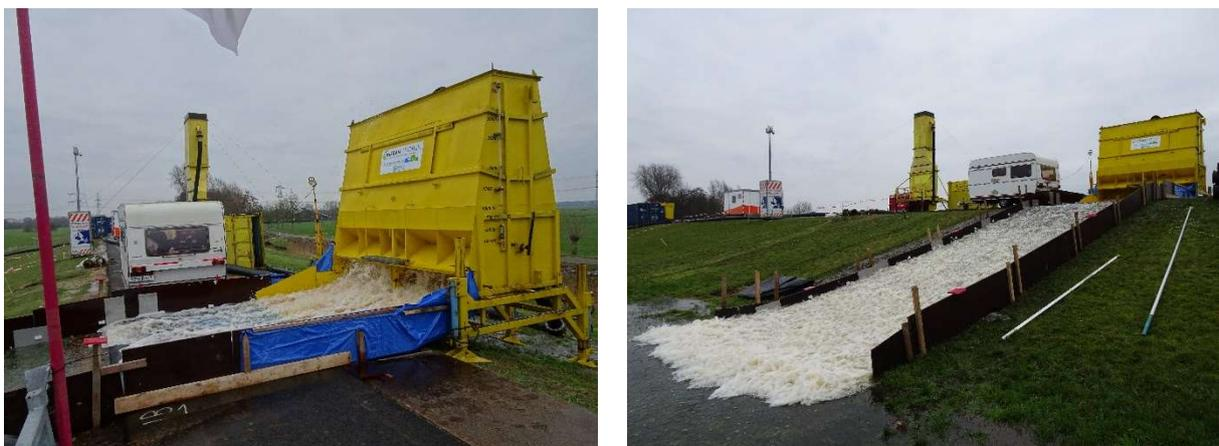
Figure 6 Wave Overtopping Simulator in deployment during a field visit in January 2021 on the Vechtdijk, Zwolle (NL)
