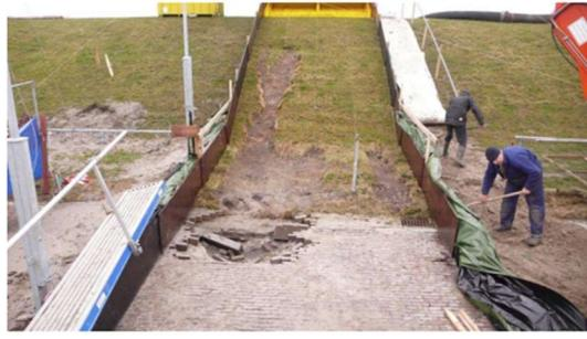
Figure 33 Left: after 10 l/s per m sessions. Right: after experiment termination, 4hr and 20min of 30l/s per meter. Af2.
