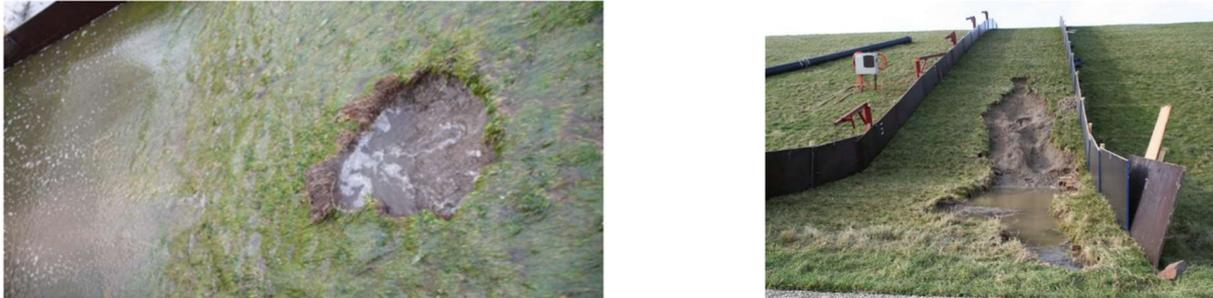
Figure 29 Left: first grass cover failure after 1.5hr. Right: End result, including the 30min extension. Bo3.
