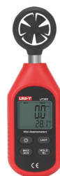
Figure 5.8 | Photo of the anemometer that is used in the test set-up | Source: own work
