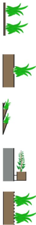
Figure 3.5 | Schematic examples of five non-ground-based systems. From top to bottom: Geotextile systems, Panel systems, Tray systems, Combination systems and Continuous soil cores | Source: (Damen et al., 2014, p.60)
