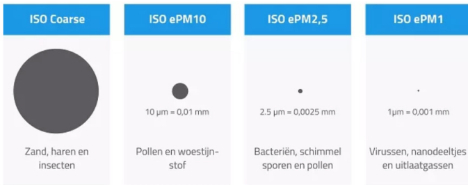
Figure 2.3 | Overview of the different filter classes for particulate matter and what type of particles they can filter | Source: (Robathern, 2021)
