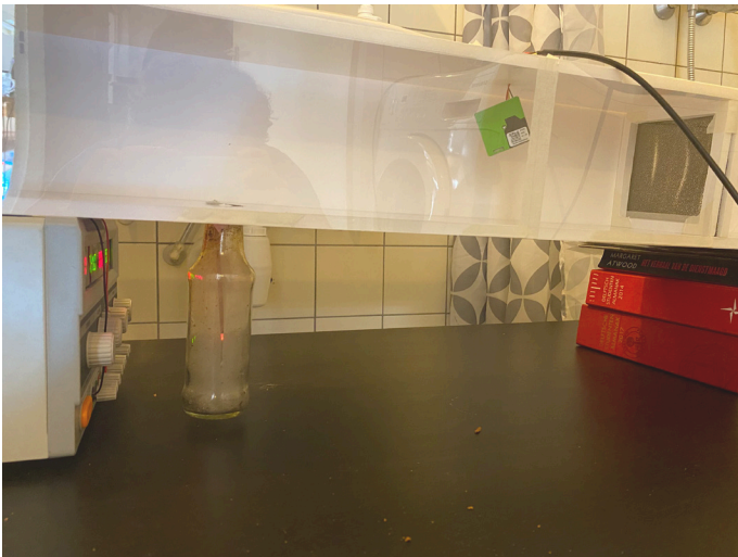
Figure 5.1 | Close-up photo of the lab power supply, the fan, and the incense as a source of smoke | Source: own work
