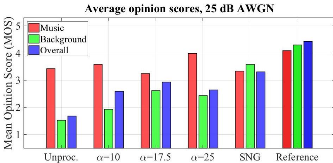
Figure 4.3: Average opinion scores per method and per added noise intensity. The results were obtained by averaging the scores given by the participants, and subsequently taking the mean of all four instrument recordings processed in that particular way. In addition to the four processing approaches, the ratings of the unprocessed noisy reference (far left, denoted 'Unproc.') and noise-free reference (far right, denoted 'Reference') are shown for comparison.
