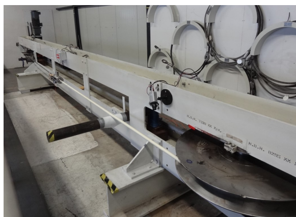
(b) CBoS Machine used for Ageing Cables with Armour
