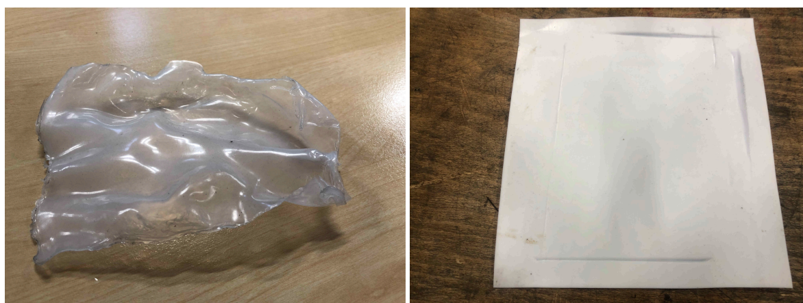
(a) Deformation due to sudden cooling of XLPE
