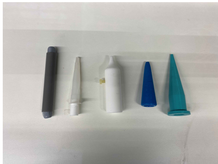
Figure B.3: Bushing trials made of different materials done starting from the left (a) PVC pipe with water-tight cap, (b) modified glue cap, (c) Teflon cone, (d) PET cone, and (e) TPU cone.
