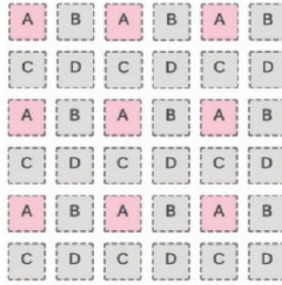
Figure 4.2: The qubit plane architecture proposed in [18] for lattice surgery-based planar surface codes, where each patch can hold one logical qubit shown in Figure 4.1a.
