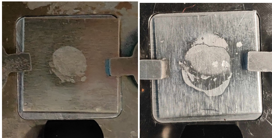
(a) X3, 31-01, cohesive failure
