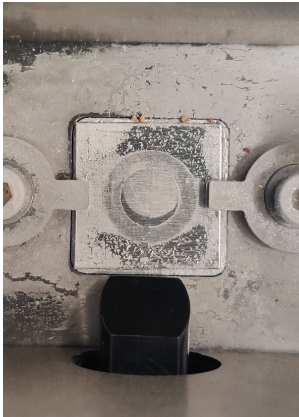
Figure 4.8: Example 1 of frost growth inside chamber and sample surfaces due to a lack of humidity control
