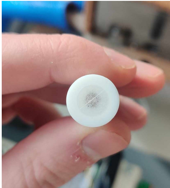
Figure 7: Hairline fracture on unpolished AA-608
