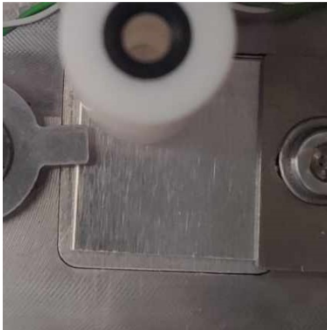
(a) X5, 31-01, clean adhesive failure
