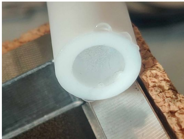
Figure 6: Spilling under mould, which was a prevalent error on polymer substrates.
