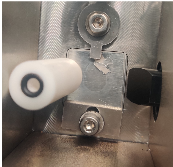
Figure 4.10: Evidence of a spill at slot X1, on an aluminium sample
