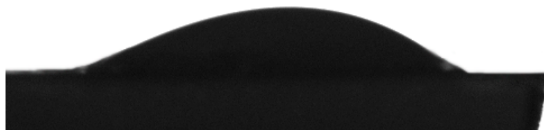
Figure 5.17: WCA of 40° on hydrophilic poly-HEMA coating.
