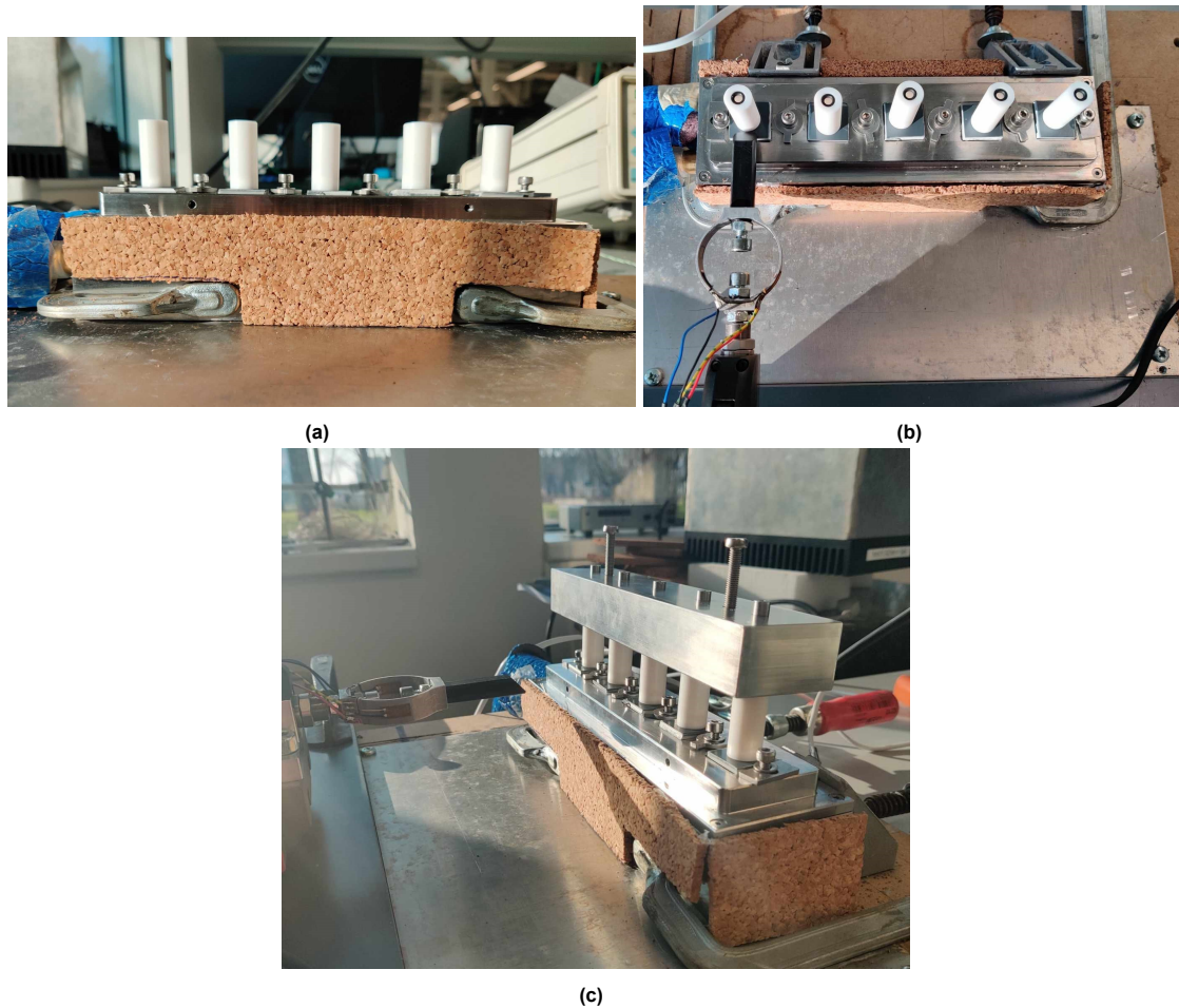
Figure 3.12: Set-up without housing chamber for visualisation. (a) Front view and (b) Plan view of moulds on samples, (c) Isometric view with alignment block. By careful removal of the alignment pins, the block can be removed from the moulds when the ice pillars are frozen.
