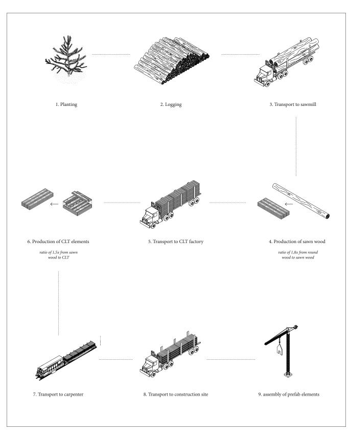
fig. 01: timber supply chain diagram from resource extraction to the construciton on site
