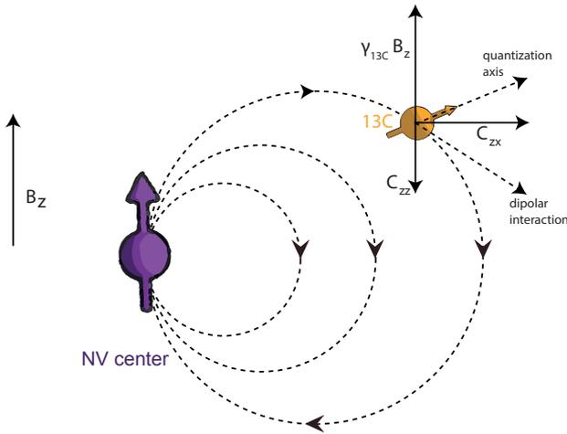
Figure 5.3:  **$^{13}\text{C}$  spin in a dipole field.** Exemplary case in which the  $J_z I_x$  interaction causes its quantization axis to become more aligned with the dipole field direction due to the the NV ( $m_s = -1$ ) given the condition  $C_{zz} < \gamma_{13\text{C}} B_z$ . The same holds for the NV in  $m_s = +1$ , in this case the direction of the dipole field and thus  $C_{zx}$  and  $C_{zz}$  change to their direct opposite.
