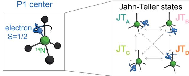
Figure 2.5: **P1 center in diamond.** Left: the P1 center surrounded by four carbon atoms in the diamond lattice. Right: the P1 center exhibits a Jahn-Teller distortion along one of the four  $^{14}\text{N} - \text{C}$  bonds (labelled as  $\{A, B, C, D\}$ ) that can vary over time.
