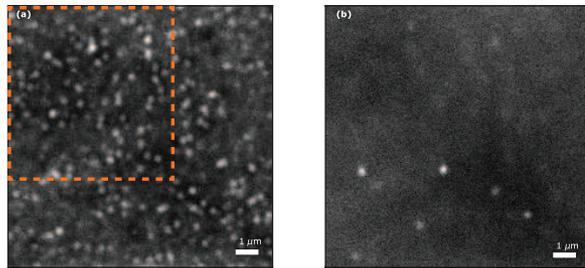
Figure 3.10: **Confocal scans of sample B (a)** at the implantation depth and **(b)** at  $\approx 5 \mu\text{m}$  under the diamond surface. The orange box indicates the approximate region at the implantation depth in which fluorescent spots were characterized.
