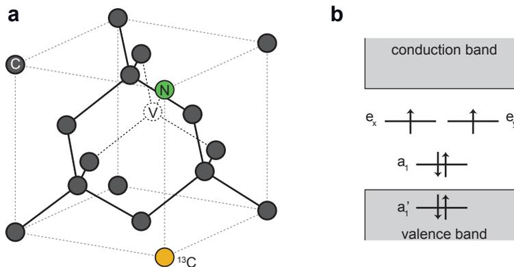
Figure 2.1: **The nitrogen-vacancy (NV) center in diamond.** a) The crystal structure of diamond. The NV center is formed by a substitutional nitrogen atom next to a vacant lattice site. The carbon atoms in the diamond lattice consist for  $\sim 1.1\%$  of  $^{13}\text{C}$  isotopes with nuclear spin-1/2 (yellow). b) The NV molecular orbitals and their occupation in the electronic ground state. Figures adapted from Pfaff [31], Bernien [32].
