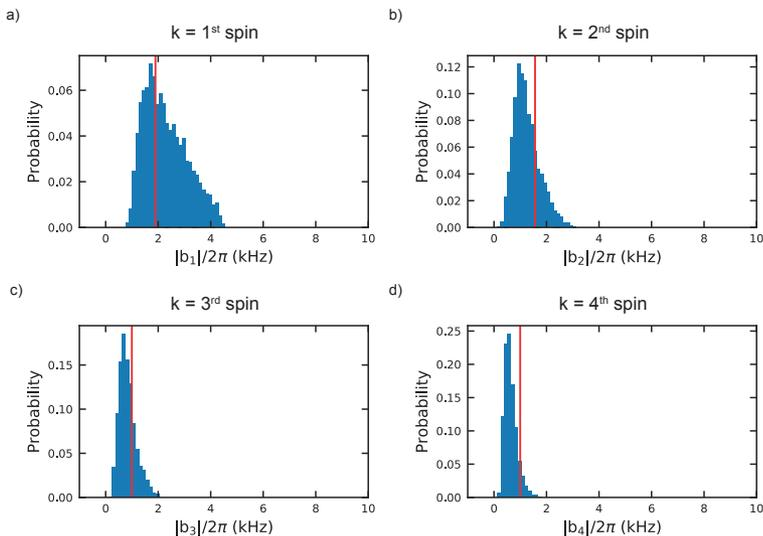
Figure 4.11: **Simulated distributions of the coupling strengths for the most strongly coupled P1 spins.** a),b),c),d) Distributions of  $|b_k|/2\pi$  given  $4 \text{ kHz} \leq 1/T_2^* \leq 10 \text{ kHz}$  and a concentration  $C_d = 75 \text{ ppb}$ .
