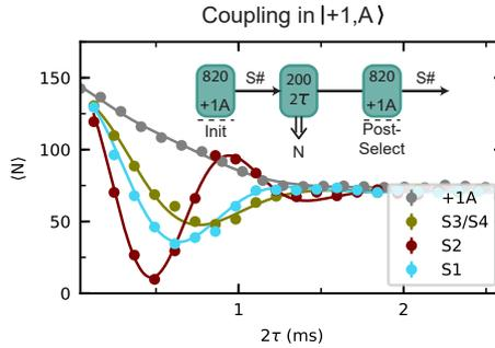
Figure A.2: **Measuring NV-P1 coupling strength in  $|+1, A\rangle$ .** We initialize S1, S2 or S3/S4 in  $|+1, A\rangle$  and vary the interaction time  $2\tau$  of a DEER sequence ( $K=200$ ). To improve the signal, the results are post-selected on again obtaining  $|+1, A\rangle$ . Inset: experimental sequence. Grey: without P1 initialisation (data from Fig. 4.1c, chapter 4).
