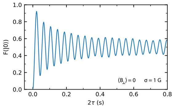
Figure 5.10: **Simulation of the nitrogen thermal echo.** The simulated fidelity of the NV electron spin after a nitrogen thermal echo sequence (see Fig. 5.6), under Gaussian distributed perpendicular magnetic field noise,  $\langle B_{\perp} \rangle = 0$ , with standard deviation  $\sigma = 1$  G. Numerical simulations of  $10^3$  sampled  $B_{\perp}$  values from this distribution are performed and averaged to emulate quasi-static Gaussian distributed noise.
