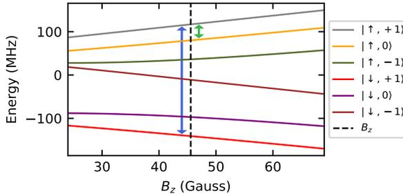
Figure 4.18: **Energy levels for a single P1 center in JT axis D.** Simulation of the six energy levels which are labelled according to their P1 electron and nitrogen nuclear spin state. The black dashed line denotes the experimental magnetic field value. The green (blue) double headed arrow indicates the transition used in the nitrogen (electron) coherence experiments (Fig. 4.6c,d)
