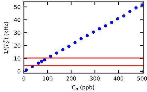
Figure 4.10: Simulated  $1/\langle T_2^* \rangle$ . Simulation based on  $m = 10^4$  different defect configurations of  $N_d = 40$  defects. The red vertical lines indicate estimated bounds for  $1/\langle T_2^* \rangle$ .
