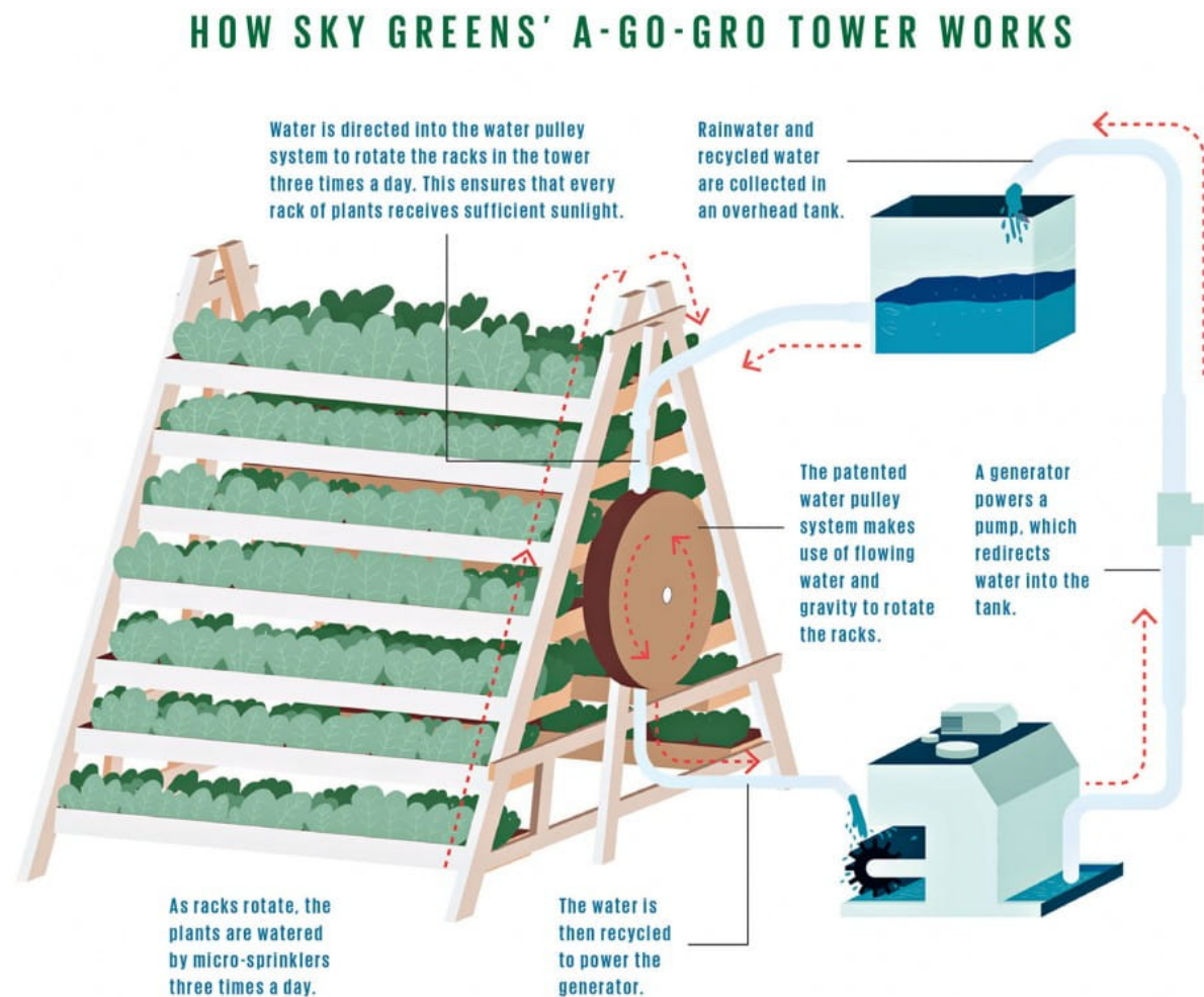
Figure 3.5: The operating principles of Sky Greens' A-Go-Gro tower. Reprinted from "Singapore Magazine: Farming in the Sky" (2015).
