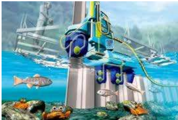
Figure 3 Seabed piling rig ( www.giken.com )
