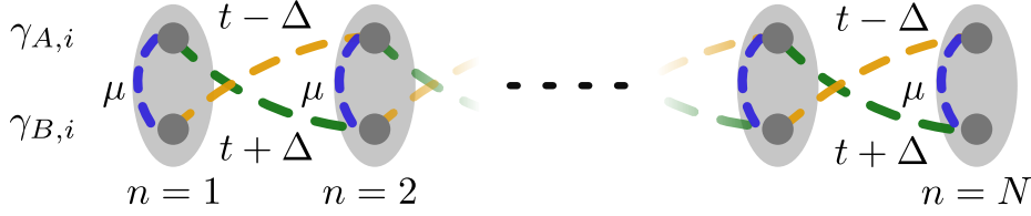
Figure 1.2: Kitaev chain in the Majorana basis. Each electronic site is split into two Majoranas which couple through the chemical potential, \mu , on each site. Between sites, coupling is mediated by combinations of normal hopping, t , and p-wave pairing, \Delta . At \mu = 0 and |t| = |\Delta| , the onsite couplings and one diagonal coupling vanish, isolating a single Majorana on the terminating sites.
