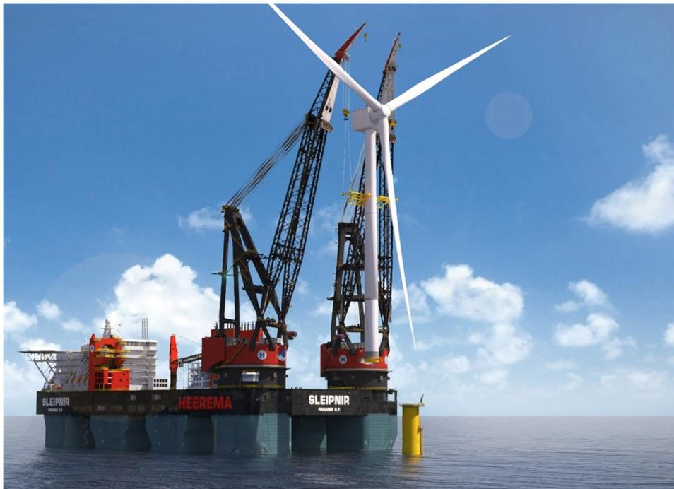
Figure 1.4: Render of dual crane whole WTG installation with SSCV Sleipnir
