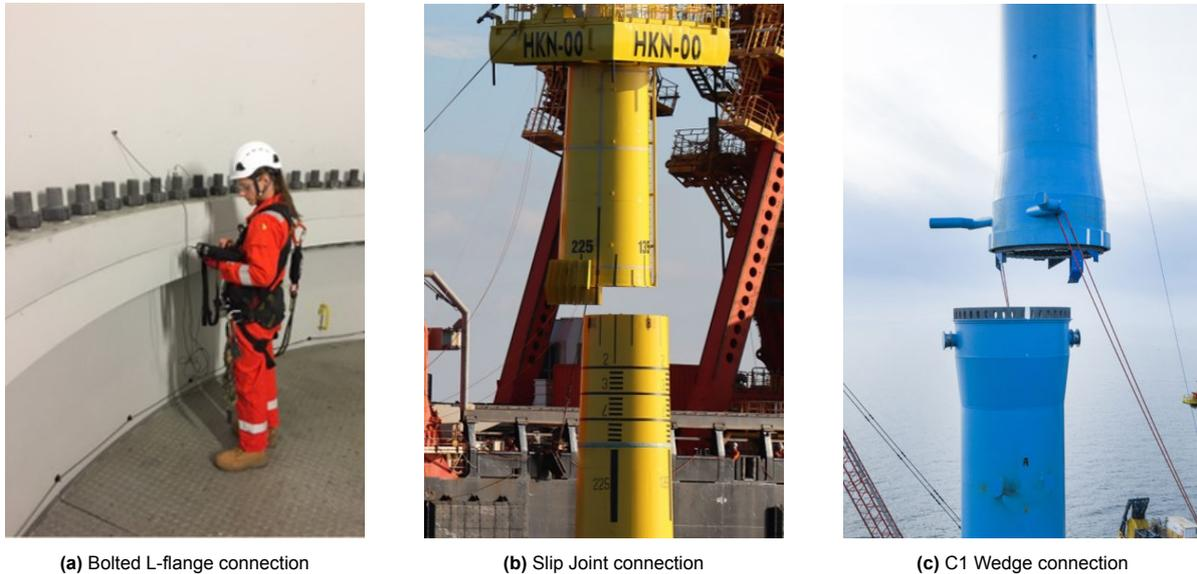
**Figure 2.12:** Three connection types used in offshore wind turbines [31, 30, 12].
