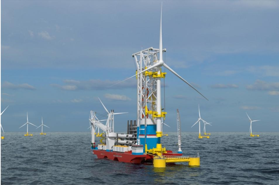
**Figure 2.9:** Windfarm Installation Vessel (WIV) concept by Huisman [9].
