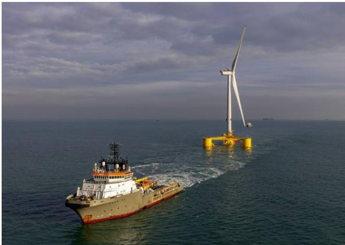
(b) Feeder transport strategy example of Boskalis' Manta towing a pre-assembled WTG on a semi-submersible floating support structures [98]. Note that this is a possible example of how a feeder strategy could be executed. In the project related to this figure, the transport was not for feeder purposes.
