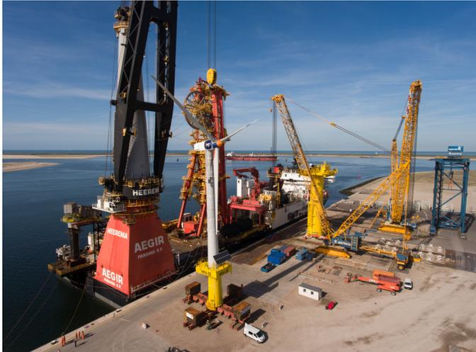
(a) Shuttling transport strategy example of HMC's Aegir lifting the DOT SJOR Turbine before sailing to the OWF [94].
