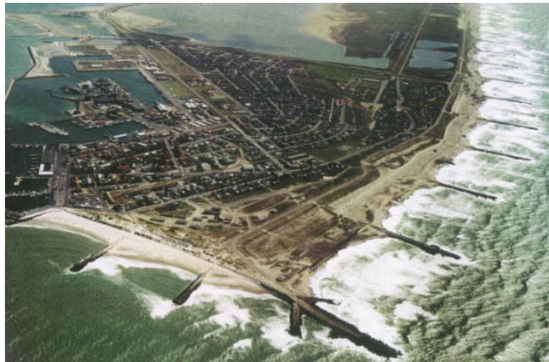
Fig. II-18. Coastal protection with excessive system of groins, Jutland, Denmark
