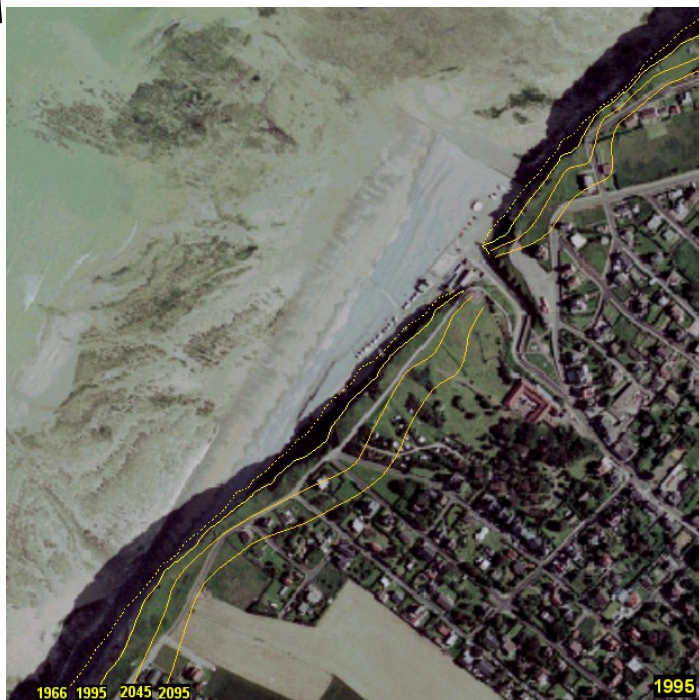
Fig. III-19. Approach for estimating cliff erosion rates and future coastline positions
