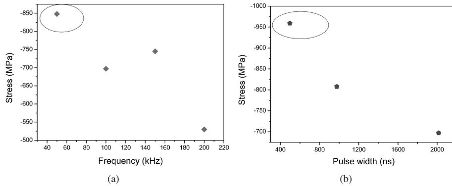
Figure 6.4: Residual stress as a function of (a) frequency and (b) pulse width. Ellipses indicate the selected parameters.
