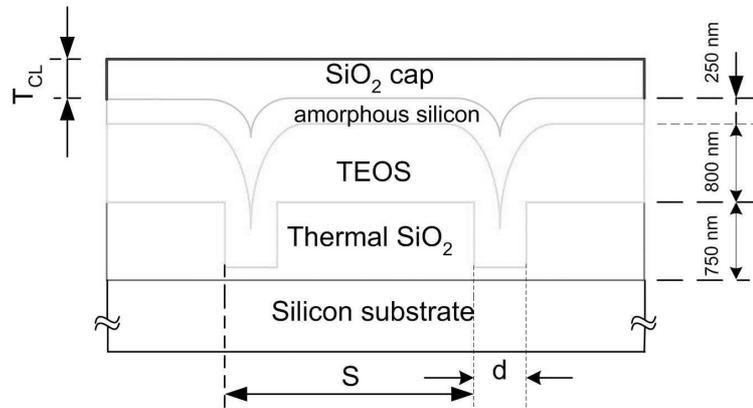
Figure 3.1: Schematic cross-sectional view of a grain filter with a capping layer: the thickness  $T_{CL}$  of the capping layer varies from 200 to 500 nm in 100 nm steps; the grid spacing ( $S$ ) varies from 3 to 15  $\mu\text{m}$ ; the original diameter of the grain filter ( $d$ ) is fixed at 1.0  $\mu\text{m}$ .
