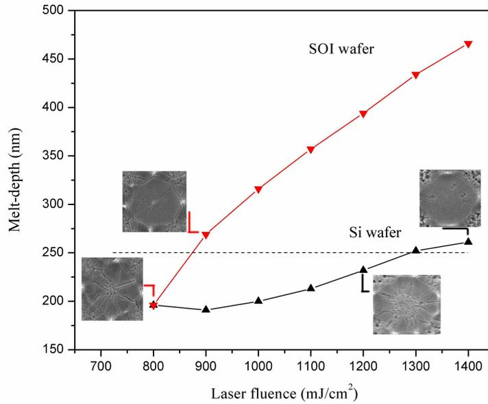
Figure 3.7: Simulated melt depth as a function of laser fluence. The insets show the corresponding grain morphologies observed experimentally.
