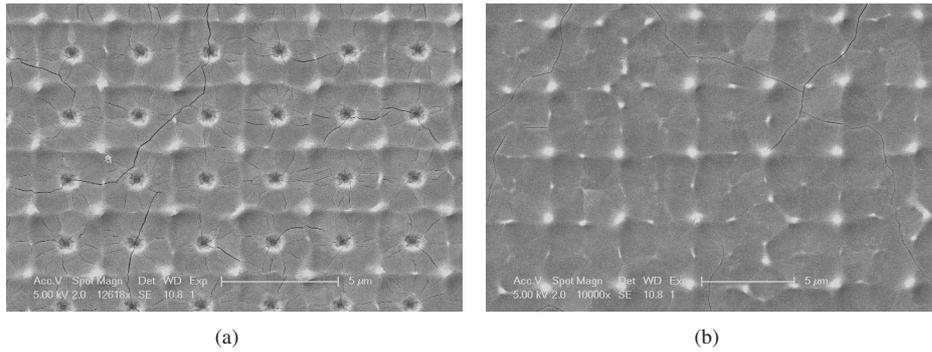
Figure 5.7: SEM images of location-controlled grains crystallized at room temperature with a laser fluence of (a) 700 mJ/cm<sup>2</sup>, and (b) 1140 mJ/cm<sup>2</sup>. Cracks are clearly visible in both images.
