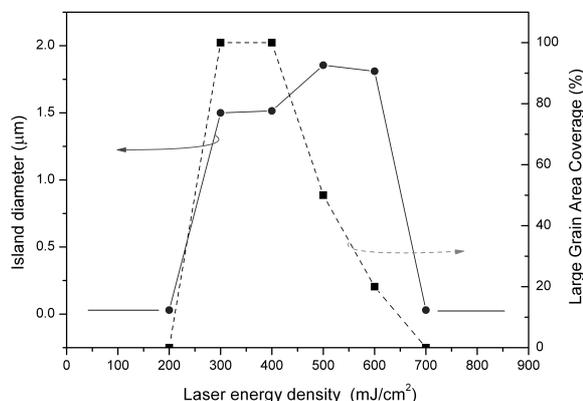
Figure 6.6: Diameter of laterally grown grains and large-grain area coverage for a 122 nm  $\alpha$ -Si layer (wafer No. E15) as a function of the energy density of the laser pulse.
