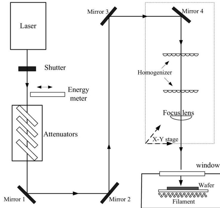
Figure 2.1: Schematic representation of the XMR 7100 system. The energy meter can be moved into the laser path to measure the energy density of the laser output. The energy density at the wafer surface is tuned by the laser spot size. The dotted rectangle indicates an X-Y stage, onto which mirror 4, the homogenizer, and the focus lens are mounted. During laser processing, the X-Y stage moves, whereas the wafer stays stationary.
