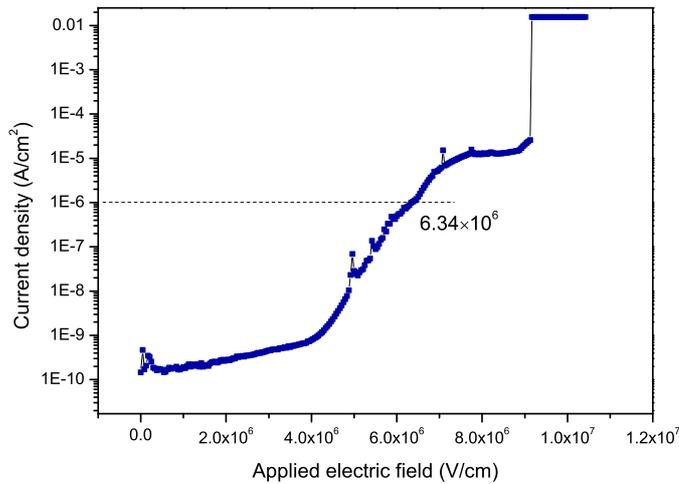
Figure 6.13: Current density ( $I$ ) vs. applied electric field ( $E$ ) characteristics for Al/SiO<sub>2</sub>/p-type Si MOS capacitors. The breakdown field is  $6.34 \times 10^6$  V/cm; the resistivity is  $5.20 \times 10^{15}$  Ω·cm.
