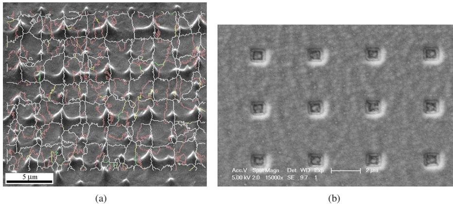
Figure 5.10: Defects generated during epitaxial growth from the seeding layer. (a) SEM image overlaid with a grain-boundary-component map, indicating large grain boundaries inside one island and normally four grains per hole. (b) Top view of square-shaped holes, where grains start to grow from the seeding layer.
