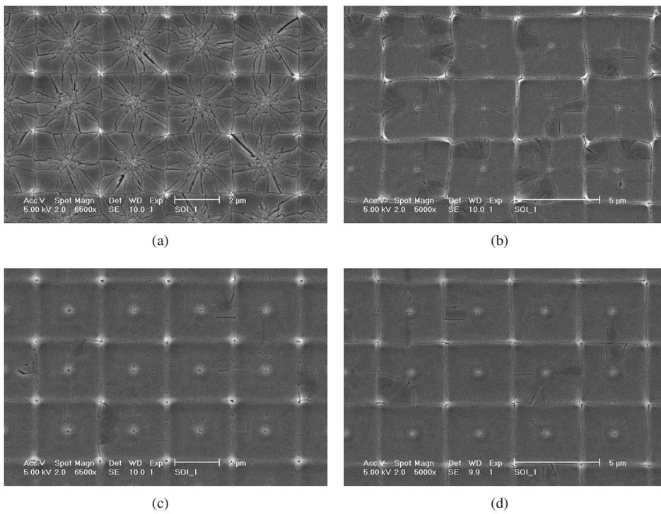
Figure 3.6: Grains grown from (100)-oriented SOI wafers with a wet soft-landing step (method (i)); the step height is 450 nm and the substrate is heated up to 450°C with a laser fluence of (a) 800 mJ/cm<sup>2</sup>, (b) 900 mJ/cm<sup>2</sup>, (c) 1000 mJ/cm<sup>2</sup>, and (d) 1300 mJ/cm<sup>2</sup>.
