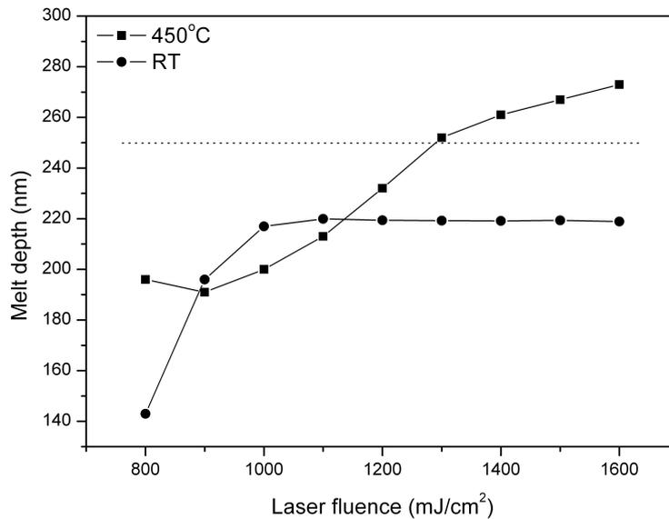
Figure 3.9: Simulated melt depth as a function of laser fluence for a bulk silicon seed crystallized at room temperature (RT), and with substrate heating to 450°C. Without substrate heating the melt depth saturates before reaching the  $\alpha$ -Si/c-Si interface.
