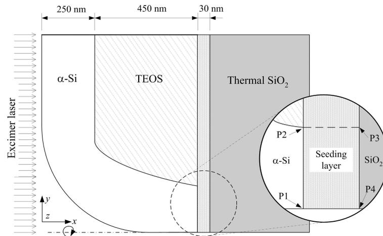
Figure 5.3: Schematic diagram of the axisymmetric configuration for simulating epitaxial growth from the seeding layer. The symmetry axis is along the  $x$ -direction. Points of special importance, P1, P2, P3, and P4, are marked in the inset image.
