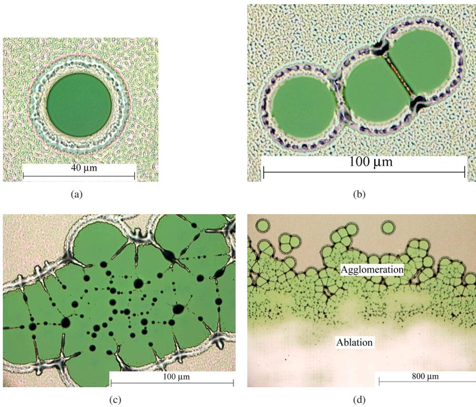
Figure A. 5: Optical images of agglomeration in  $\alpha$ -Si films irradiated with an energy density of (a) 1385  $\text{mJ}/\text{cm}^2$ ; (b) 1549  $\text{mJ}/\text{cm}^2$ ; (c) 1793  $\text{mJ}/\text{cm}^2$ ; (d) 1893  $\text{mJ}/\text{cm}^2$ .
