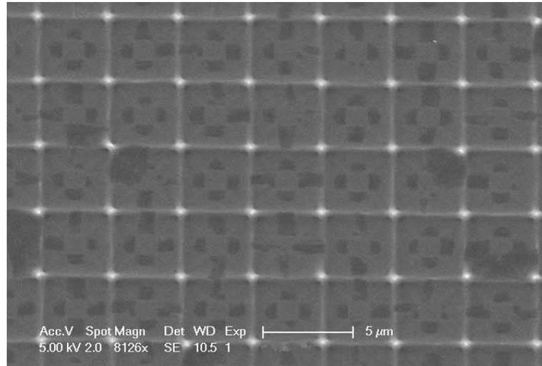
Figure 3.12: Grains produced from a (100)-oriented wafer with a dry soft-landing step (method ii) using excimer-laser crystallization and substrate heating to 450°C with a laser fluence of 1400 mJ/cm<sup>2</sup>.
