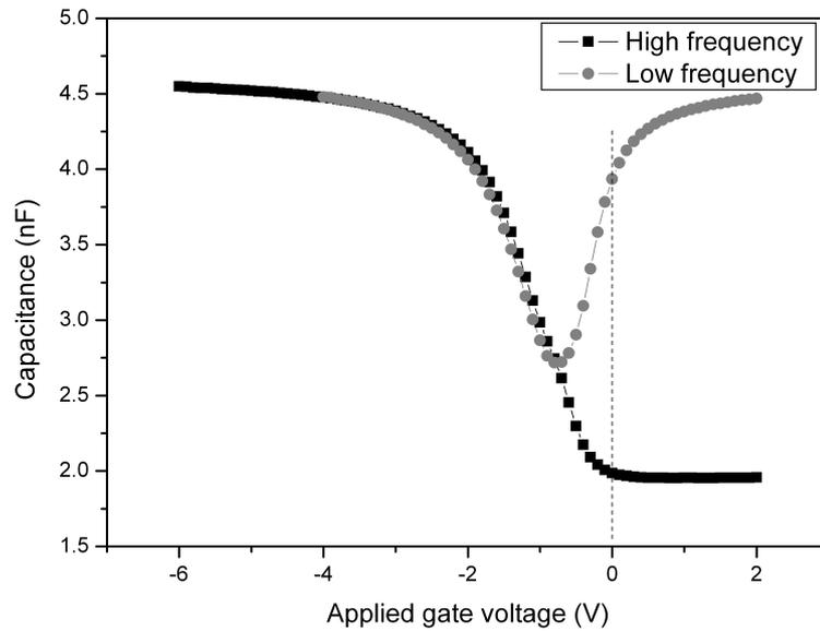
Figure 6.14: Capacitance vs. applied gate voltage curves for Al/ $\text{SiO}_2$ /p-type Si MOS capacitors;  $\text{SiO}_2$  is deposited at  $80^\circ\text{C}$ .
