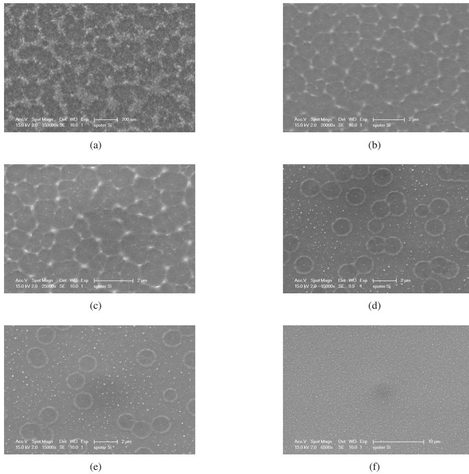
Figure 6.5: SEM images of grains grown from a 122 nm thick  $\alpha$ -Si film (wafer No. E15) crystallized at: (a) 200  $\text{mJ}/\text{cm}^2$ ; (b) 300  $\text{mJ}/\text{cm}^2$ ; (c) 400  $\text{mJ}/\text{cm}^2$ ; (d) 500  $\text{mJ}/\text{cm}^2$ ; (e) 600  $\text{mJ}/\text{cm}^2$ ; and (f) 700  $\text{mJ}/\text{cm}^2$ .
