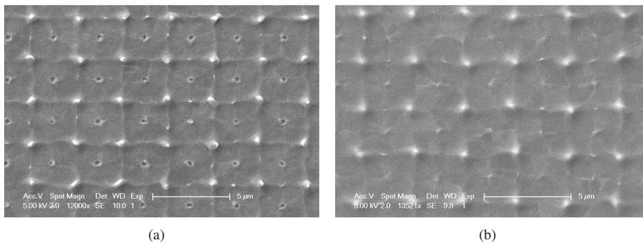
Figure 5.8: SEM images of location-controlled grains crystallized with substrate heating up to 450°C, with a laser fluence of (a) 960 mJ/cm<sup>2</sup>, and (b) 1020 mJ/cm<sup>2</sup>.
