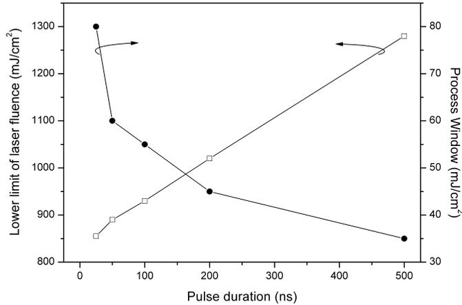
Figure 5.6: Effects of laser-pulse duration on the process windows for orientation- and location-controlled grains.
