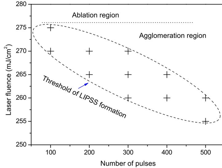
Figure 4.5: Energy density window for obtaining textured self-assembled poly-Si grains. Crosses indicate experimental points where textured self-assembled poly-Si grains were obtained. The dashed ellipse indicates the laser energy density window, taking into account the number of shots. The dotted line separates the ablation region from the agglomeration region.
