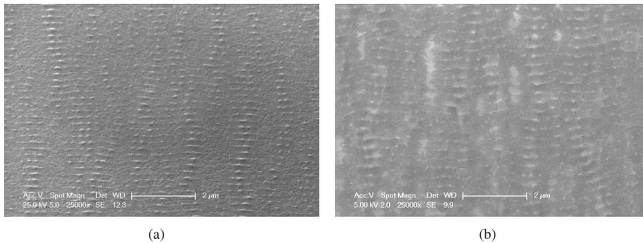
Figure 4.7: SEM images of poly-Si grains crystallized at  $280 \text{ mJ/cm}^2$  after 500 shots. (a) Periodic grain boundaries; (b) high-resolution image of the periodic grain boundaries.
