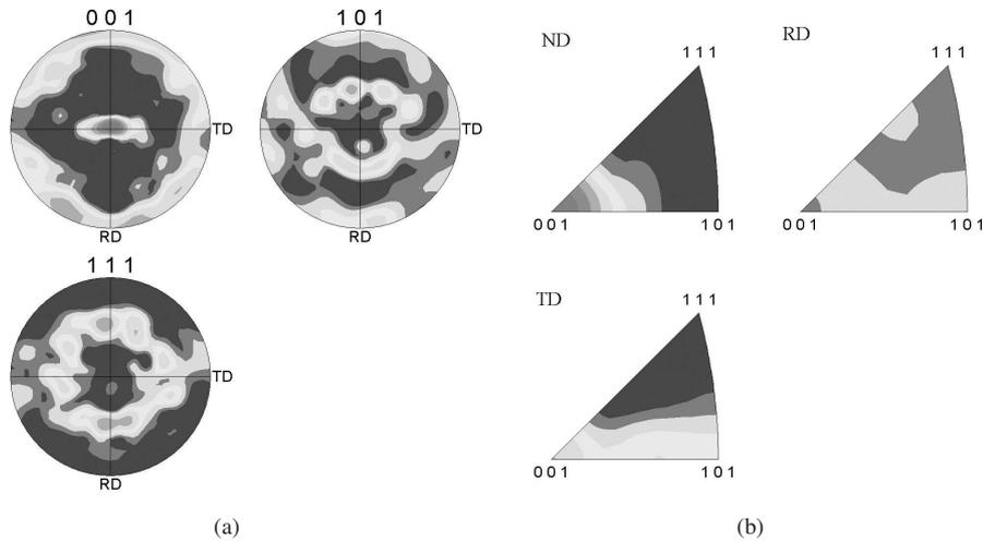
Figure 4.8: Microtexture of poly-Si grains, crystallized at  $280 \text{ mJ/cm}^2$  after 500 shots. (a) Pole figures for  $\langle 100 \rangle$ ,  $\langle 110 \rangle$ , and  $\langle 111 \rangle$  orientations. (b) Inverse-pole figures of ND, RD and TD.
