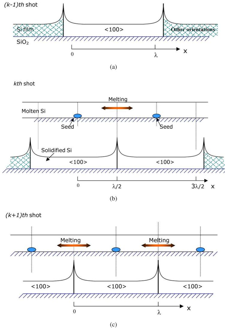
Figure 4.9: Schematic representation of the development of the  $\langle 100 \rangle$  texture through three successive shots during LIPSS formation. After the  $(k - 1)$ th shot a  $\langle 100 \rangle$ -oriented grain grows largest. After the  $k$ th shot two seeds survive the melting phase, hence the length of the  $\langle 100 \rangle$  direction is doubled. After the  $(k + 1)$ th shot three seeds are present, so the length of the  $\langle 100 \rangle$  direction is tripled.
