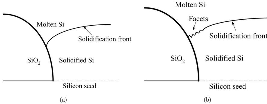
Figure 3.18: Schematic representation of facet formation at the three-phase boundary: (a) facets are absorbed at the boundary, and the l-Si/c-Si interface remains smooth; (b) facets are not absorbed, and the l-Si/c-Si interface near the three-phase boundary (TPB) features facets.
