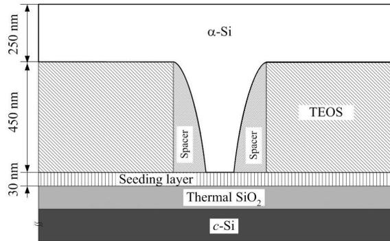
Figure 5.1: Schematic cross-sectional view of stacked layers for crystallographic orientation and location control. The  $\alpha$ -Si layer is applied directly on a TEOS oxide layer, with an opening to the seeding layer that has a  $\langle 100 \rangle$  texture.
