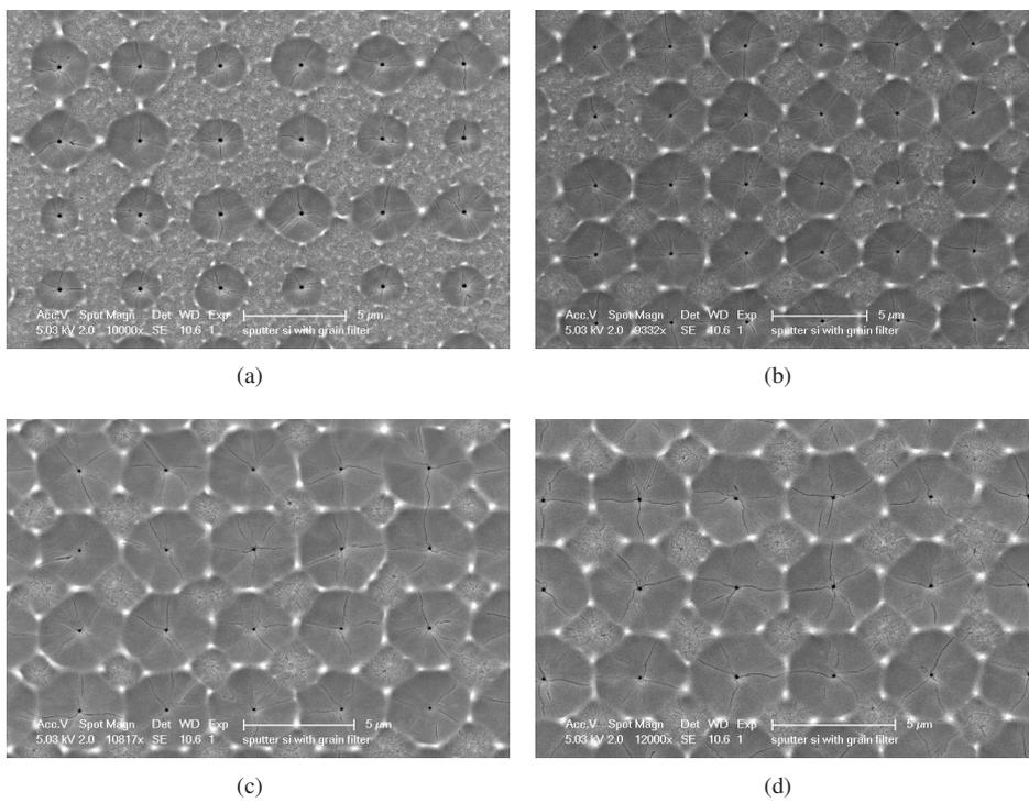
Figure 6.12: SEM images of grains grown from a 250 nm thick  $\alpha$ -Si film crystallized at (a) 775 mJ/cm<sup>2</sup>; (b) 825 mJ/cm<sup>2</sup>; (c) 875 mJ/cm<sup>2</sup>; (d) 900 mJ/cm<sup>2</sup>.
