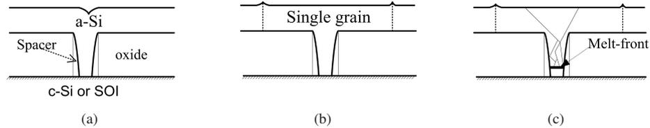
Figure 3.5: Schematic explanation of the effects of melt depth on the morphology of grains: (a) cross section of the experimental configuration; (b) melt front reaching the  $\alpha$ -Si/c-Si interface, resulting in a single grain; (c) melt front not reaching the interface, resulting in multiple fine grains.
