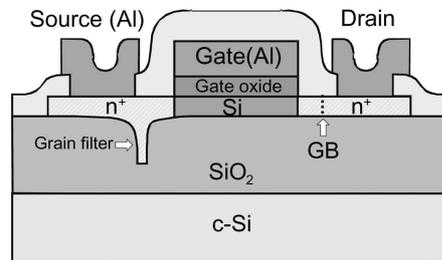
Figure 2.3: Schematic representation of the cross-sectional view of a SG-TFT inside a location-controlled grain, fabricated with the  $\mu$ -Czochralski process. GB denotes the grain boundary. The channel region is free of grain boundaries.
