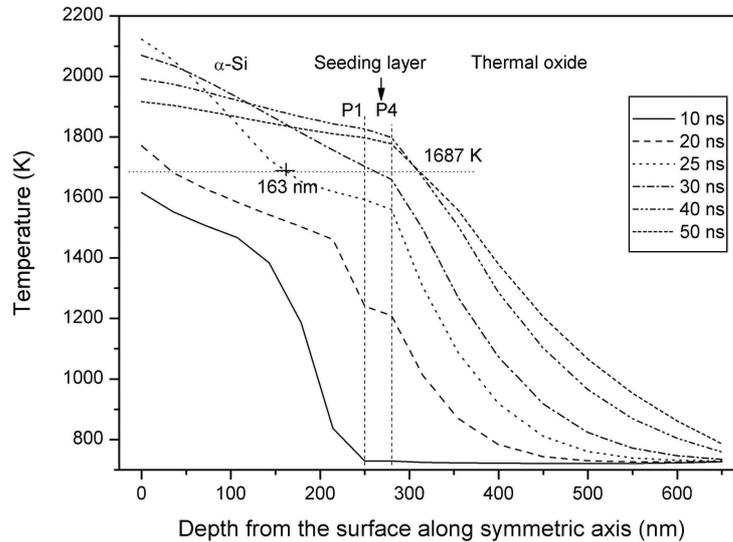
Figure 5.5: Path plots along the symmetry axis through the  $\alpha$ -Si layer, seeding layer, and thermal oxide layer. The origin is at the surface of  $\alpha$ -Si. The region between P1 and P4 (denoted by two dashed lines) is the seeding layer.
