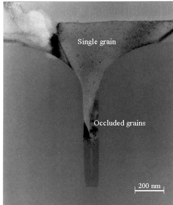
Figure 1.2: Cross-section transmission electron microscopic (TEM) image of the grain filter of diameter  $d = 1.0 \mu\text{m}$ , at an energy density of  $1250 \text{ mJ/cm}^2$ .
