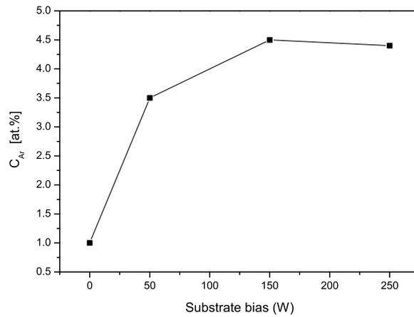
Figure 6.2: Content of trapped Ar in an  $\alpha$ -Si film as a function of the substrate bias (wafers No. A1, B5, B6, B7).  $C_{Ar}$  is analyzed by RBS.
