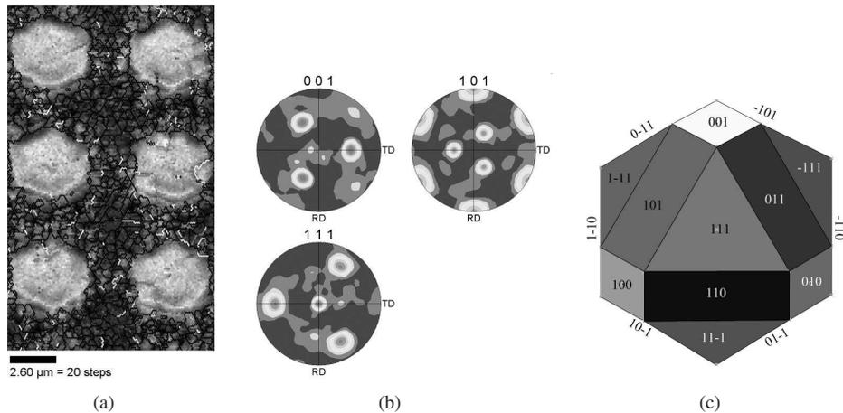
Figure 3.16: Individual grains grown from (111)-oriented seeds with a wet soft-landing step, substrate heating up to 450°C, and a laser fluence of 1400 mJ/cm<sup>2</sup>. (a) EBSD image-quality map overlaid with CSL grain-boundary-component map, clearly showing that grains are hexagonal shaped. (b) Pole figure of the grains. (c) Schematic drawing of the crystal shape of grains grown with normal direction  $\langle 111\rangle$  and transmission direction  $\langle 2\bar{1}\bar{1}\rangle$ .
