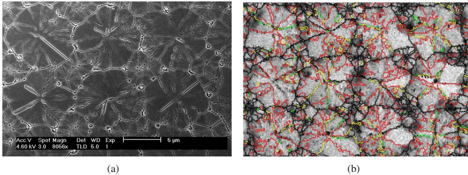
Figure 3.2: (a) SEM image of crystallized location-controlled silicon grains. The thickness of the capping layer ( $T_{CL}$ ) is 200 nm, while the energy density of the laser pulse ( $E_l$ ) is 1400 mJ/cm<sup>2</sup>. (b) Grain-boundary-component map overlaid with an image quality map obtained from EBSD analysis. Black lines indicate random grain boundaries, while yellow and green lines show  $\Sigma 3$ ,  $\Sigma 9$ , and  $\Sigma 27$  boundaries, respectively.
