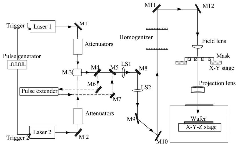
Figure 2.2: Schematic representation of the Exitech M8000V laser system. The removable mirrors M4 and M5 are used to direct the pair of beams into and out of the pulse-duration extender when required.
