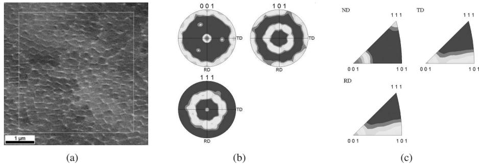
Figure 4.4: Texture of poly-Si grains, crystallized at  $280 \text{ mJ/cm}^2$  after 500 shots. (a) SEM image of poly-Si; the rectangle shows the mapping area. The grain boundaries are facets, forming zigzag lines. (b) Pole figure of the mapped area. (c) Inverse pole figures in the ND, RD, and TD.
