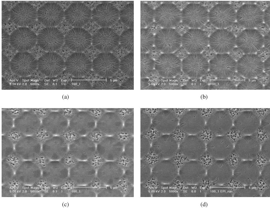
Figure 3.4: Grains grown from (100)-oriented wafers with wet soft-landing (method (i)); the step height is 450 nm and the substrate is heated up to 450°C with a laser fluence  $E_1$  of (a) 900 mJ/cm<sup>2</sup>, (b) 1100 mJ/cm<sup>2</sup>, (c) 1300 mJ/cm<sup>2</sup>, (d) 1400 mJ/cm<sup>2</sup>.
