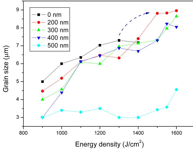
Figure A. 1: Variations of the grain size with the energy density ( $E_1$ ) for several values of  $T_{CL}$ . Because of ablation, an  $\alpha$ -Si film without a CL cannot withstand an energy density in excess of 1400 mJ/cm<sup>2</sup> – however,  $E_1$  can be higher, up to 1600 mJ/cm<sup>2</sup> for capped samples.
