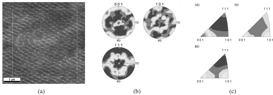
Figure 4.3: Texture of poly-Si grains, crystallized at  $260 \text{ mJ/cm}^2$  after 500 shots. (a) SEM image of poly-Si; the rectangle shows the mapping area. (b)  $\langle 100 \rangle$ ,  $\langle 111 \rangle$  and  $\langle 110 \rangle$  pole figures of the mapped area. (c) Inverse-pole figures in the normal direction (ND), rolling direction (RD), and transverse direction (TD).
