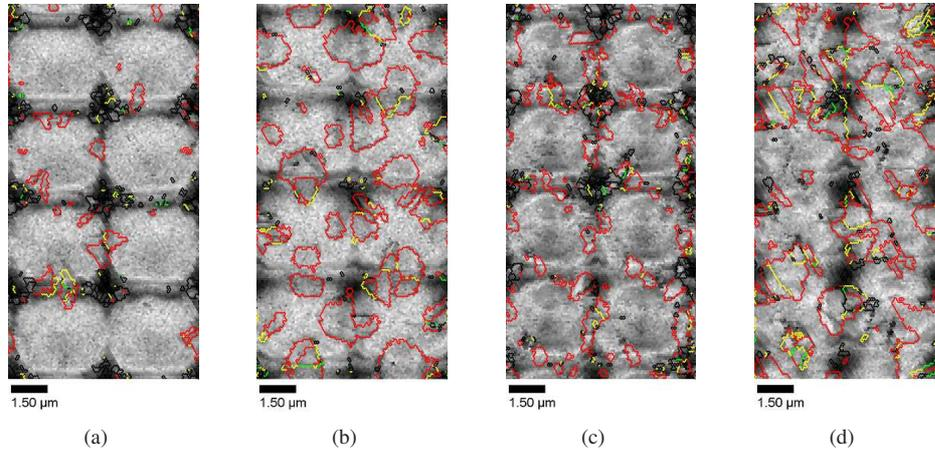
Figure 3.10: Grain-boundary maps of grains grown from (100)- [(a), (b)] and (110)- [(c), (d)] oriented wafers with method (ii). Samples are crystallized at  $1200 \text{ mJ/cm}^2$  and  $450^\circ\text{C}$ ; the step height is  $450 \text{ nm}$  [(a) and (c)] or  $750 \text{ nm}$  [(b) and (d)].
