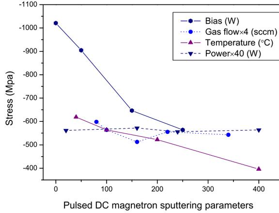
Figure 6.1: Effect of the parameters of pulsed DC magnetron sputtering on the residual stress in the  $\alpha$ -Si film.
