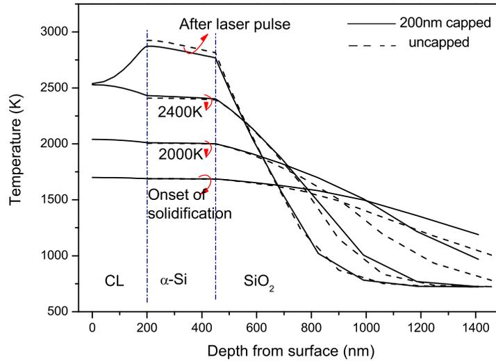
Figure A. 3: Temperature profiles of  $\alpha$ -Si films with and without a capping layer for the same input  $E_{\text{eff}}$ . Dotted line: without capping layer at  $1067 \text{ mJ/cm}^2$ ; straight lines: 200 nm thick capping layer at  $1400 \text{ mJ/cm}^2$ .
