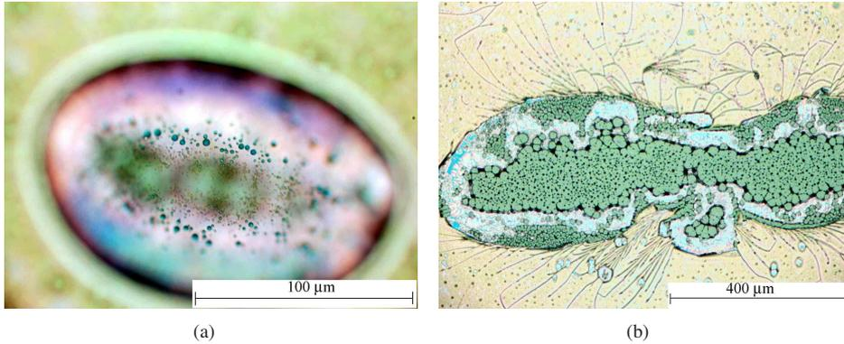
Figure A. 8: Agglomeration of  $\alpha$ -Si films with a 400 nm thick capping layer at (a)  $E_1 = 1941 \text{ mJ/cm}^2$ ; (b)  $E_1 = 2046 \text{ mJ/cm}^2$ .
