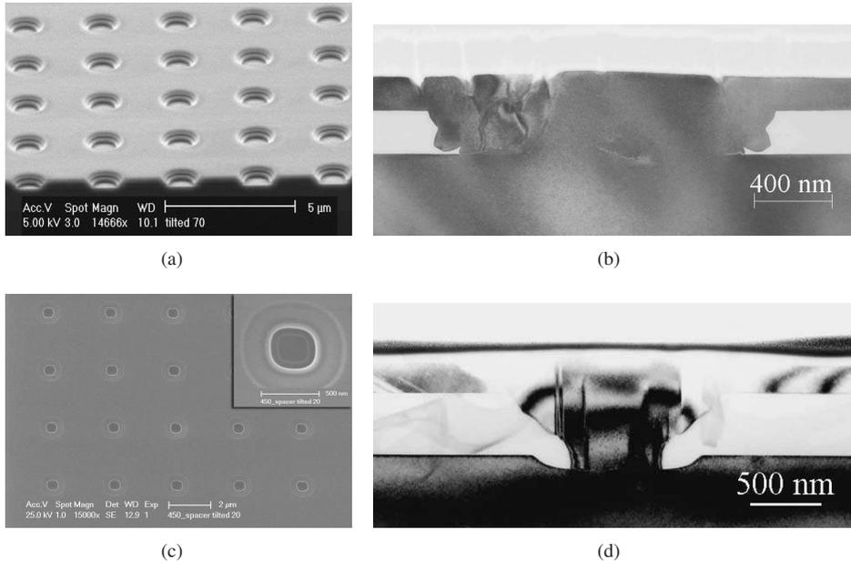
Figure 3.11: Cross-sectional SEM images of holes produced with (a) a wet soft-landing step; and (c) a dry soft-landing step. Sample (a) was tilted at  $70^\circ$ , while sample (c) at  $20^\circ$ . Cross-sectional TEM images of (b) grains grown from a (100)-oriented wafer with a wet soft-landing step; and (d) grains grown from a (110)-oriented wafer with a dry soft-landing step, crystallized at  $1200 \text{ mJ/cm}^2$  with a step height of 450 nm.
