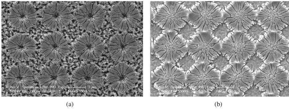
Figure 3.8: Grains grown from (100)-oriented bulk-Si wafers with a wet soft-landing step (method (i)); the step height is 450 nm and the laser fluence used in room-temperature excimer-laser crystallization is (a) 900 mJ/cm<sup>2</sup>, (b) 1400 mJ/cm<sup>2</sup>.
