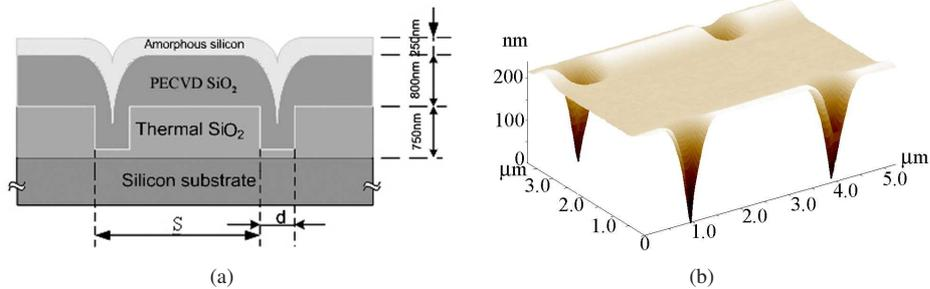
Figure 1.1: The structure of the grain filter. (a) Parameters of the grain filter:  $d$  is the diameter of the hole in the thermal SiO<sub>2</sub> layer, and  $S$  is the spacing of grain filters. (b) The cavity matrix of grain filters with a hole diameter of 1.0 μm before  $\alpha$ -Si deposition.
