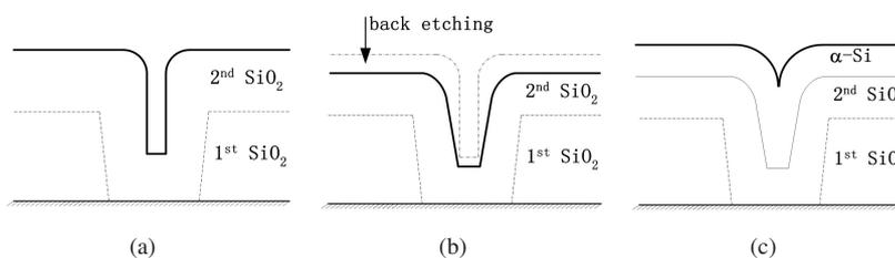
Figure 6.10: Modified grain filter obtained by back-etching the 2nd TEOS layer. (a) Normal grain filter; (b) back-etching of the 2nd TEOS layer; (c) sputtering  $\alpha$ -Si on the modified grain filter.
