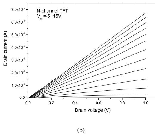
Figure 6.15: Transfer characteristics (a) and output characteristics (b) of single-grain TFTs fabricated with gate-oxide deposition at  $80^\circ\text{C}$ . The subthreshold slope is 0.49 V/dec., while the maximum electron field-effect mobility is  $290 \text{ cm}^2/\text{V}\cdot\text{sec}$ .
