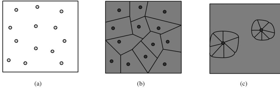
Figure 6.8: Schematic representation of the growth mechanism of an  $\alpha$ -Si precursor after laser irradiation. (a) As-deposited  $\alpha$ -Si; round dots are randomly distributed fine crystals. (b) Collided grains at a low energy density of laser pulse. (c) Large grains at a higher energy density of laser pulse.
