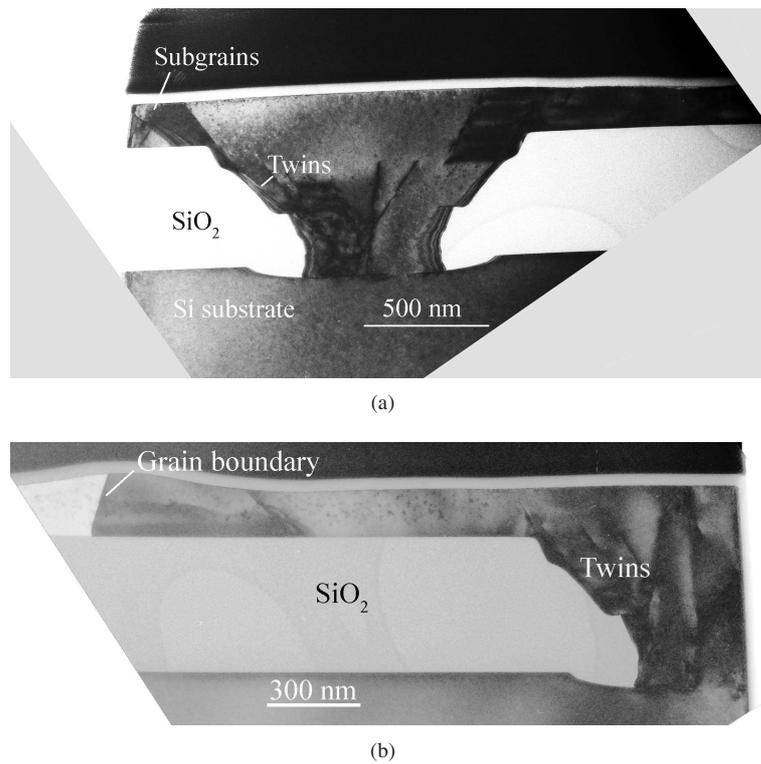
Figure 3.20: Cross-sectional TEM images of grains grown from  $\langle 100 \rangle$ -oriented seeds with a dry soft-landing step (etching method (ii)), with substrate heating up to  $450^\circ\text{C}$ . (a) Epitaxial growth and vertical growth from the seed. (b) Lateral growth along the Si/SiO<sub>2</sub> interface.
