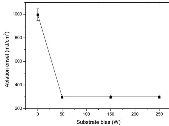
Figure 6.3: Influence of the substrate bias on ablation during excimer-laser crystallization (wafers No. A1, B5, B6, B7).
