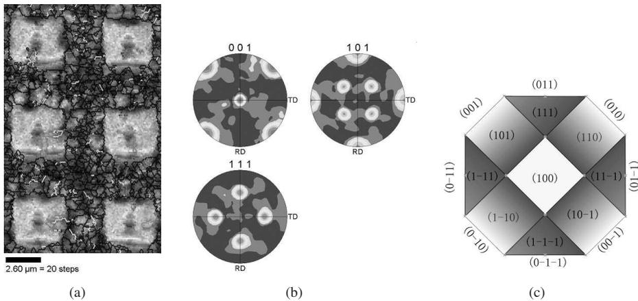
Figure 3.15: Individual grains grown from (100)-oriented seeds with a wet soft-landing step, substrate heating up to 450°C, and a laser fluence of 1400 mJ/cm<sup>2</sup>. (a) EBSD image-quality map overlaid with CSL grain-boundary-component map, clearly showing that grains are square-shaped. (b) Pole figure of the grains. (c) Schematic drawing of the crystal shape of grains grown with normal direction  $\langle 100 \rangle$  and transmission direction  $\langle 1\bar{1}0 \rangle$ .
