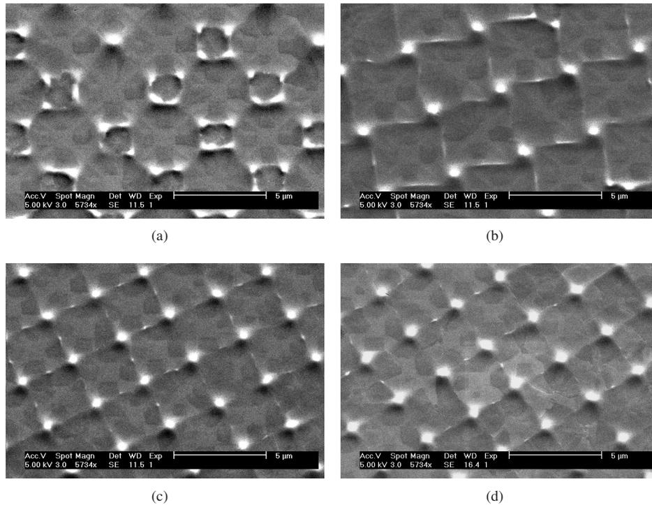
Figure 3.22: SEM images of grains grown from (100)-oriented seeds with a dry soft-landing step [crystallization at  $1300 \text{ mJ/cm}^2$  and  $450^\circ\text{C}$ ], with (a) [100]-, (b) [210]-, (c) [310]-, and (d) [510]-oriented holes. Secondary subgrains (dark regions inside the grains) are generated at identical positions for holes of different orientation.
