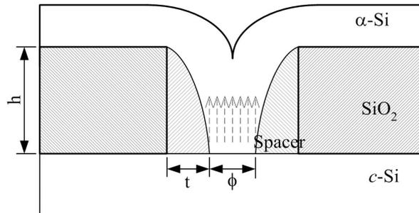
Figure 3.3: Schematic cross-sectional view of the selective epitaxial growth of single-crystalline grains through a SiO<sub>2</sub> window with silicon wafer as seed. The step height  $h$  is either 450, 600, or 750 nm;  $t$  is the spacer offset, and  $\phi$  is the diameter of the opening to the seeds at the bottom of the grain filter. Dashed arrows indicate the vertical growth from the seed after excimer-laser irradiation.
