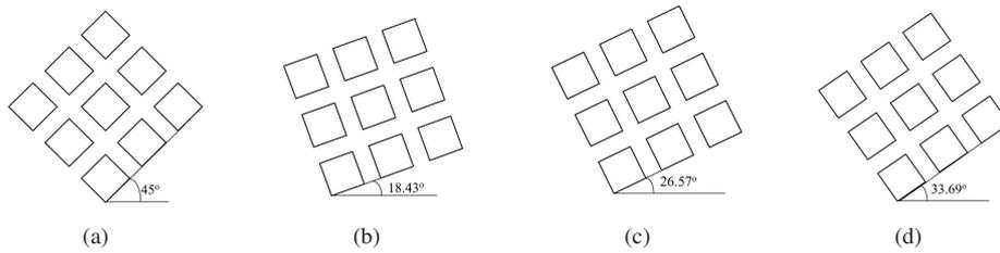
Figure 3.21: Schematic drawing of the orientation of holes opened in the first TEOS layer, with respect to the orientation of the underlying (100)-oriented wafer. (a) [100]-oriented holes; (b) [210]-oriented holes; (c) [310]-oriented holes; and (d) [510]-oriented holes. Holes are normally along the [110] orientation and the horizontal direction.
