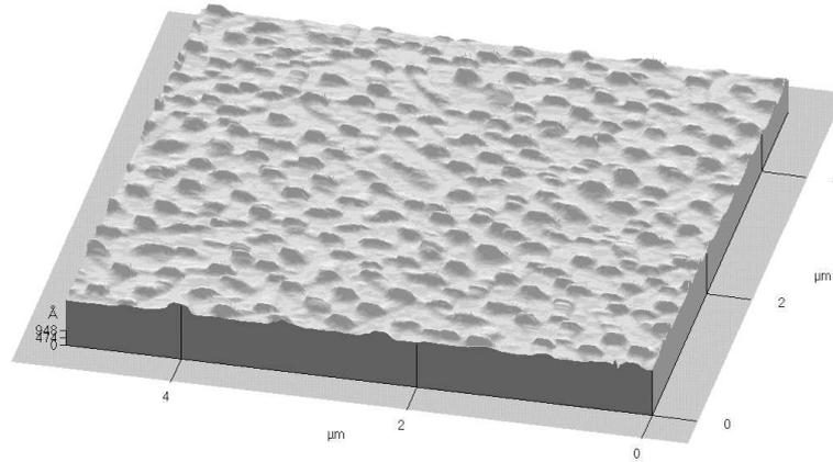
Figure 4.2: AFM image of poly-Si grains crystallized at  $260 \text{ mJ/cm}^2$  after 500 shots.
