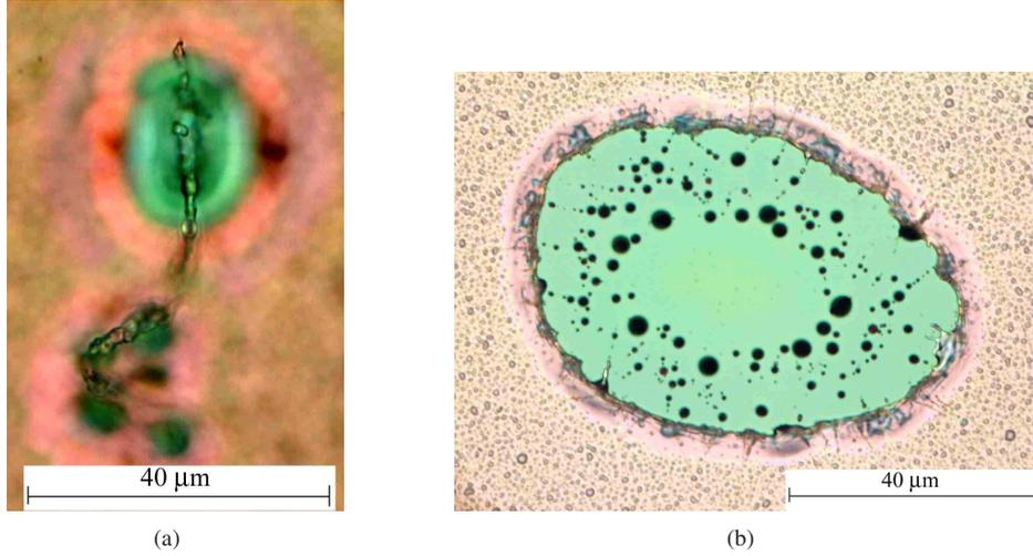
Figure A. 7: Agglomeration of  $\alpha$ -Si films with a 100 nm thick CL at an irradiation energy density of (a) 1441 mJ/cm<sup>2</sup>, (b) 1793 mJ/cm<sup>2</sup>.
