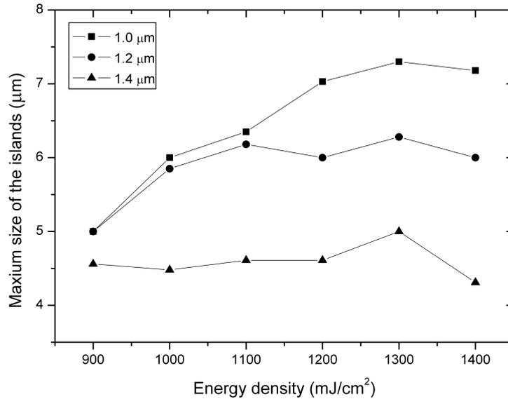
Figure 1.3: The maximum island size as a function of the laser energy density for different diameters  $d$  of the grain filter.
