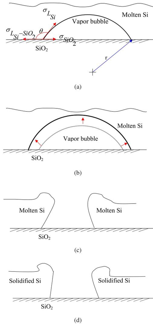
Figure A. 10: Schematic representation of the process of hole formation. (a) Heterogeneous nucleation of the vapor bubble at the  $L_{Si}/S_{SiO_2}$  interface. The contact angle between  $L_{Si}$  and  $S_{SiO_2}$  is larger than  $90^\circ$ . (b) Growth of the vapor bubble. (c) Burst of the vapor bubble. (d) Solidification of the molten Si.
