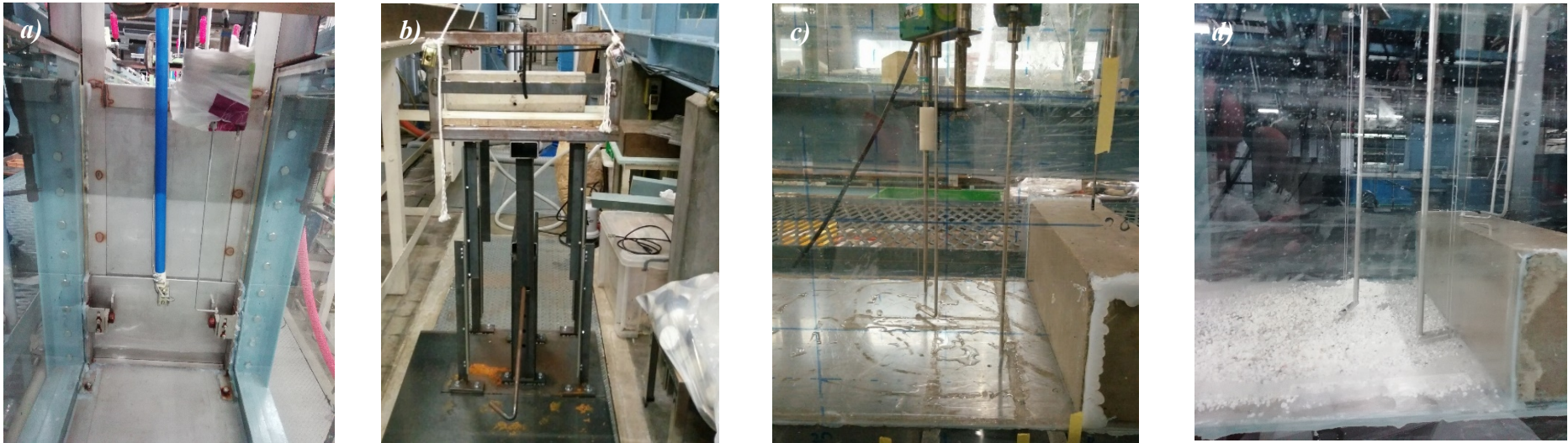
Figure 4. Experimental Apparatus. a) View of the back of the gate. b) Weight system to release the gate. c) wave gauge and velocity meters (smooth flat bed). d) stone flat bed
