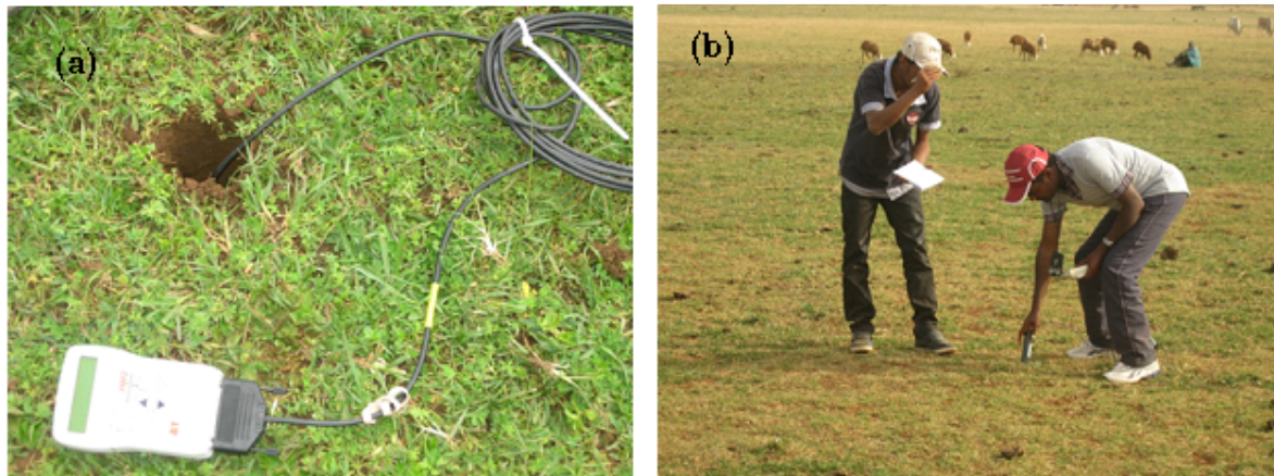
Figure 30 Pictures of in-situ soil moisture observation using Theta Probe ML2x over Sentera grassland (a & b)
