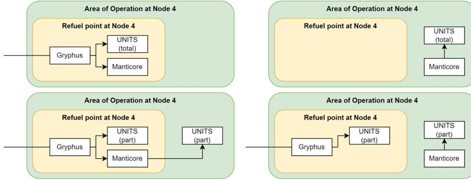
Figure 4.4: Schematic representation of the various deployment options of the Manticore.
