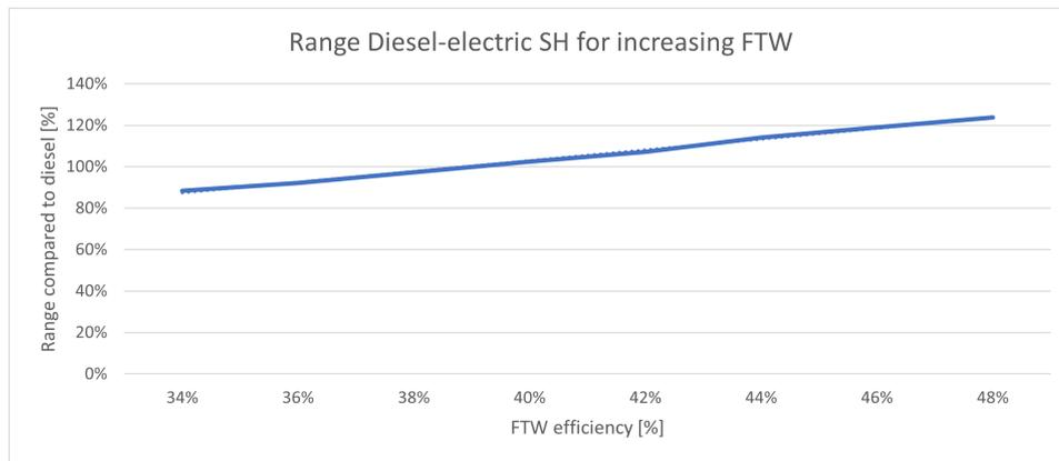
**Figure 5.20:** Impact of increasing FTW efficiency on the average vehicle range for diesel-electric series hybrid
