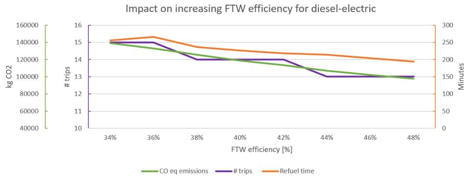
Figure 5.21: Impact of increasing FTW efficiency for diesel-electric series hybrid
