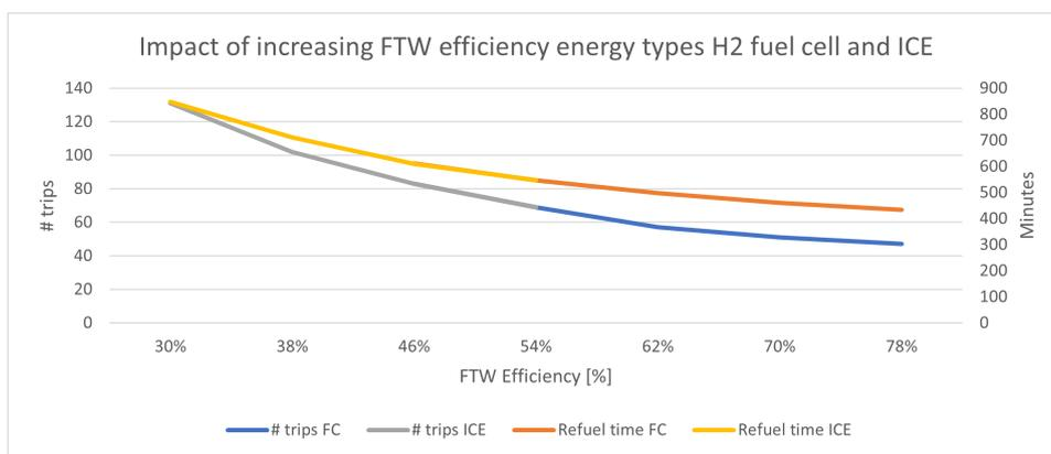
Figure 5.19: Impact of increasing FTW efficiency for energy types H2 fuel cell and ICE
