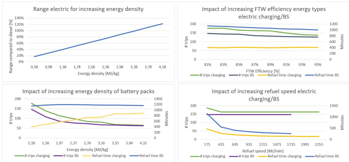
**Figure 5. P3 results for electric battery swap and charging**
