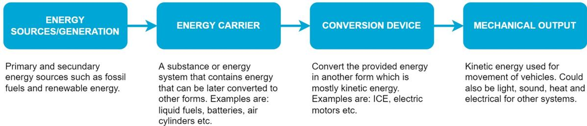
**Figure 2.1:** Components of the energy chain
