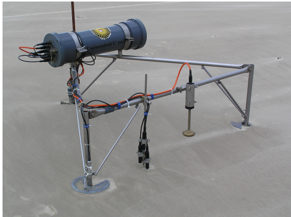
Figure 8-1 Mini tripod including pressure sensor, optical backscatter sensors and an electromagnetic flow meter
