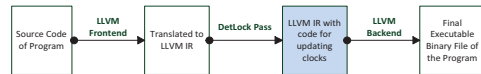
Figure 1: DetLock modifies the LLVM IR code by inserting code for updating logical clocks
