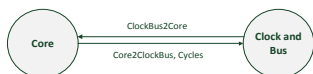
Figure 5. Block diagram of communication between a core process and the clock and bus process
