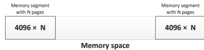
Fig. 3. Memory pages can be grouped into segments to reduce the overhead of memory comparison for error detection
