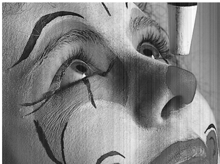
Figure 4-19: Sample image with 3% Gaussian column FPN. DCS is simulated on the left half of the image using a 4x4 unit switching cell
