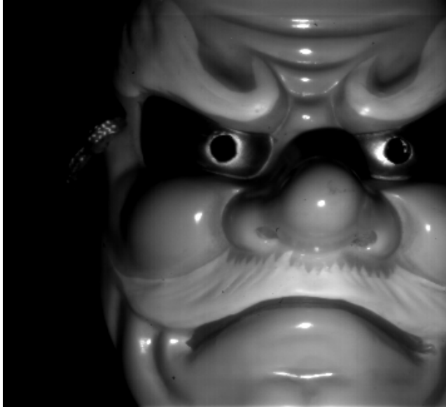
Figure 6-15: Captured image with the ADC in single-slope mode, at 50 frames/second
