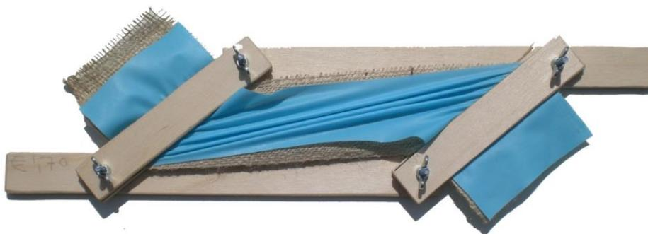
Figure 4: Room temperature shear-deformation of a thin elastic film with burlap for comparison down to 40 degrees.
