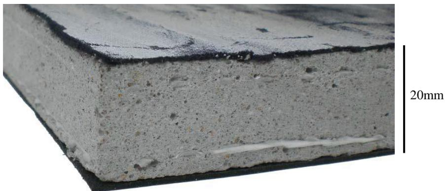
Figure 5: Photo of the physical prototype of the material showing reinforcement, concrete matrix, black elastic layer, and grey-black cloth layer, 20mm thick, 100mm wide, and 200mm long.
