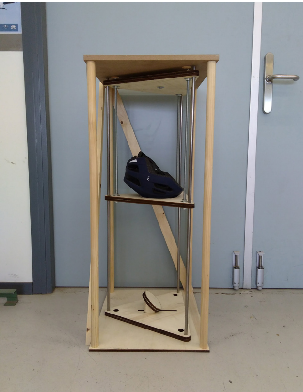
Fig. 6.1.11.: Fabricated drop setup with the 45 degrees anvil installed.
