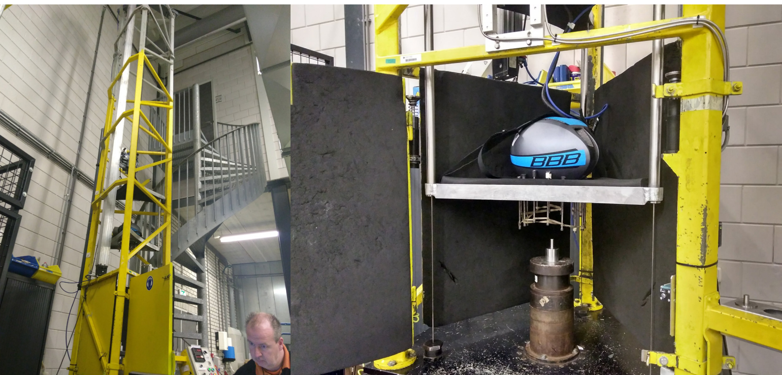
Fig. 6.1.10.: Inspiration for the drop test; a professional drop test setup from TASS International.
