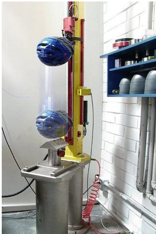
Fig. 3.3.1.: A standard straight drop helmet impact setup.
