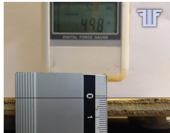
Fig. 6.1.6.: Measuring the amount of compression of prototype A while exercising 49.8N of force.
