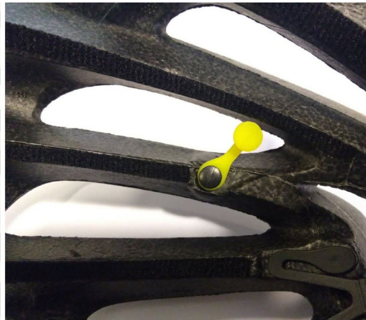
Fig. 6.1.1.: The energy absorbing part of MIPS: four elastomers orientated in a square.
