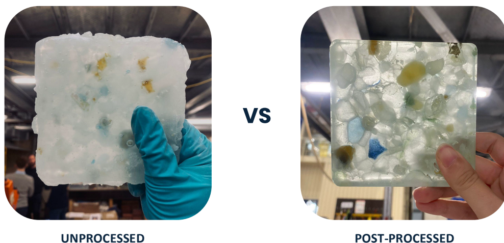
FIGURE 03.30 | The composite sample unprocessed (left), and the composite sample after the post-processing of surface and edge treatments with grinding, polishing, and the addition of UV coating for extra strength (right).
