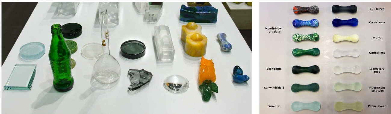
FIGURE 01.21 | Re 3 Glass Project's commercial glass products (left) converted into recycled bone-capsule interlocking elements (right). (Bristogianni et al., 2019)
