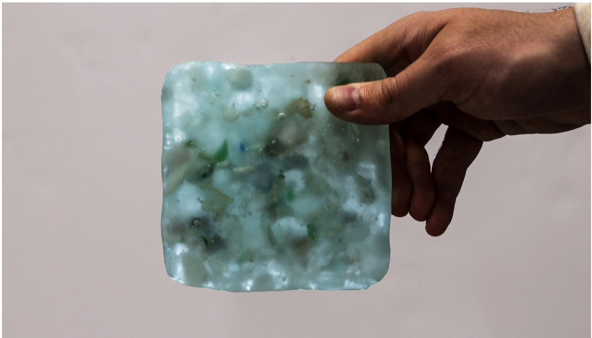
FIGURE 03.23 | The translucent composite tile from recycled glass waste in front of a light source.
