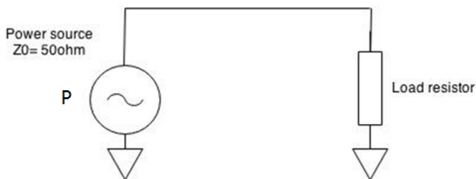
Fig. 2.4 - General schematic of a power source injecting power into an arbitrary load impedance.
