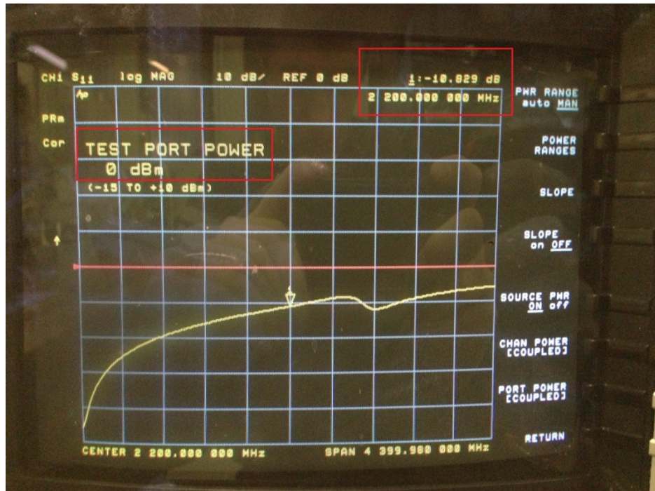
Fig. 6.8 - Return loss of the improved diode power detector when a 0 dbm power level is applied at its input.
