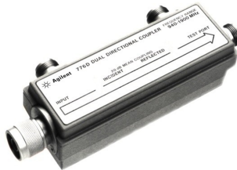
Fig. 3.18 - External directional coupler able to handle large input powers while providing high directivity.
