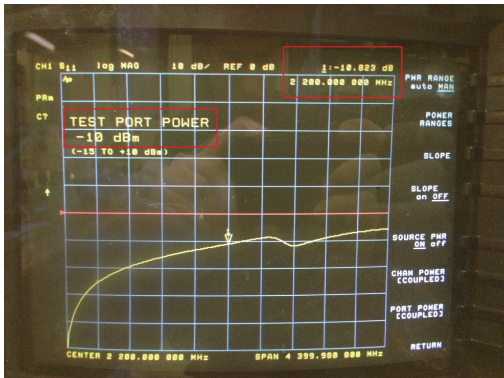
Fig. 6.9 - Return loss of the improved diode power detector when a -10 dbm power level is applied at its input.
