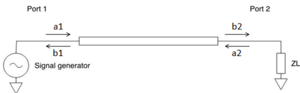
Fig. 2.2 - Forward and reflected “a” and “b” waves at the ports of a transmission line.
