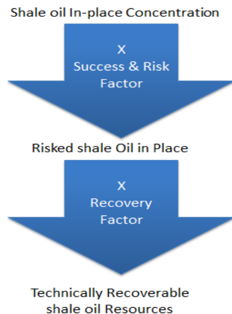
Figure 5: Flowchart of evaluation of potential shale oil formations by the EIA
