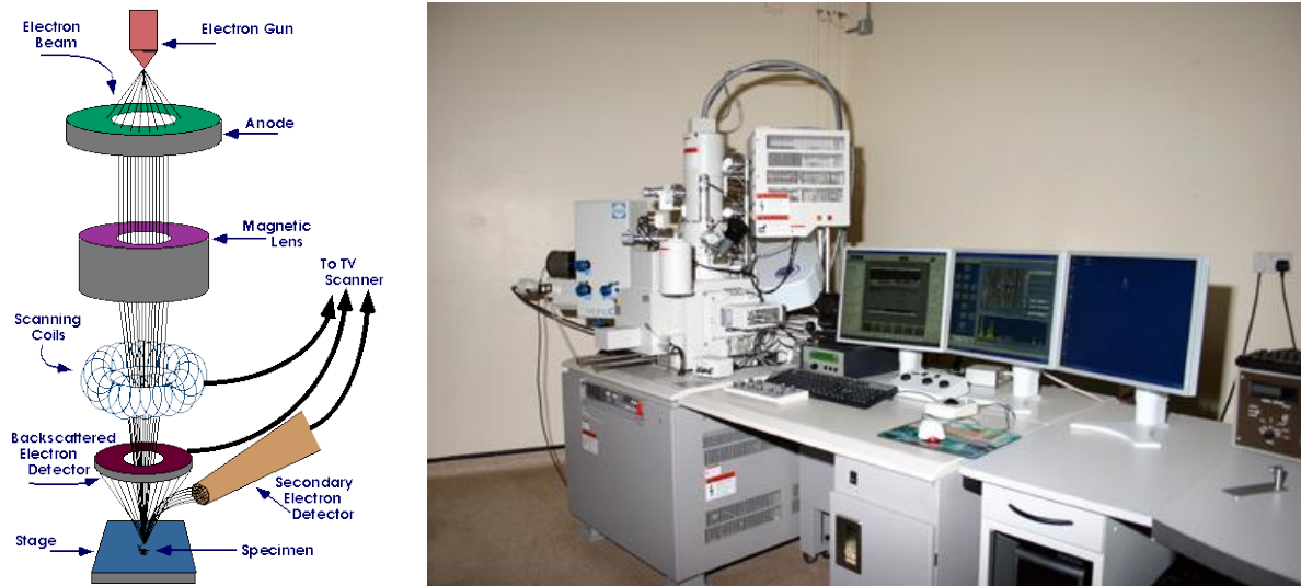
Figure 15: Schematic drawing (Purdue University) of the working principle of a SEM and the used SEM setup at Durham University ( www.dur.ac.uk ).
