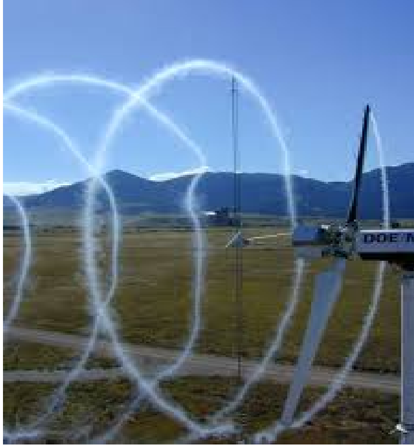
Figure 3.1: Helical structure formed of tip vortices shed from wind turbine [8]
