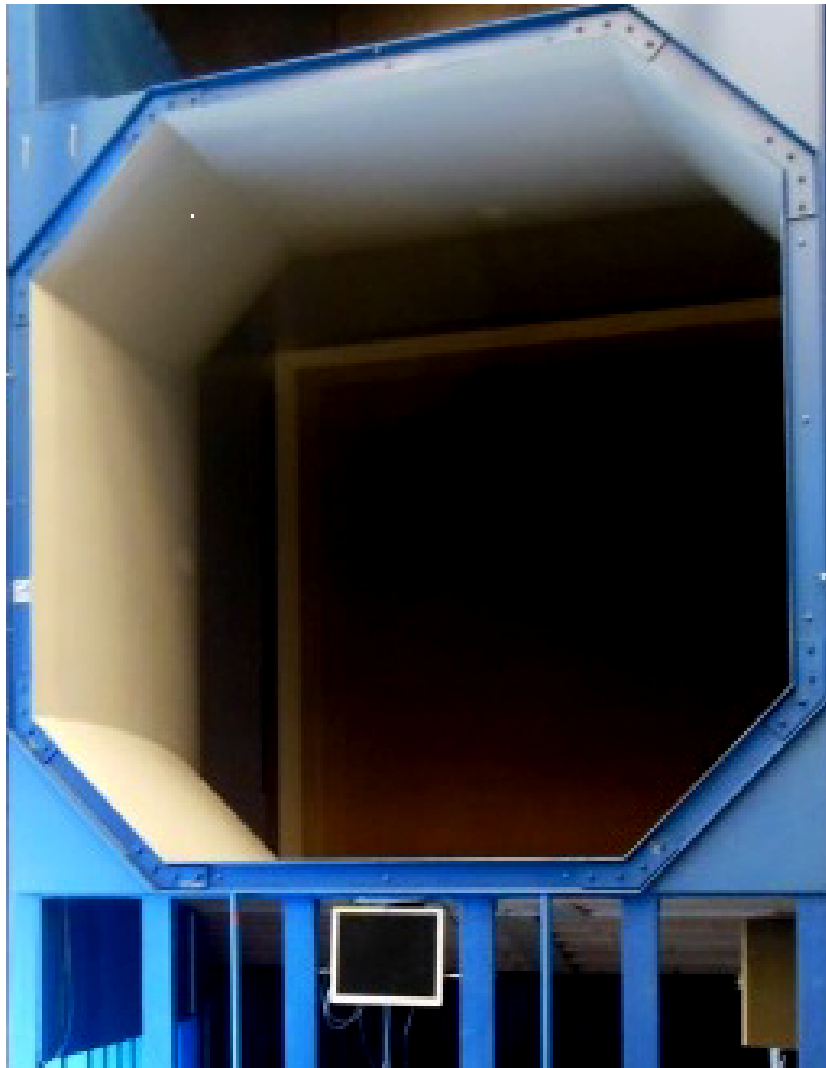
Figure 5.4: Octagonal Nozzle of OJF [1]
