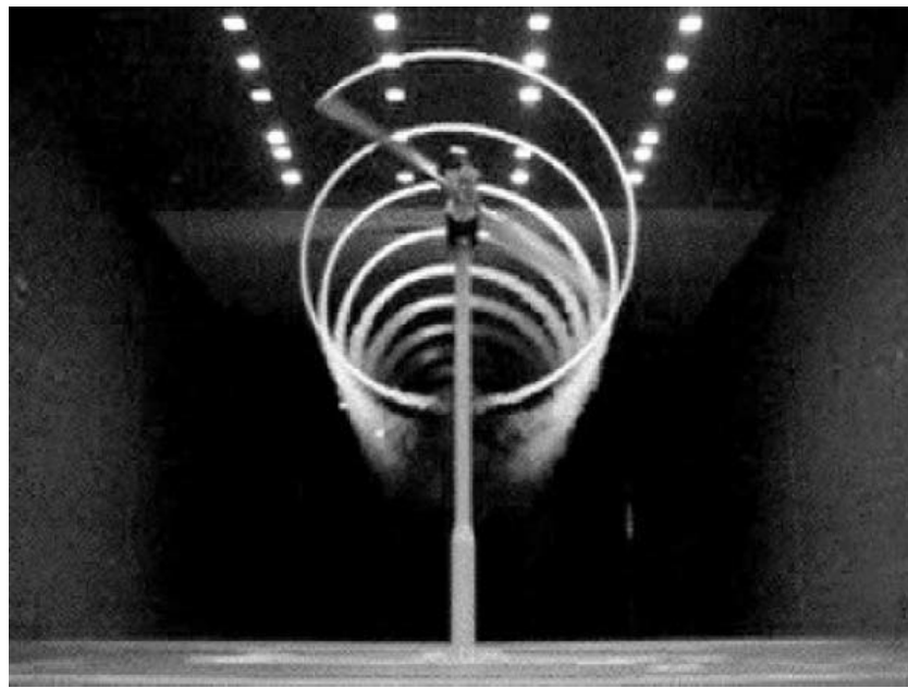
Figure 3.4: Smoke flow visualization showing helical structure of tip vortices for the NREL turbine in the NASA-Ames wind tunnel [11]
