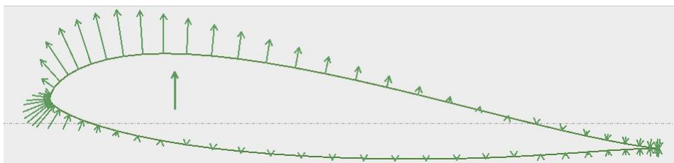
Figure 8.2: Visualisation of pressure distribution around aerofoil at cruise
