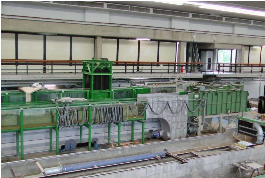
Fig. 3.7: Wave flume and generator
