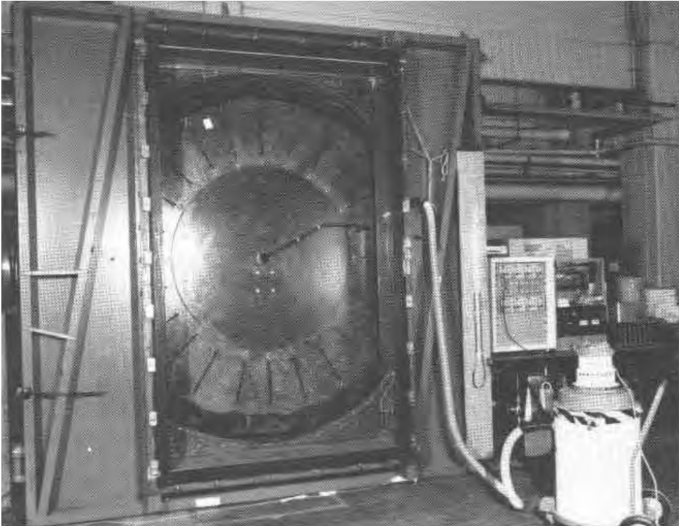
Figure 8.2: Dynamic glass testing rig (Dalglish & Taylor, 1990)
