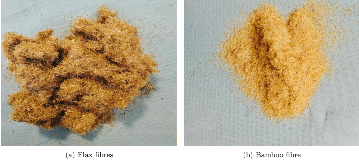
Figure 3.2: Flax (6mm) and Bamboo (5mm) fibres used for BMC Production
