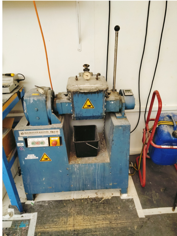
Figure 3.3: Sigma (Z) blade mixer for BMC dough mixing
