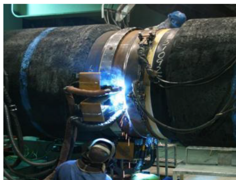
Figure 3: Joint welding system.
