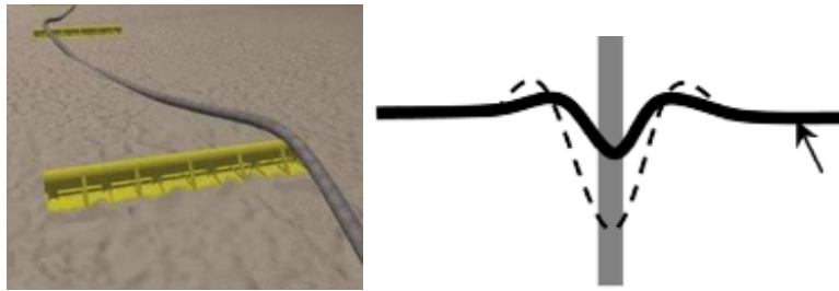
Figure 2.6: Schematic representation of the vertical out-of-straightness method [33].
