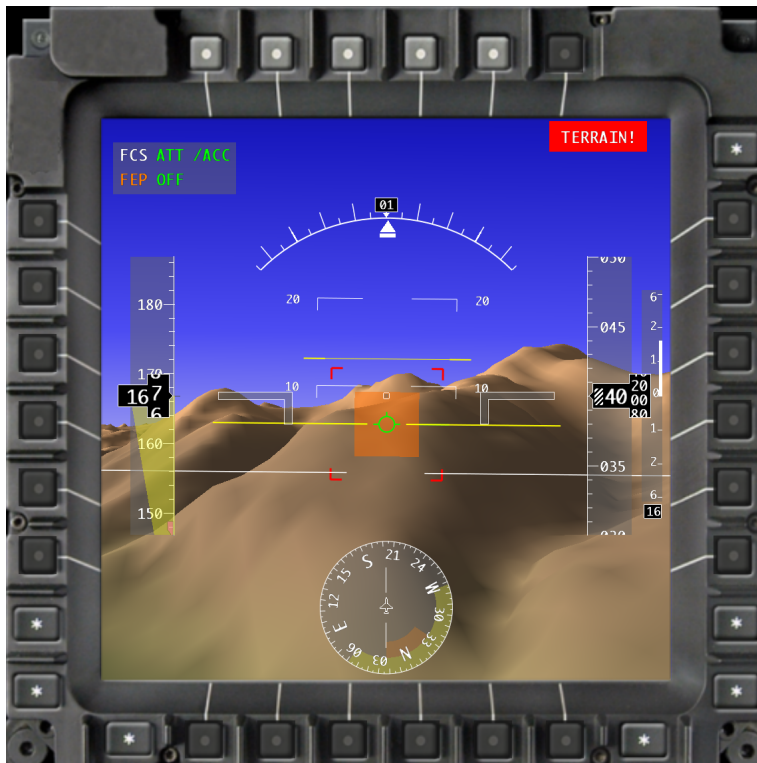
Figure 1.5: The ecological Synthetic Vision Display (SVD)(Borst et al., 2010).
