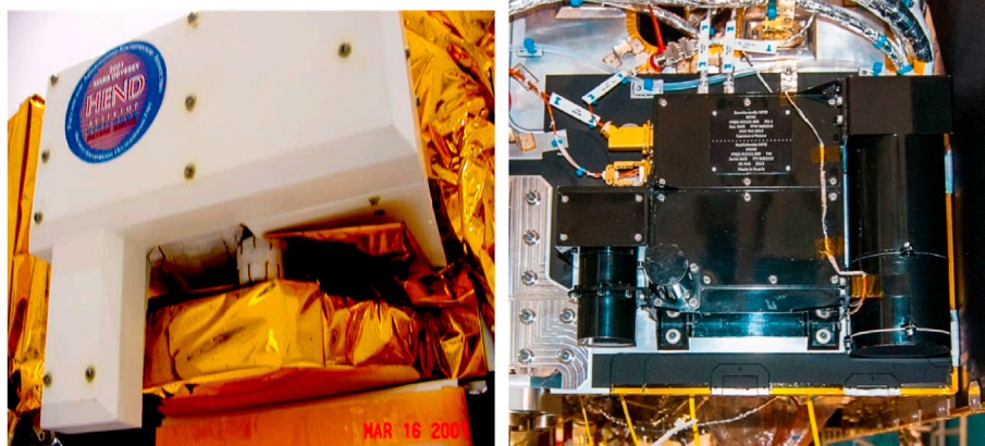
Fig. 2. MGNS instrument (left) and HEND instrument (right) integrated into the ESA BepiColombo Mercury Planetary Orbiter and NASA Mars Odyssey flight spacecraft, respectively.
