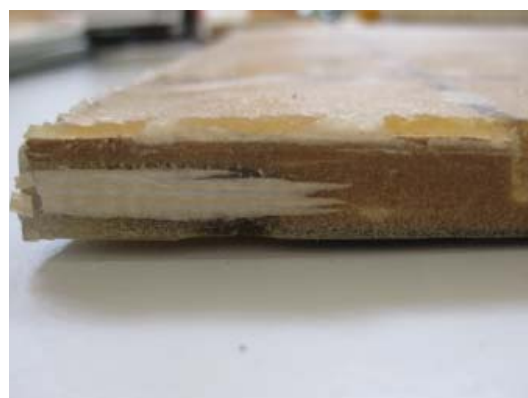
fig.7.21 rigid carved formwork enclosed with a thin PU layer
