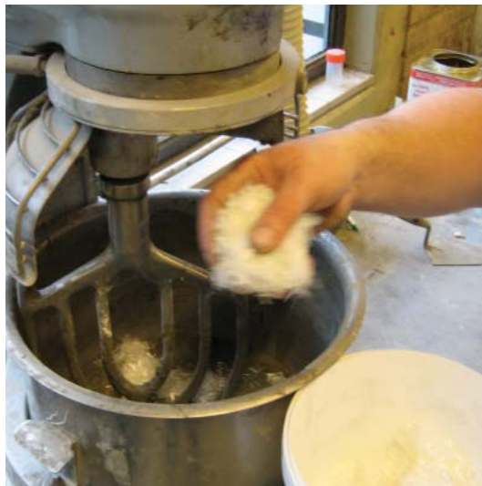
fig.5.1 mixing of ECC concrete
