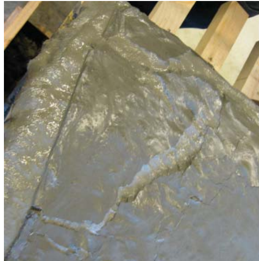
fig.5.7 composition 2; profile sagging
