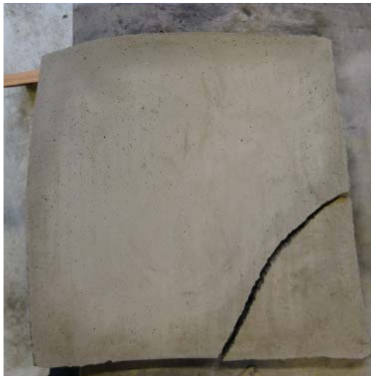
fig.5.6 corner failure in hardened composition1
