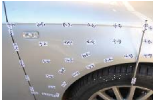
fig.6.16 example of Rhinophoto. The green dots represent the according marks on the actual surface.
