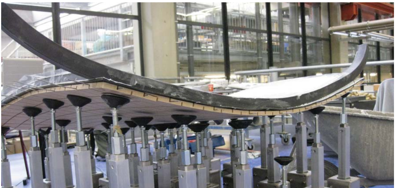
fig.7.16 formwork D in deformed state; several actuators to do not touch the formwork
