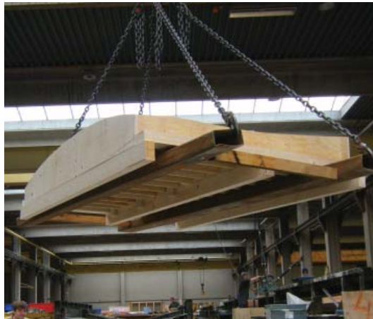
fig.8.1 mould of mock-up1 at Hurks Beton in Veldhoven
