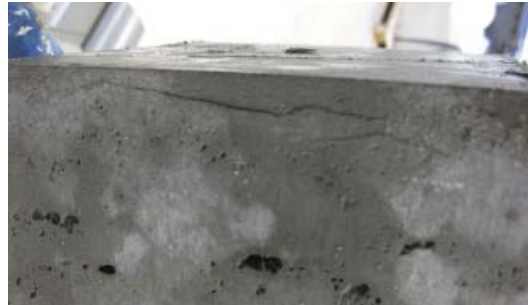
fig.5.12 surface cracks appear at f_c
