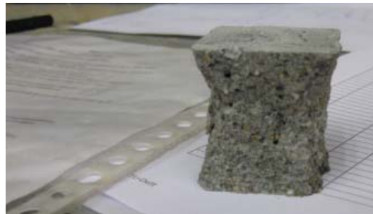
fig.5.13 typical failure of traditional concrete under compression.
