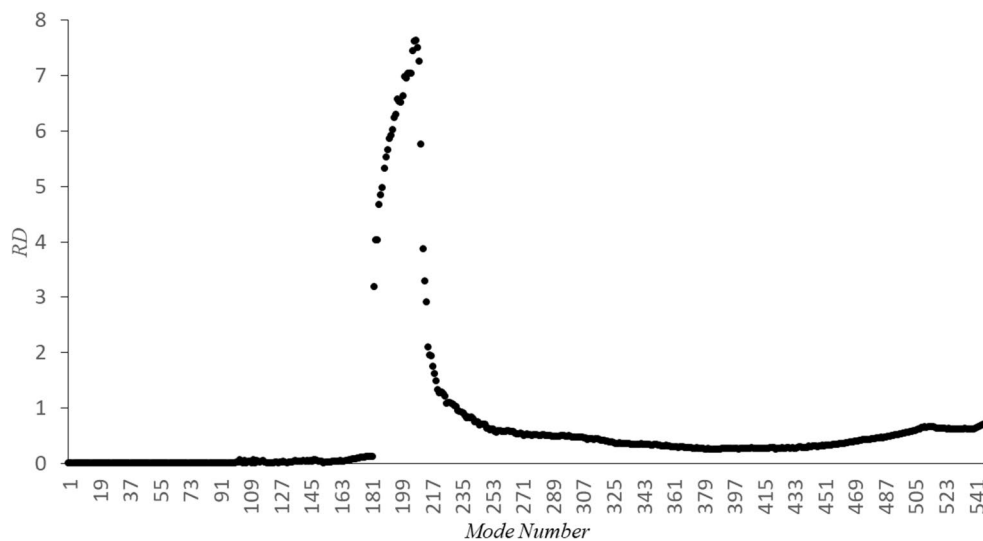
Fig. 4 Relative difference between full models with functions of \theta ranging from 1 to 30 and from 4 to 30, Eqs. (22) and (23); 7 functions of \xi ; CC VSCL thin circular cylindrical shell, properties in Tables 1 and 2
