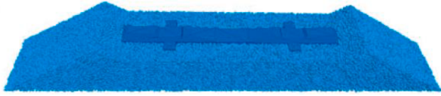
Fig. 2. DEM model of a single sleeper(wing-shape) section [8].
