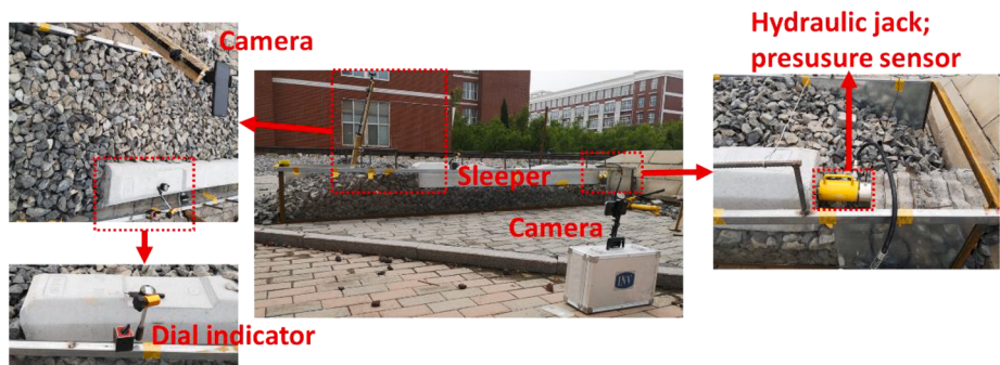
Fig. 15. PIV setting on lateral resistance test [34].
