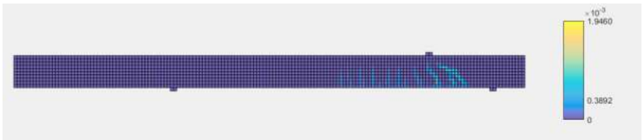
Figure 4. 25 Major principal strain over Finite element mesh at load step 1(0.5mm) for specimen2
