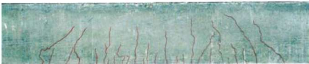
Figure 1. 13 Crack pattern after load step 6 [12]
