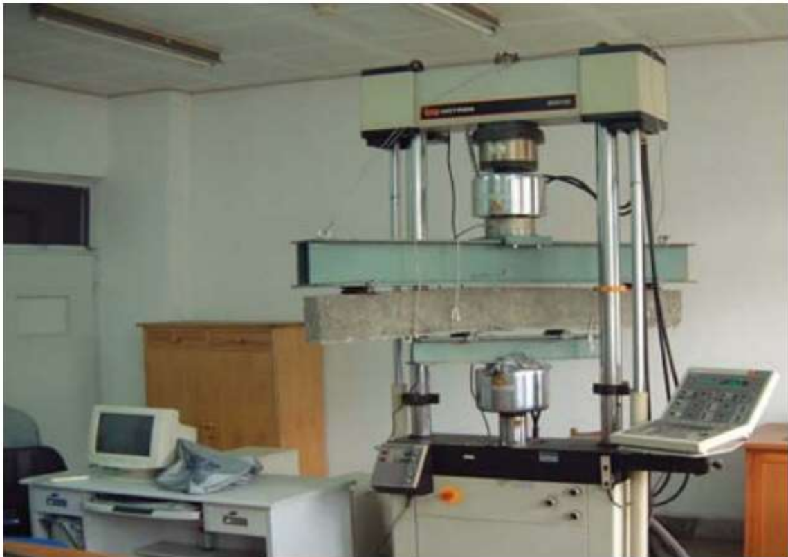
Figure 1. 12 Experimental setup of three-point bending test [12]
