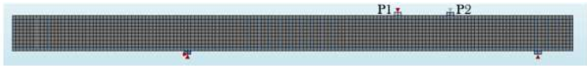
Figure 4. 38 Finite element mesh for phased analysis (Specimen1)
