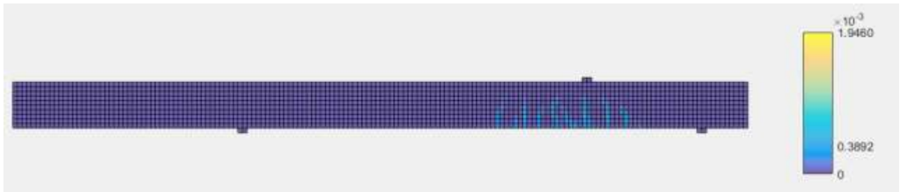
Figure 4. 24 Major Principal strain over Finite element mesh at load step 1(0.5mm) for specimen1
