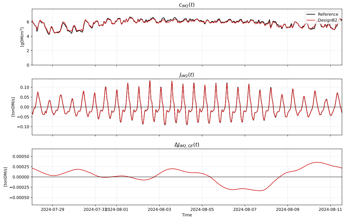
Figure D.10: Temporal variability of IM2 concentration ( c_{IM2} ), advective flux ( J_{IM2} ), and Godin-filtered flux difference ( \Delta J_{IM2,GF} ) between Design B2 and the Reference scenario.
