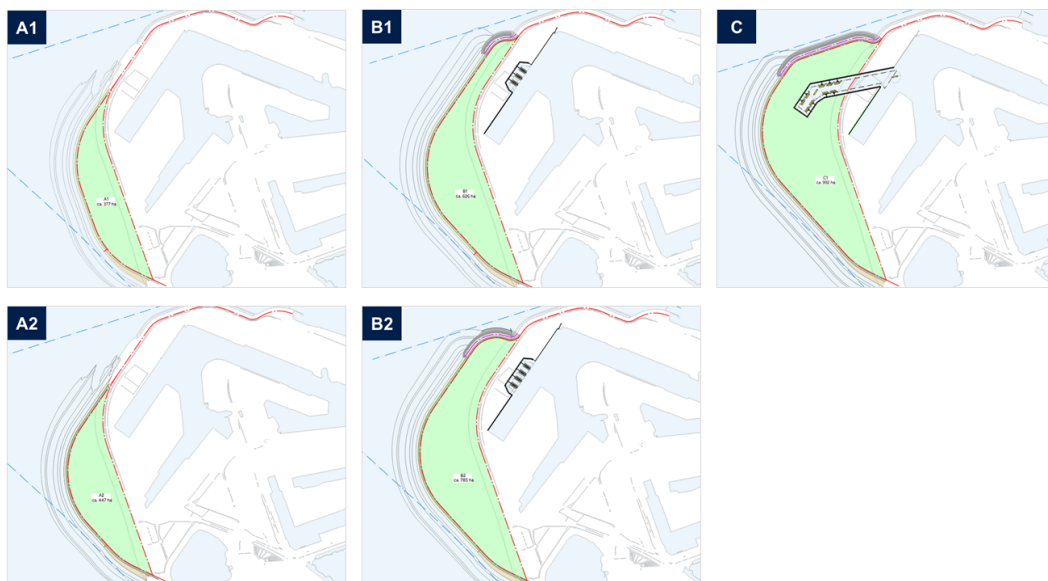
Figure 1.3: Map of the seaward side of Maasvlakte showing the proposed SPE design alternatives A1, A2, B1, B2, and C. The green areas indicate the spatial footprint of each expansion geometry (NOVEX 2025).
