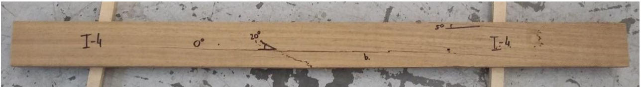
Figure 93: Failure of specimen I-4 (front side).
