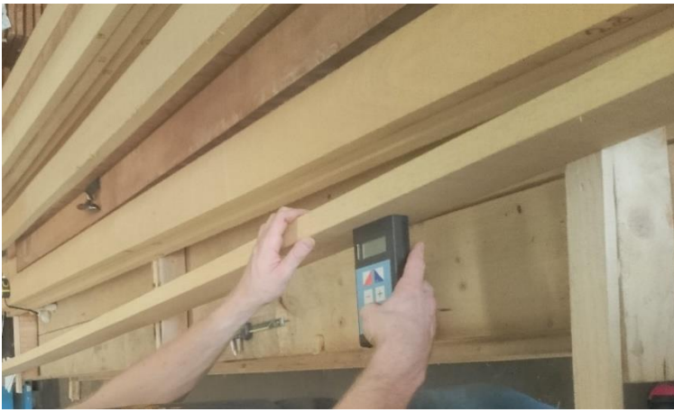
Figure 55: Estimating the moisture content of batch III.
