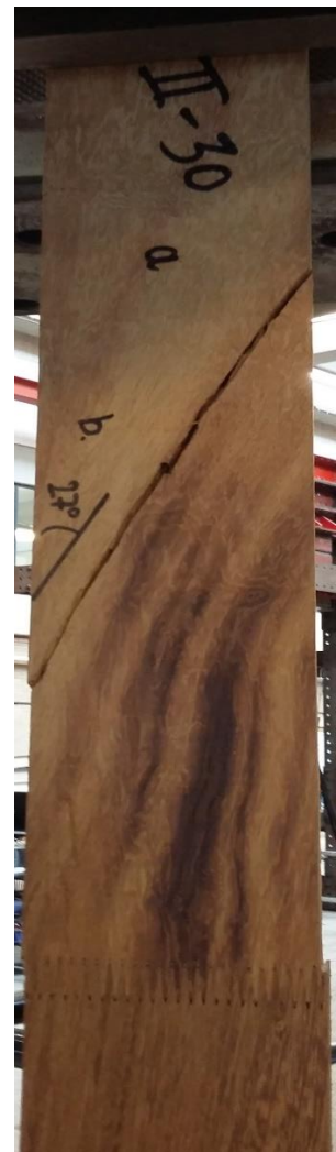
Figure 70: Wood failure (II-30).
