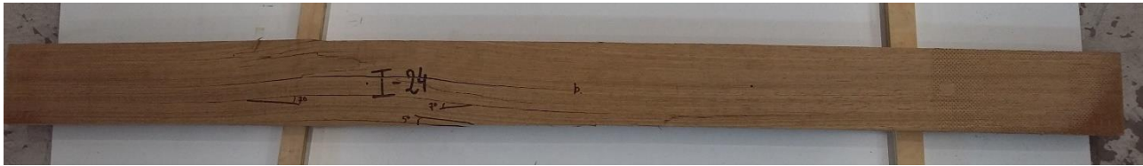
Figure 131: Failure of specimen I-24 (front side).
