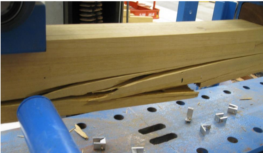
Figure 218: Failure of specimen IV-10 (crack detail).
