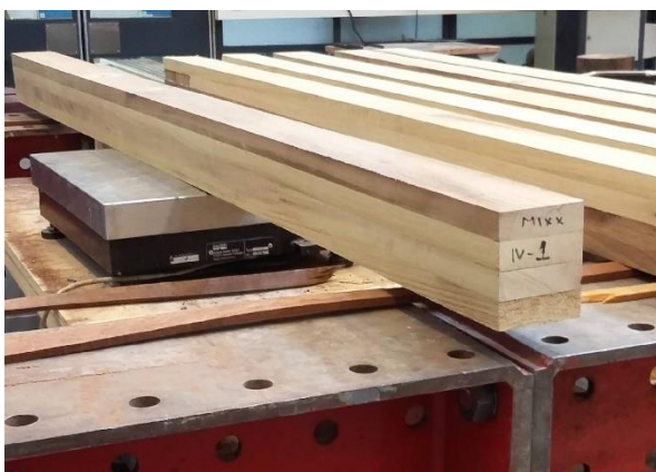
Figure 50: (Heavy) balance, used to weigh specimens of batch I, II and IV.
