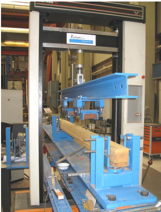
Figure 61: Four point bending test setup (reality).
