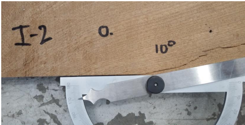
Figure 58: Measuring the angle at which failure occurred.
