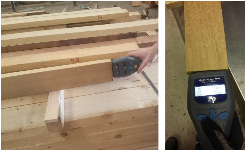
Figure 54: Timber grader handheld: initiating stress wave and measuring vibrations.
