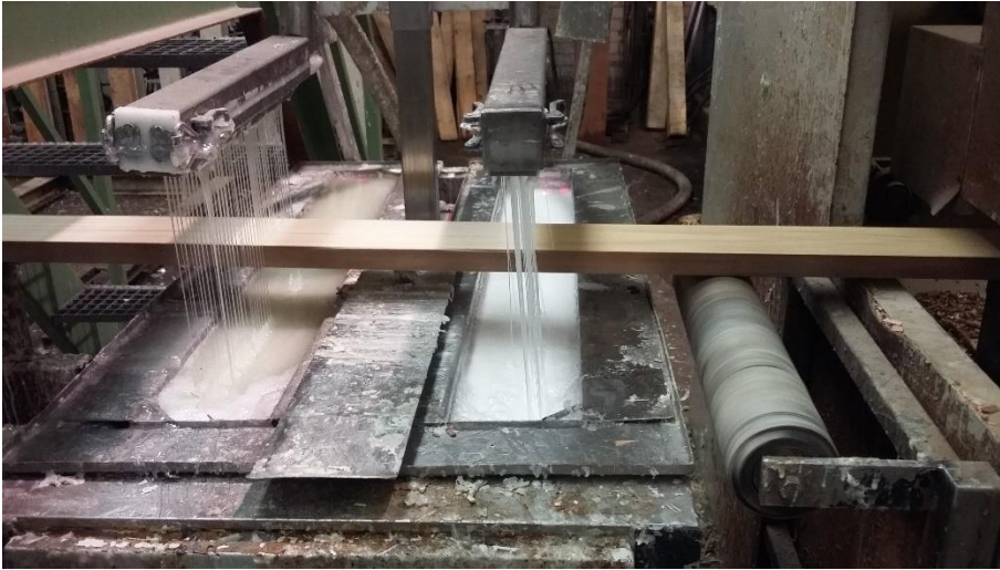
Figure 38: Gluing of the lamellas.
