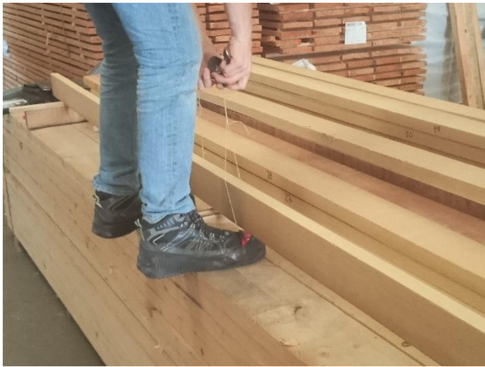
Figure 49: Mass measurement of batch III specimen.
