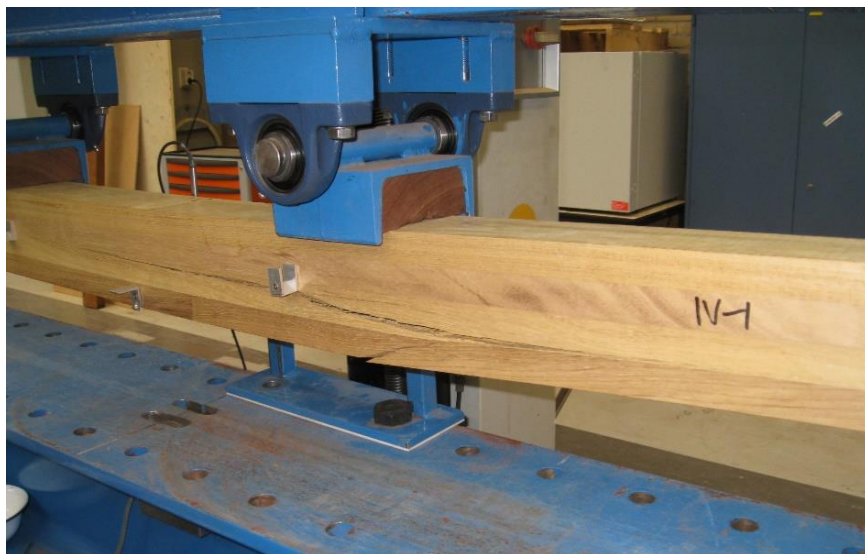
Figure 199: Failure of specimen IV-1.
