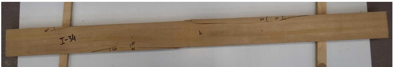
Figure 151: Failure of specimen I-34 (front side).
