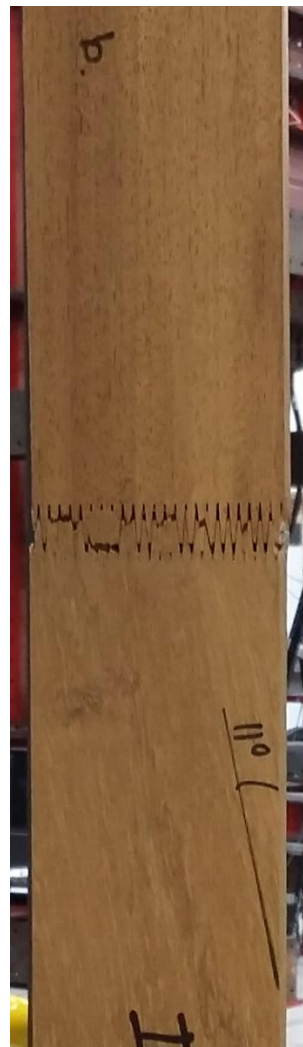
Figure 69: Failure of both fingers and glue (II-24).
