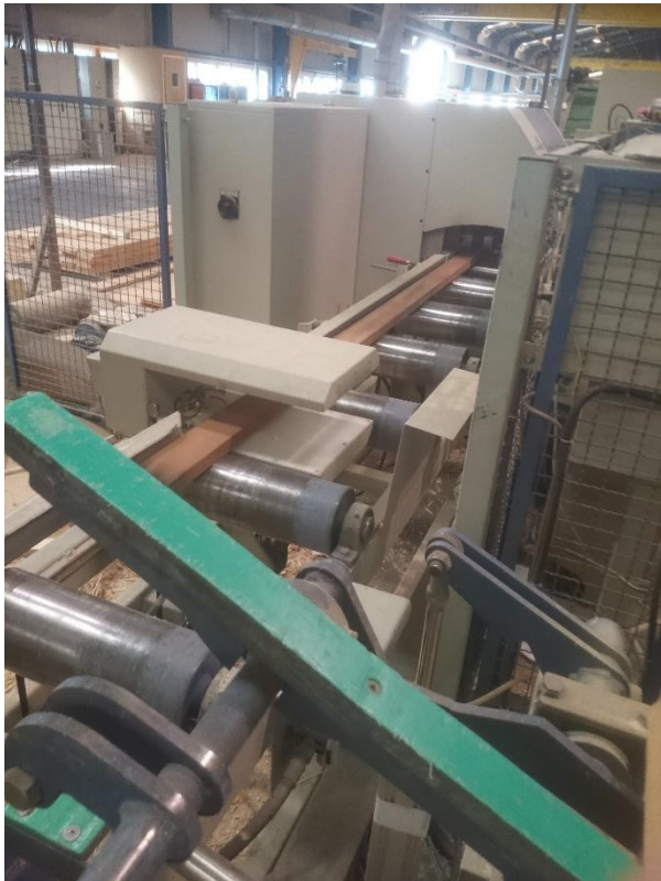
Figure 32: Automatic moisture meter, with the mitre saw in the back.
