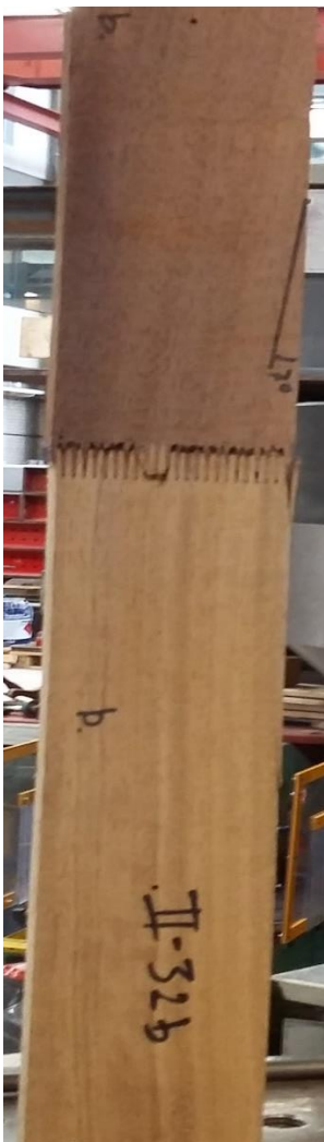
Figure 67: Finger failure (II-32).
