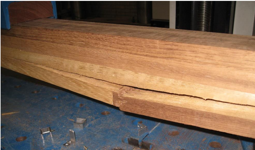
Figure 212: Failure of specimen IV-7 (crack detail).
