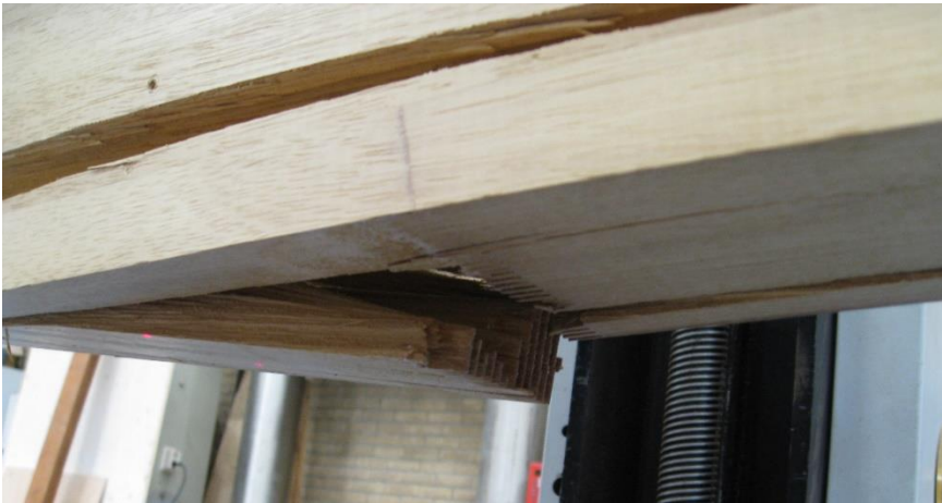
Figure 220: Failure of specimen IV-11 (crack detail).
