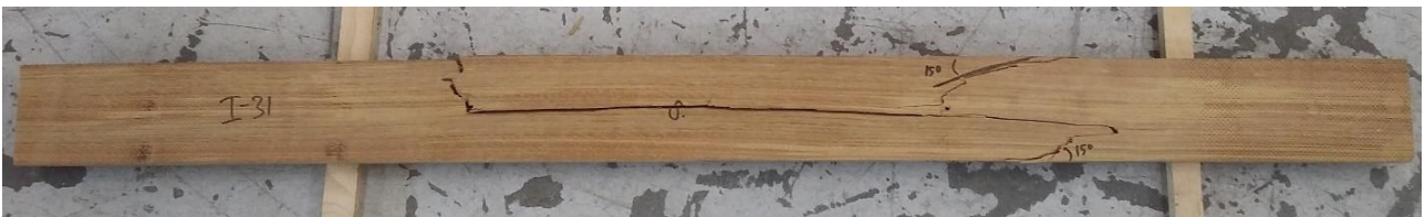
Figure 146: Failure of specimen I-31 (flipside).
