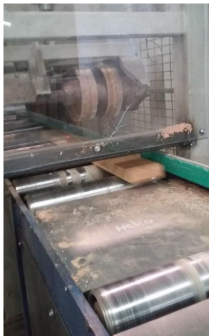
Figure 37: Planing of the boards.
