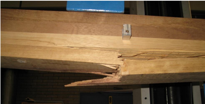
Figure 202: Failure of specimen IV-2 (crack detail).
