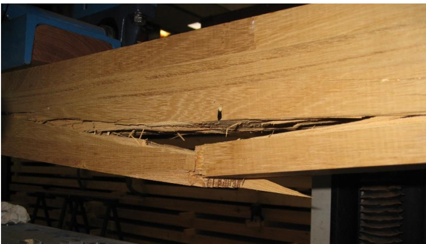
Figure 206: Failure of specimen IV-4 (crack detail).
