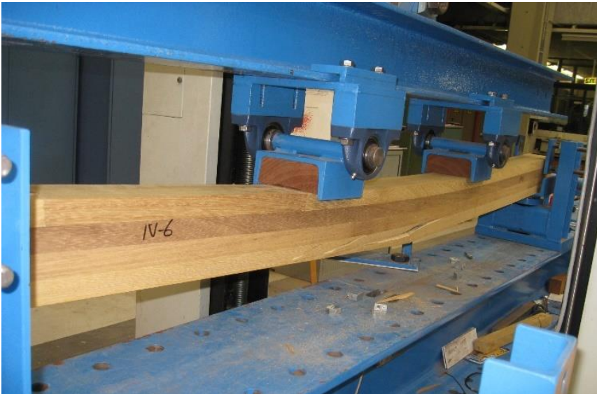
Figure 209: Failure of specimen IV-6.
