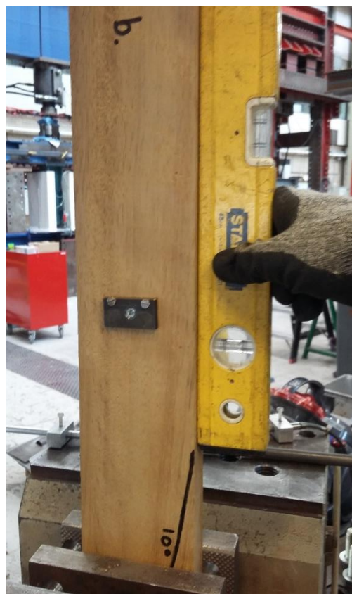
Figure 57: Levelling the lamella.
