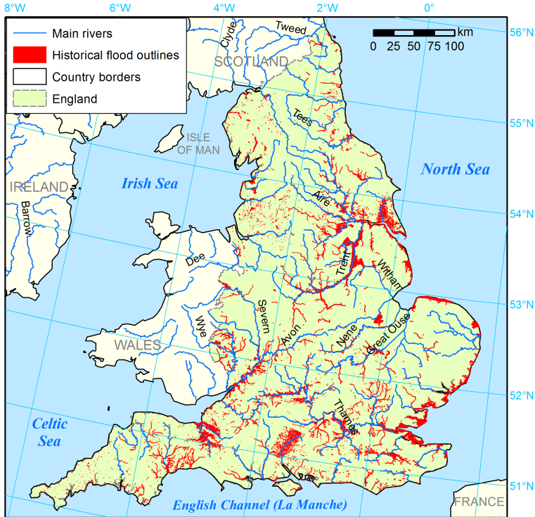
Figure 1.5: Recorded flood outlines in England, 1703–February 2017. Data from Recorded Flood Outlines, version May 2017, by the Environment Agency [54].
